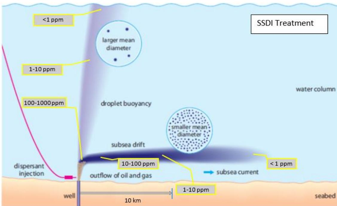
Figure 25 Cross-section of a SSDI-Treated Blowout, indicating estimated oil concentrations.
