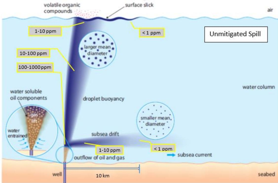
Figure 24 Cross-Section of an Unmitigated Blowout, with Estimated Oil Concentrations.
