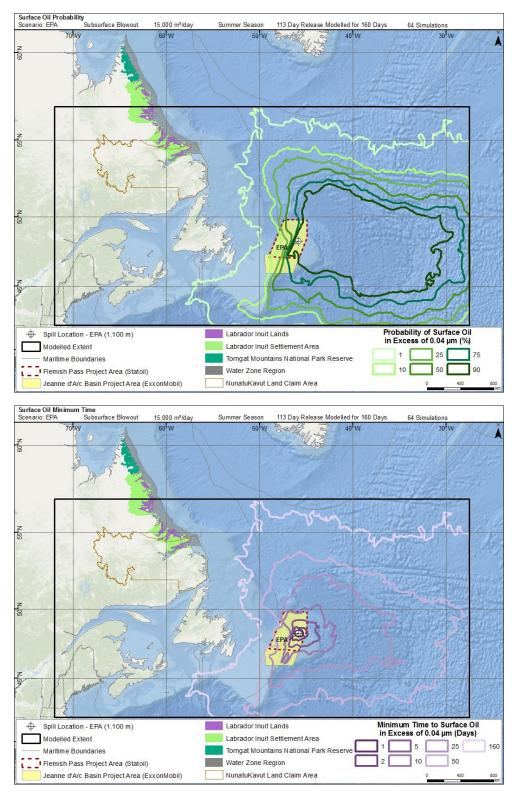
Figure 17 Summer probability of average surface oil thickness >  $0.04 \mu m$  (top) and minimum time to threshold exceedance (bottom) resulting from a subsurface blowout.
