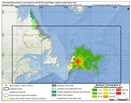
Figure 22. Maximum dissolved hydrocarbon concentration at any depth in the water column for the 95<sup>th</sup> percentile surface oil thickness case.
