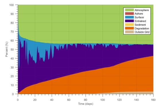
Figure 21. Mass balance plots for the 95<sup>th</sup> percentile surface oil thickness case.
