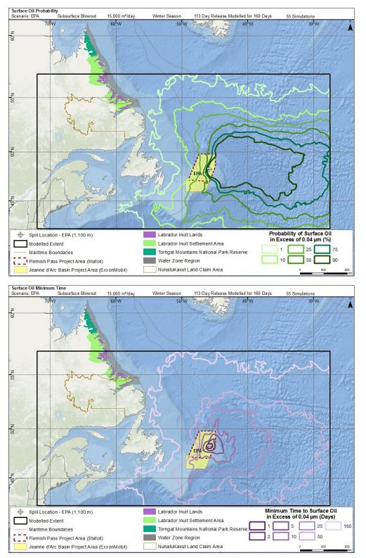
Figure 18 Winter probability of average surface oil thickness > 0.04  $\mu$ m (top) and minimum time to threshold exceedance (bottom) resulting from a subsurface blowout.
