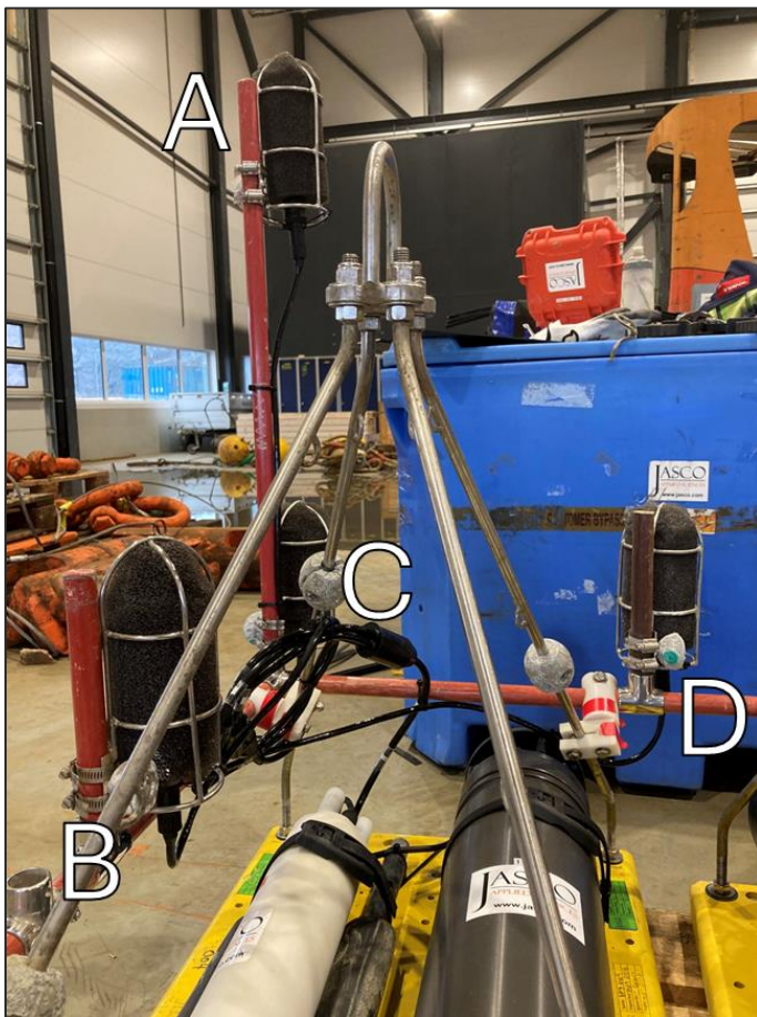
Figure 6. Photo of the tetrahedral hydrophone array set-up on a baseplate with fitted AMAR G4 (white tube) and battery pack (grey tube). Hydrophones are labelled as in Table 3.
