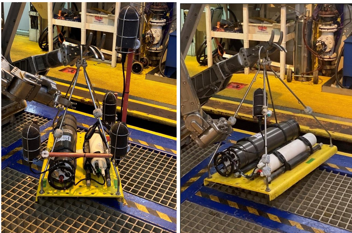
Figure 3. Baseplate moorings connected to the ROV: four-hydrophone directional array (left) and single omnidirectional hydrophone system (right).
