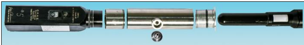
Figure 7. GRAS 42 AC Pistonphone, sleeve coupler and hydrophone
