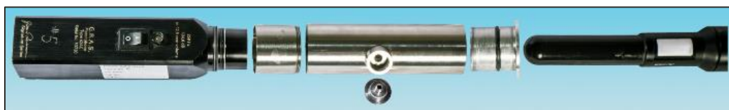
Figure 7. GRAS 42 AC Pistonphone, sleeve coupler and hydrophone
