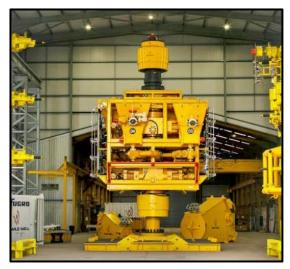
Figure 4: Capping stack
