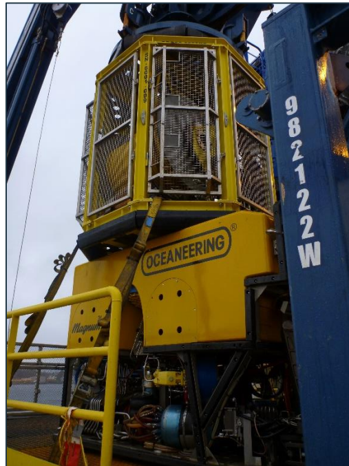
Figure 2-2 Oceaneering Magnum ROV used for the Flemish Pass benthic survey in its cradle
