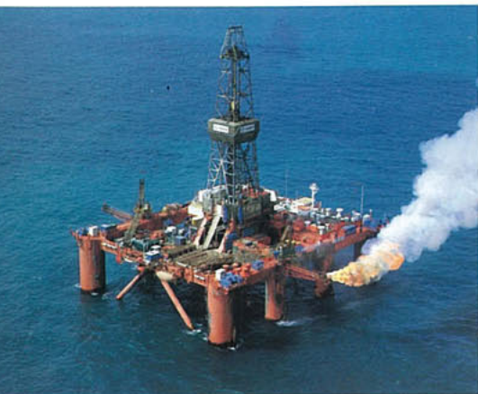
Deepsea Saga testing an exploration well on block 34/10.
