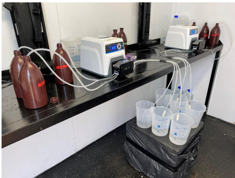
Figure 4. Simultaneous filtration of collected water samples inside the on-deck container using peristaltic pumps powered from electricity to the container. Triplicate 1L-water samples (brown bottles) from each sampling depth (50 m on the left, 10 m on the right) were filtered through 0.45 \mu\text{m} Sterivex filters using four-channel pump heads set to 300 rpm (flow rate approx. 100 mL \text{min}^{-1} ). Filter outflow was collected in 2L-beakers, and outflow volume was measured and recorded.
