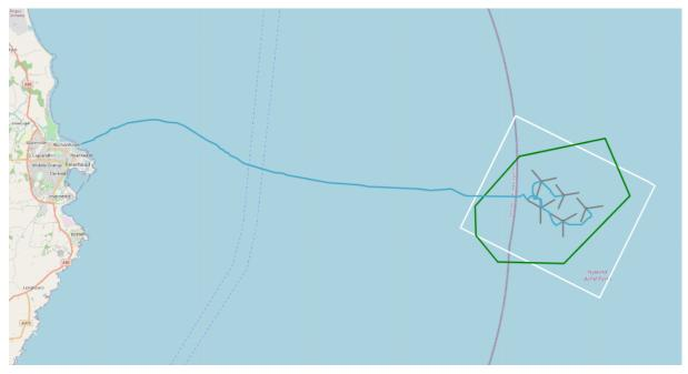
Figure 5 Hywind Scotland offshore wind park, with 5 turbines (anchor lines in grey, connecting cables in blue) outside of Peterhead (UK). The area of operation (about 8x4 km, white rectangle) and a restricted area of low marine traffic (green polygon) surround the installations.
