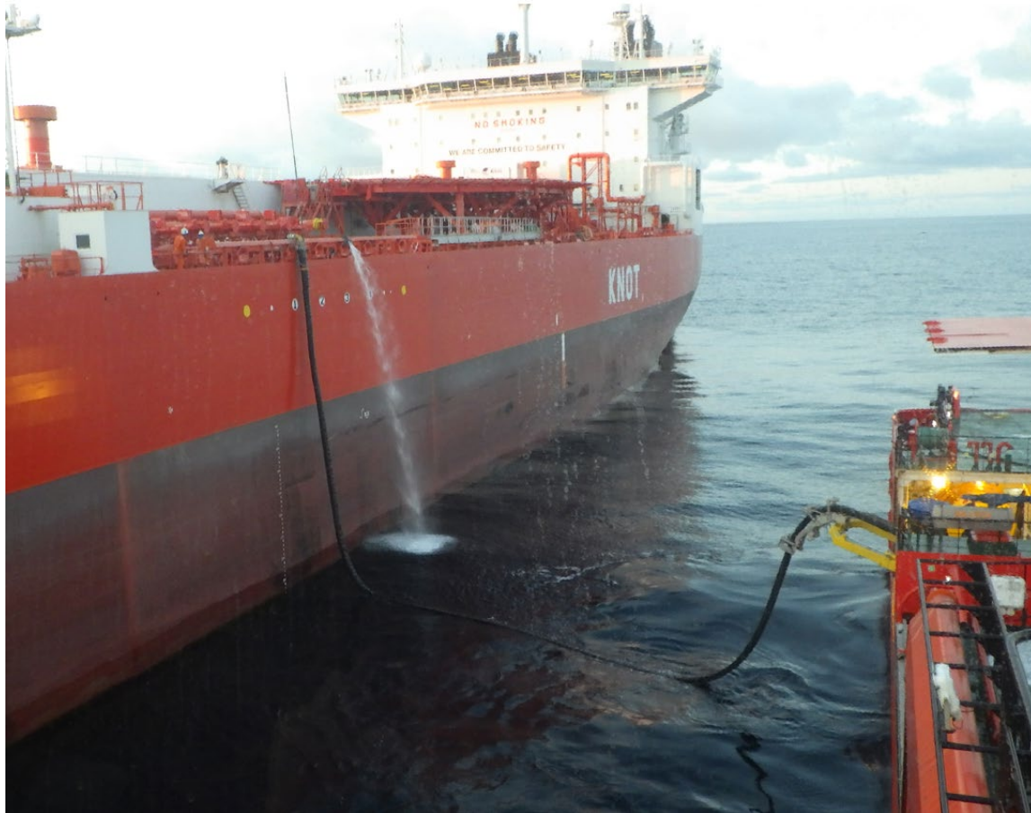
STS transfer of oil emulsion. Ref. NOFO Guide for transfer operations between OR vessels and tankers (2019)
