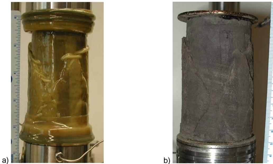
Figure 84. ST4 test specimen a) post-test specimen still inside membrane b) post-test specimen with membrane removed showing deformed state of specimen
