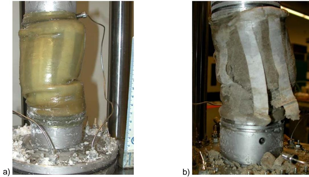
Figure 48. NTX3 test specimen a) post-test specimen still inside membrane b) frozen post-test specimen frozen and membrane removed showing highly deformed state of specimen
