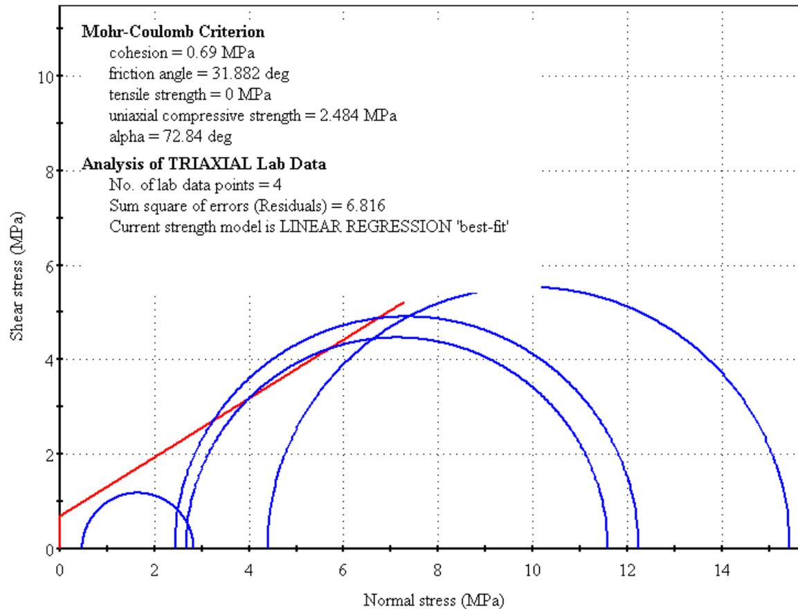
**Figure 4.5: Mohr-Coulomb failure envelope fit to peak triaxial test results on McMurray Formation oil sands samples from Paramount Leismer 09-28-78-10W4M (depth range: 420.9 mKB to 427.3 mKB). Data from U of A (2005)**
