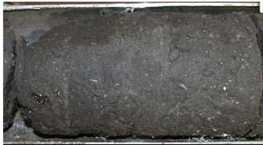
Figure 15. Interbedded mudstone/oil sands Sample SC3 (from Paramount Leismer 09-28-78-10W4M)
