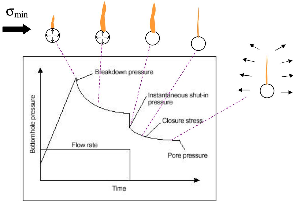
**Figure A.1:** A schematic showing a typical pressure-time history recorded during a hydraulic fracturing stress test and its corresponding fracturing events. The pressure-time plot is from Thiecrlin and Rogiers (2000).
