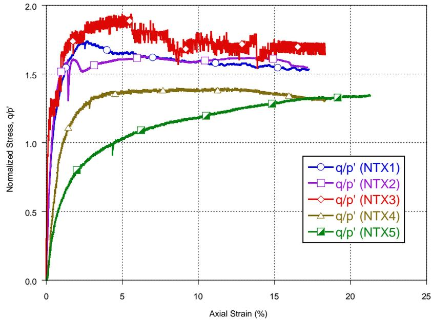
Figure 65. Normalized stress strain curves illustrating the variation in behavior between specimens.
