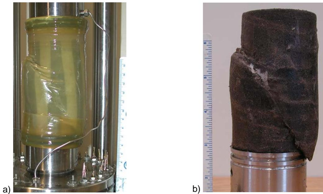
Figure 42. NTX2 test specimen a) post-test specimen still inside membrane b) frozen post-test specimen frozen and membrane removed showing highly deformed state of specimen
