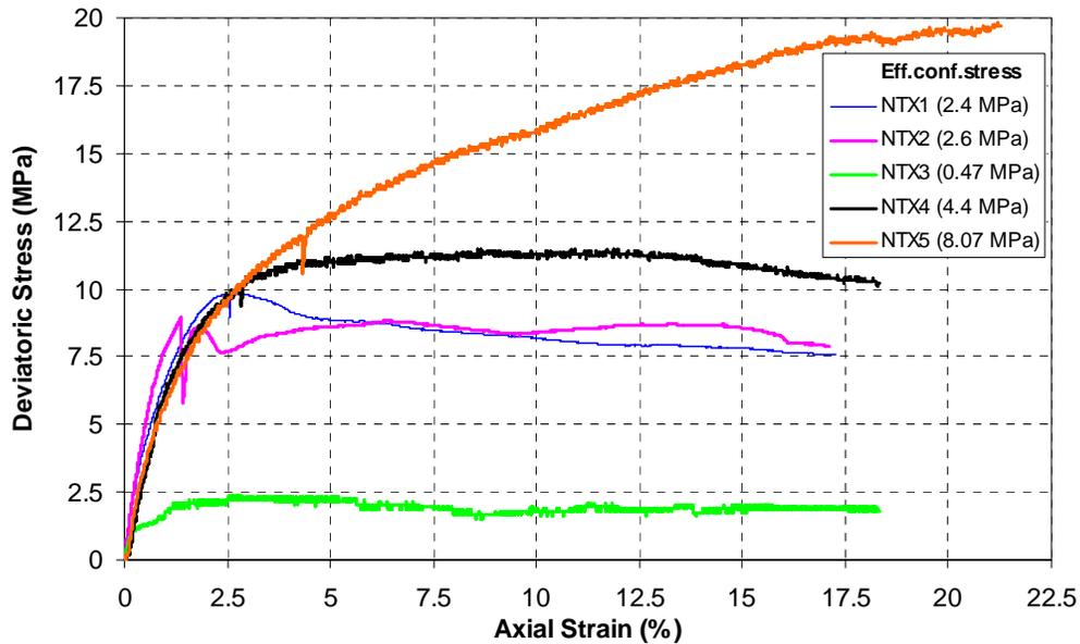
Figure 4.9: Stress-strain behaviour of McMurray Formation oil sands samples from Paramount Leismer 09-28-78-10W4M (depth range: 420.9 mKB to 427.3 mKB) during undrained triaxial tests. Data from U of A (2005).
