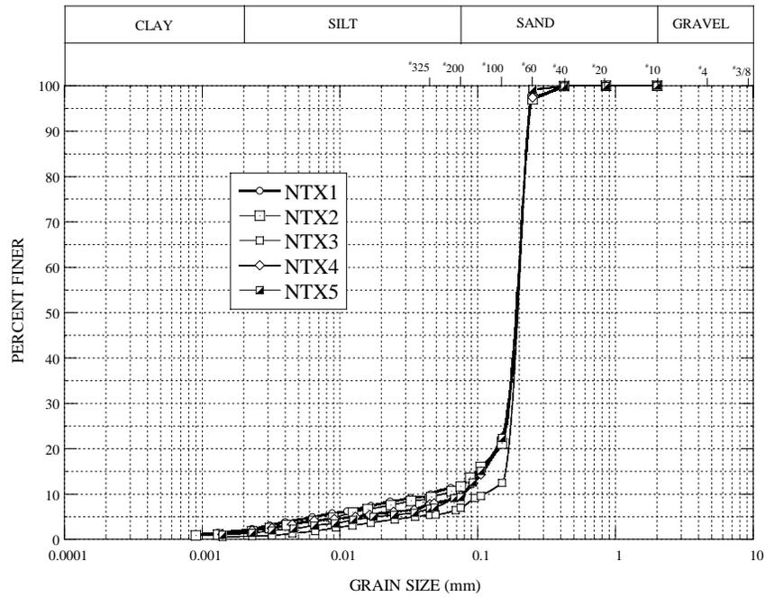
Figure 31. Particle size distributions for oil sands specimens
