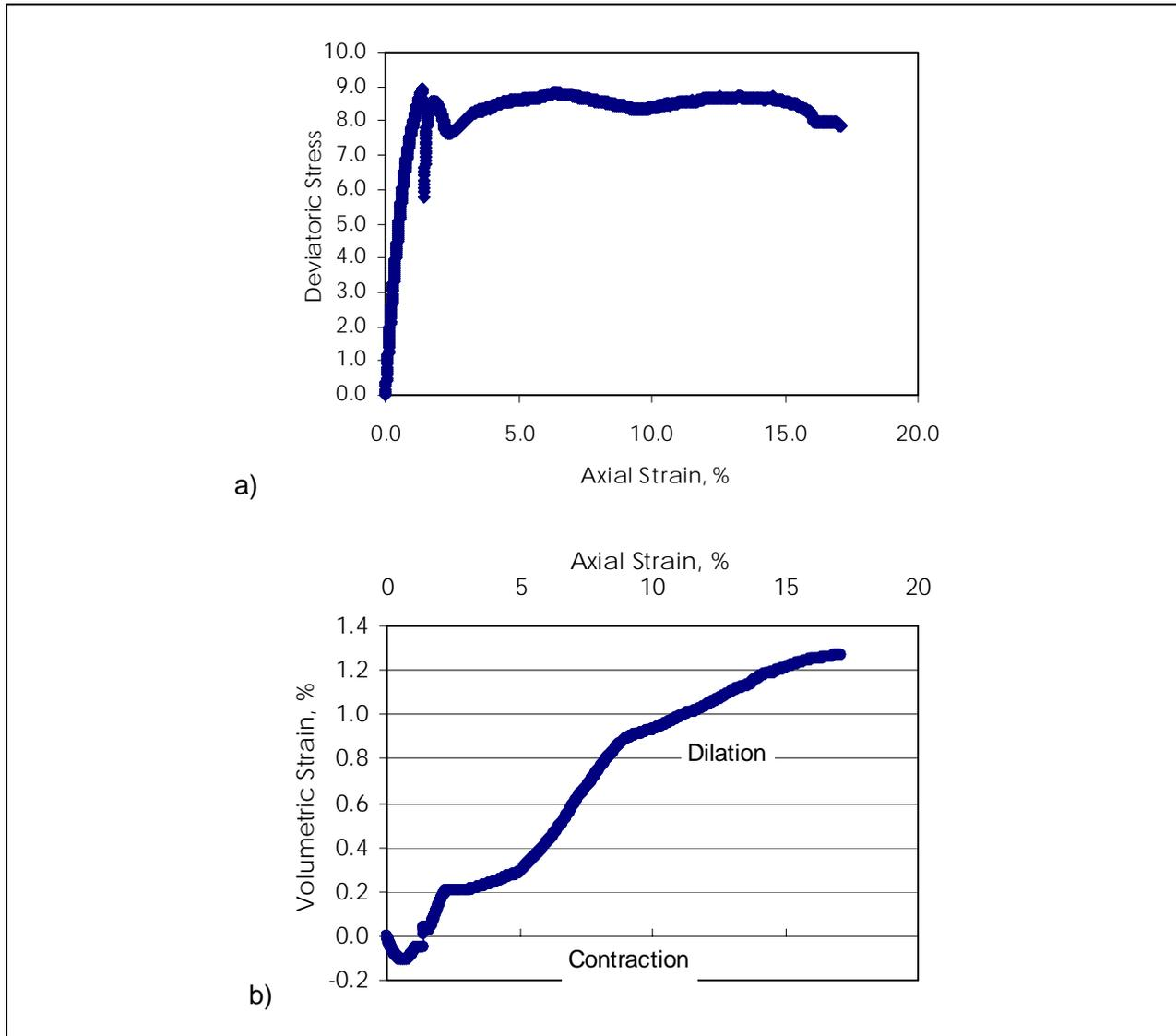
Figure 44. NTX2 triaxial test results a) stress-strain b) volume change
