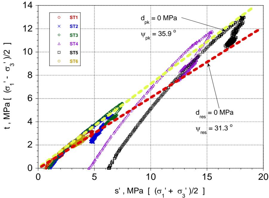
Figure 100. Stress path plot (s'-t) for shale specimen CU test results.
