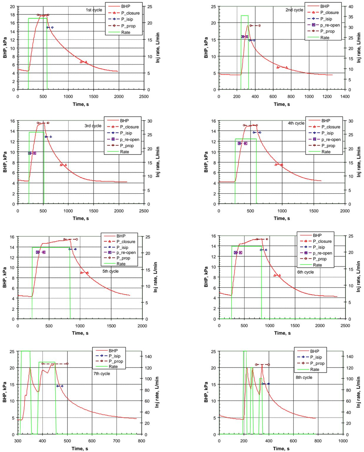
**Figure A.8:** Characteristic pressures determined from the various injection/shut-in cycles in testing the oil sands facie (420 mTVD) at well 4-27.
