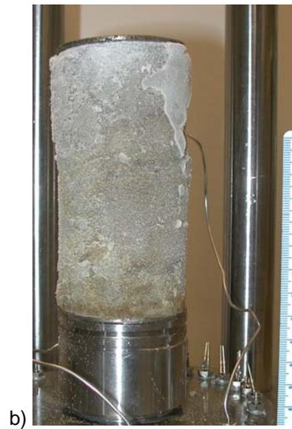
Figure 53. NTX4 test specimen a) frozen extracted specimen b) frozen bitumen free specimen installed in triaxial cell
