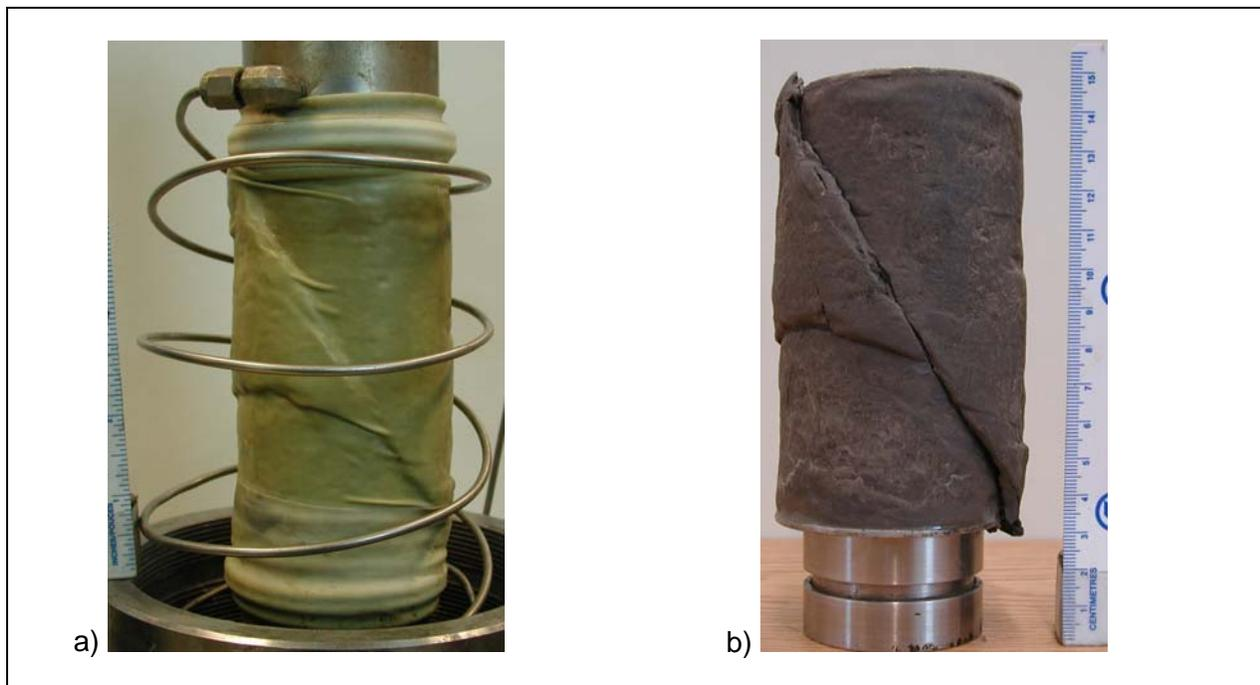
Figure 69. ST1 test specimen a) post-test specimen still inside membrane b) post-test specimen with membrane removed showing deformed state of specimen
