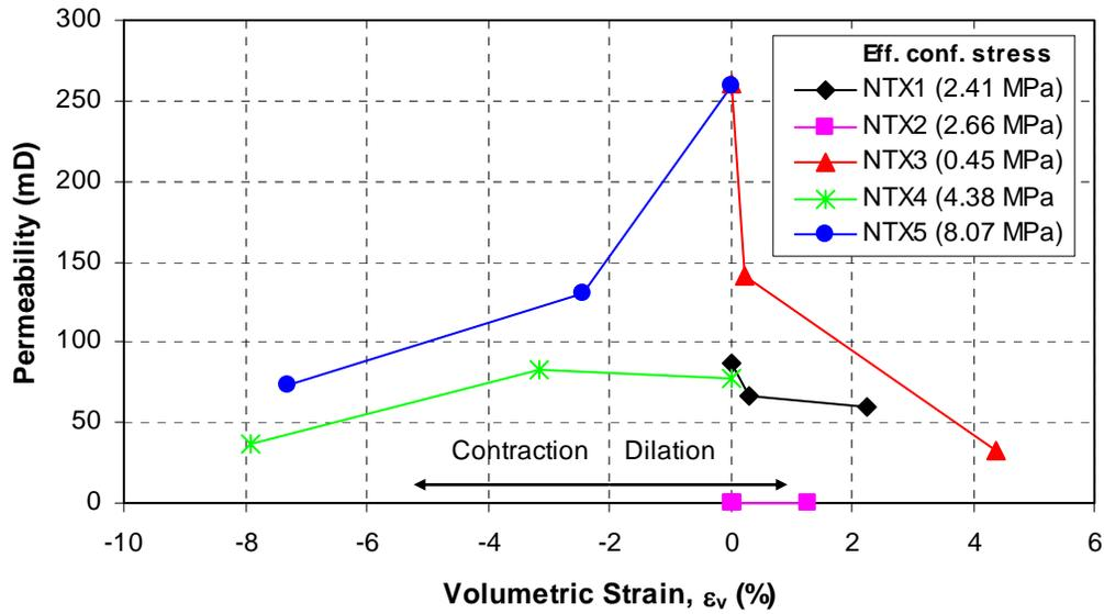
**Figure 4.11: Change of permeability ( $k$ ) as a function of volumetric strain ( $\epsilon_v$ ) in McMurray Formation oil sands samples measured before shearing, at peak and at post-peak condition in drained triaxial tests. Data from U of A (2005).**
