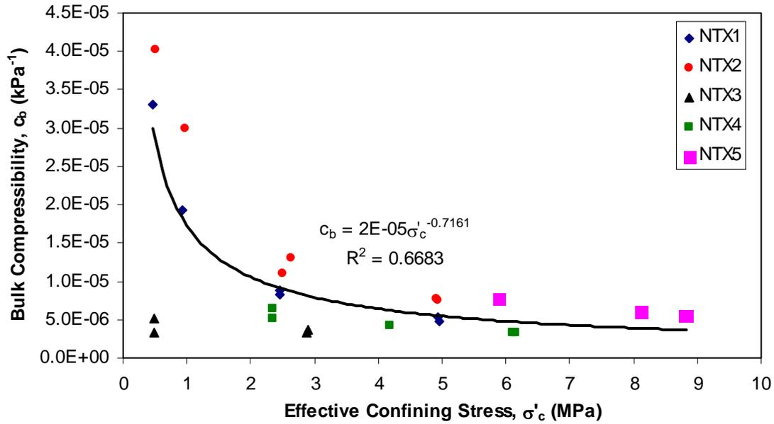
Figure 4.1: Bulk compressibility of oil sands samples as a function of effective confining stress during isotropic loading unloading tests.
