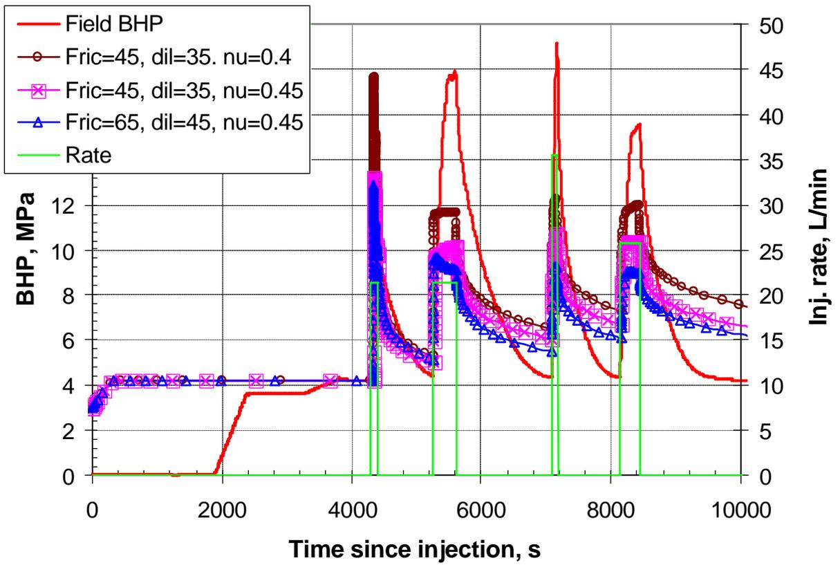
**Figure 12:** Effect of varying Poisson's ratio, friction and dilation angles in matching the field data.
