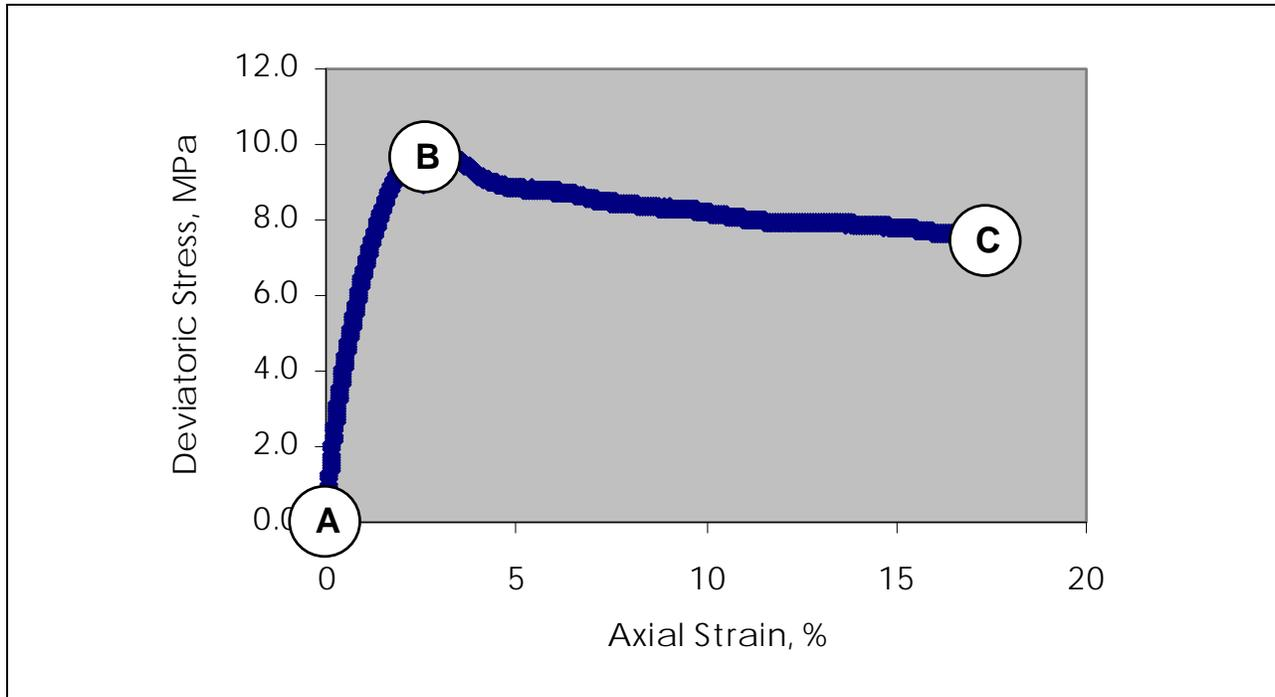
Figure 40. Locations in stress-strain curve where permeability measurements were taken on specimen NTX1
