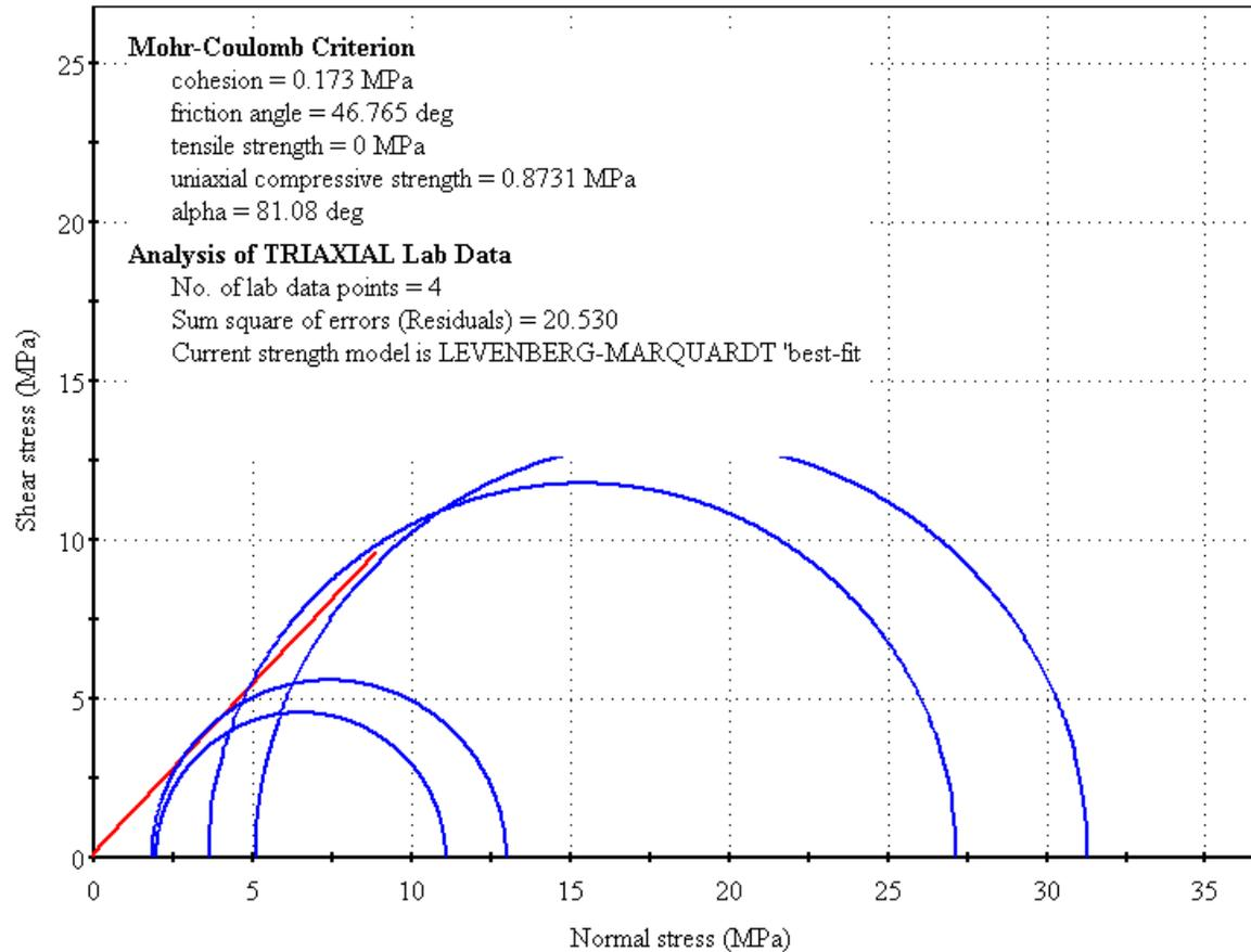
**Figure 4.3: Mohr-Coulomb failure envelope fit to peak triaxial test results on McMurray Formation mudstone samples from Paramount Leismer 09-28-78-10W4M (depth range: 394.56 mKB to 397.75 mKB). Data from U of A (2005)**
