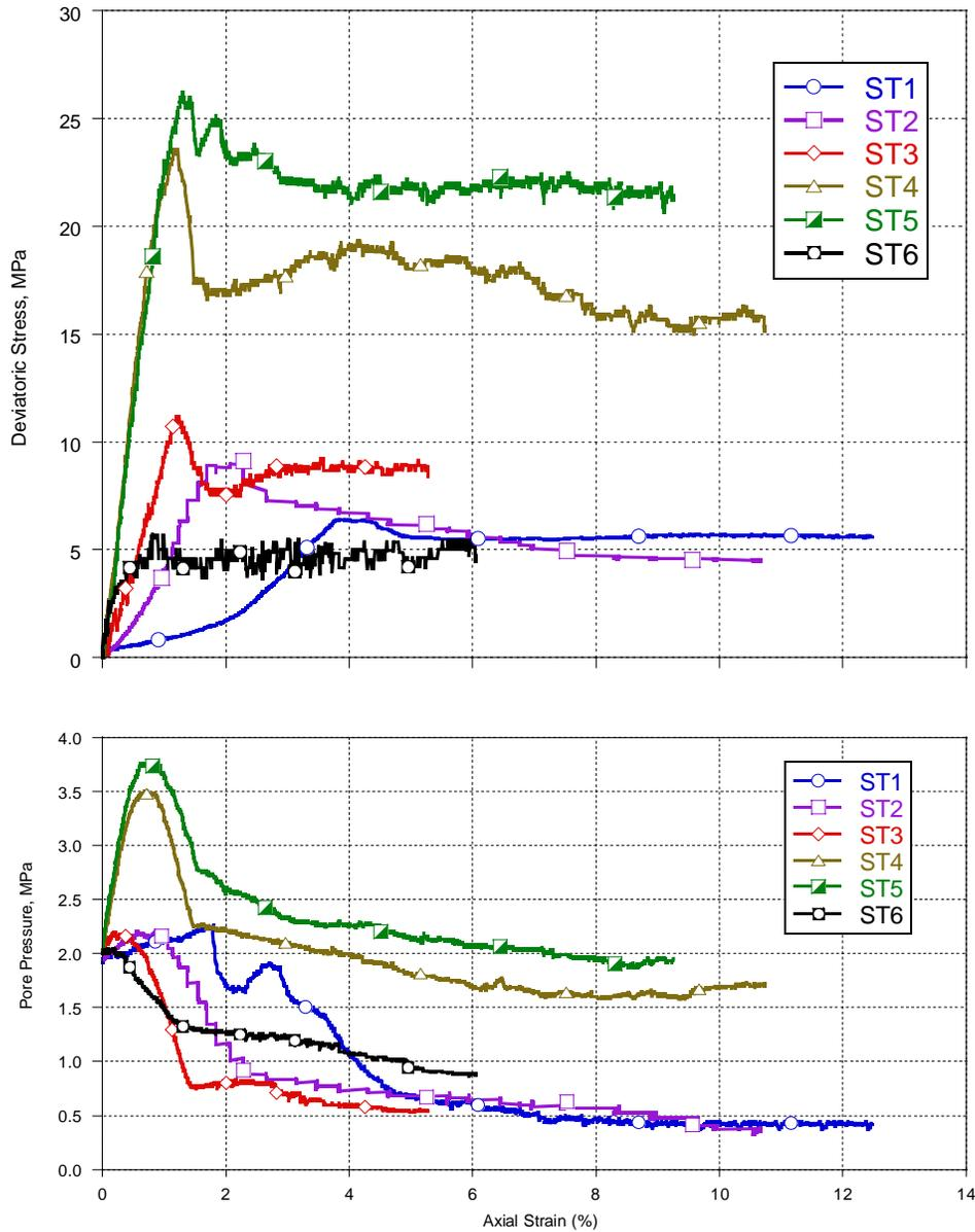
Figure 98. Summary of all shale triaxial test results
