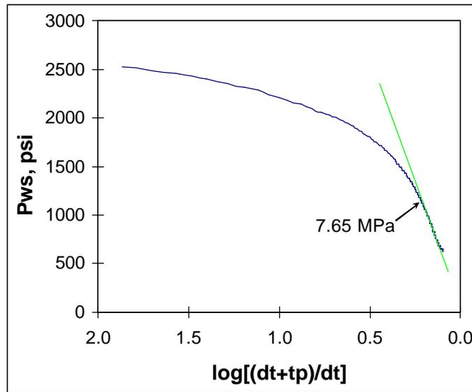
Figure A.6: An example Horner plot to determine the fracture closure pressure.
