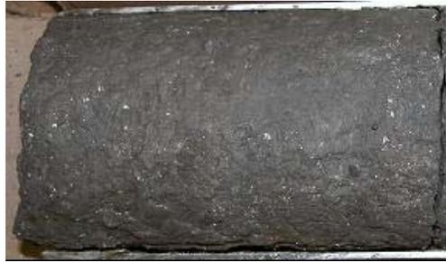
Figure 17. Interbedded mudstone/oil sands Sample SC5 (from Paramount Leismer 09-28-78-10W4M)
