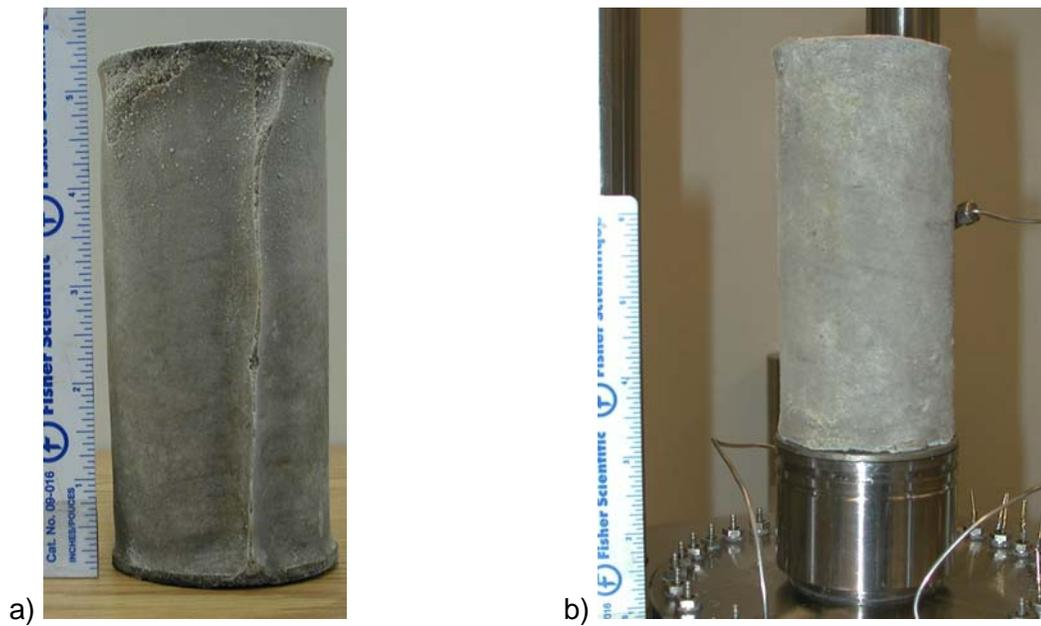
Figure 36. NTX1 test specimen a) frozen extracted specimen b) frozen bitumen free specimen installed in triaxial cell
