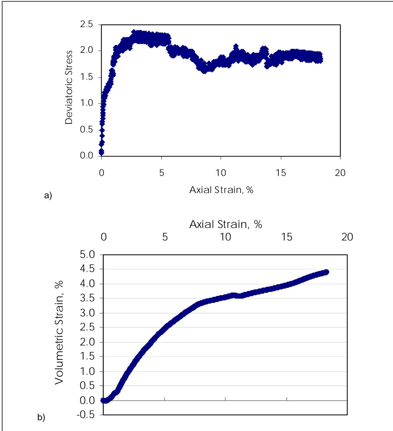
Figure 50. NTX3 triaxial test results a) stress-strain b) volume change
