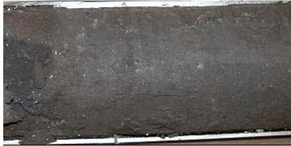
Figure 29. Interbedded mudstone/oil sands Sample SC17 (from Paramount Leismer 03-03-79-10W4M)
