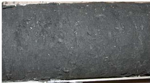
Figure 22. Interbedded mudstone/oil sands Sample SC10 (from Paramount Leismer 03-03-79-10W4M)
