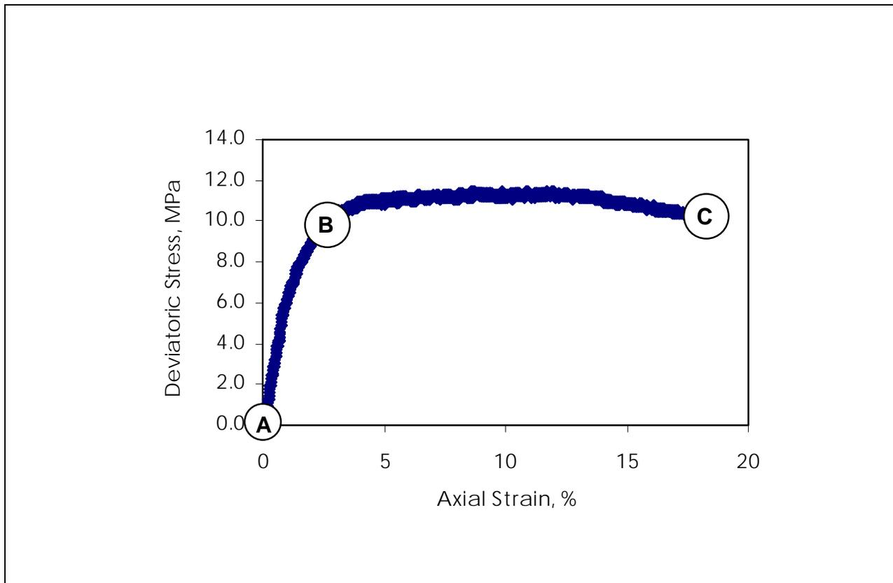
Figure 57. Locations in stress-strain curve where permeability measurements were taken on specimen NTX4
