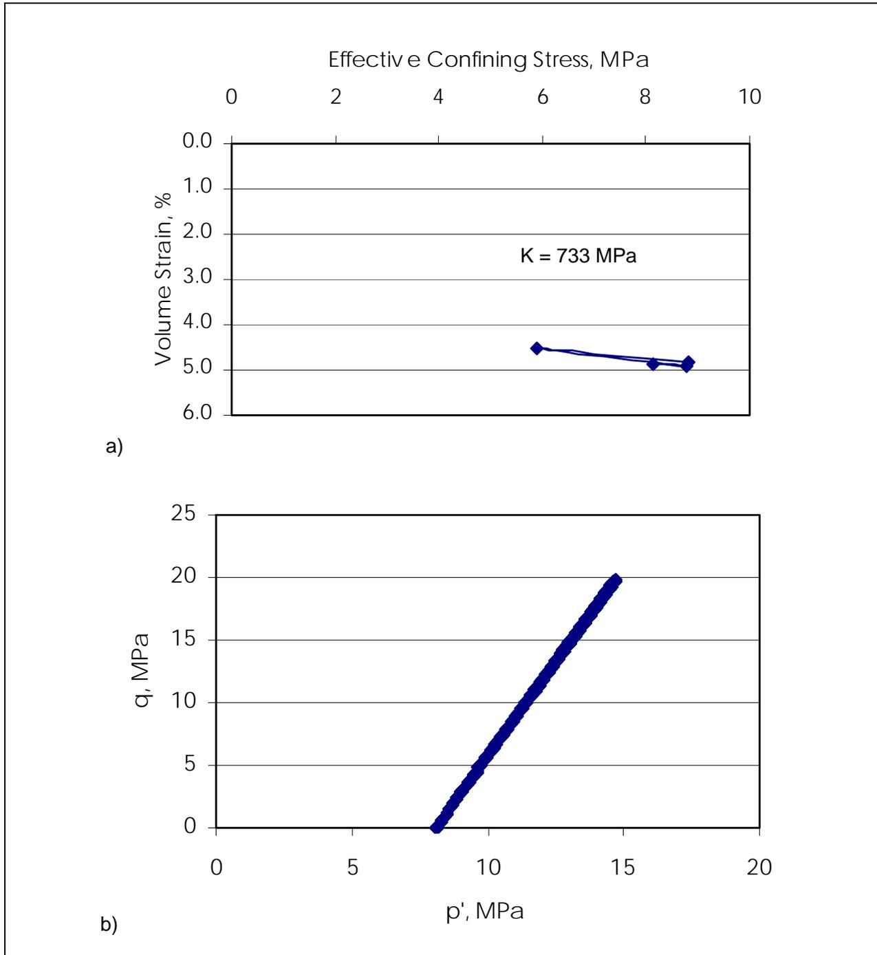
Figure 61. NTX5 triaxial test results a) compressibility b) stress path
