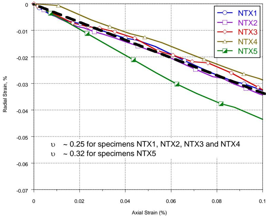
Figure 67. Poisson ratio calculation for oil sands specimens
