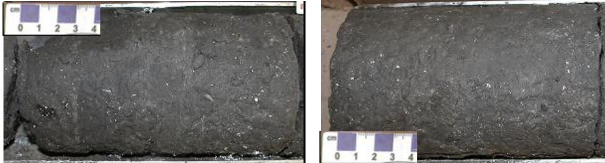
**Figure 3.1: Unfrozen mudstone core samples (SC # 3 and SC # 5) prior to core plug drilling for geomechanical testing. Paramount Leismer 09-28-78-10W4M.**
