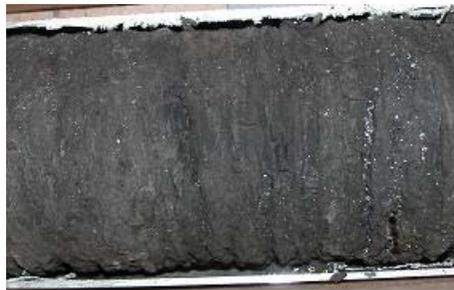
Figure 19. Interbedded mudstone/oil sands Sample SC7 (from Paramount Leismer 03-03-79-10W4M)
