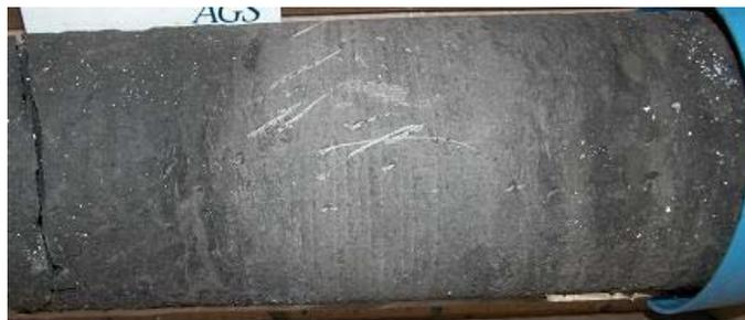
Figure 24. Interbedded mudstone/oil sands Sample SC12 (from Paramount Leismer 03-03-79-10W4M)
