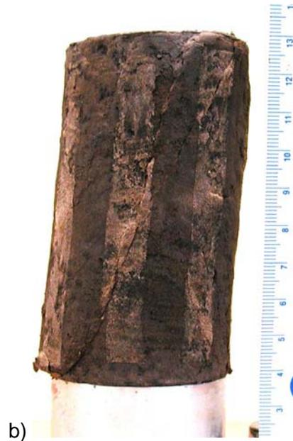
Figure 89. ST5 test specimen a) post-test specimen still inside membrane b) post-test specimen with membrane removed showing deformed state of specimen (contrast enhanced in photo)
