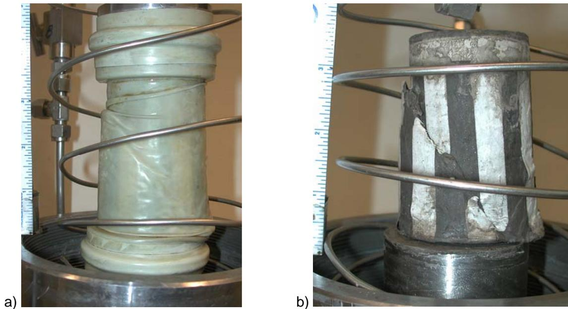
Figure 74. ST2 test specimen a) post-test specimen still inside membrane b) post-test specimen with membrane removed showing deformed state of specimen
