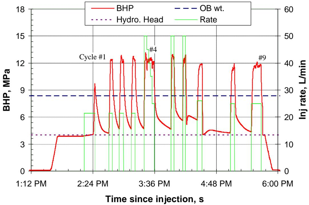
**Figure 5:** Recorded pressure history during the injection test in the shaly facie at 399 mTVD at well 14-27.
