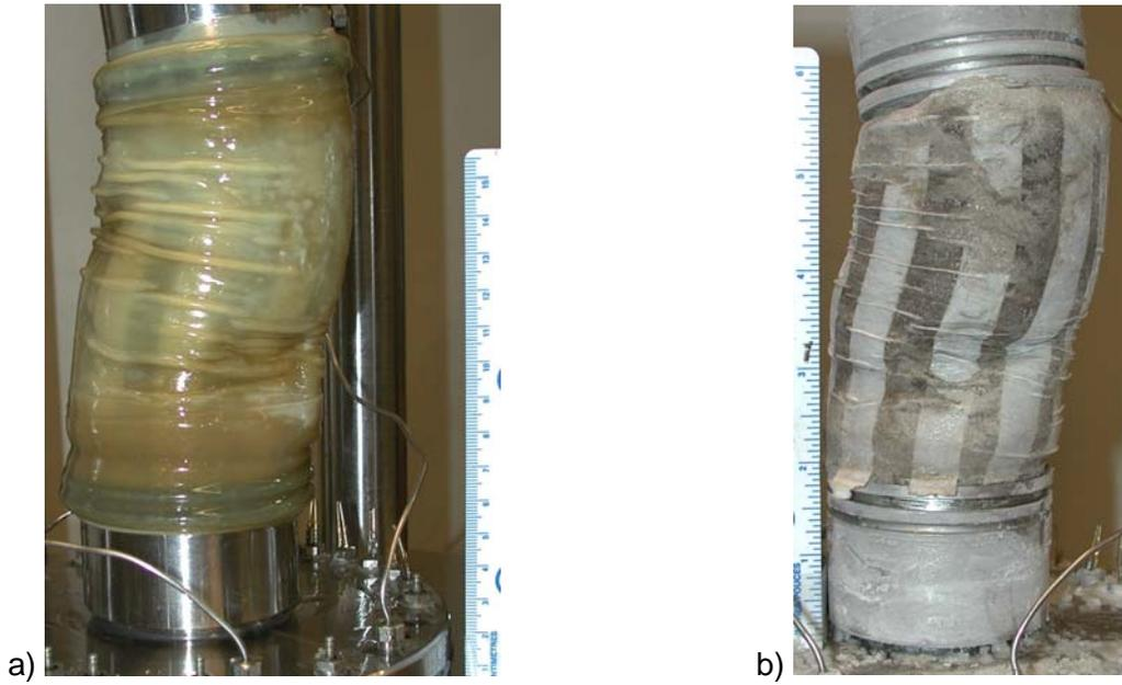
Figure 60. NTX5 test specimen a) post-test specimen still inside membrane b) frozen post-test specimen frozen and membrane removed showing highly deformed state of specimen
