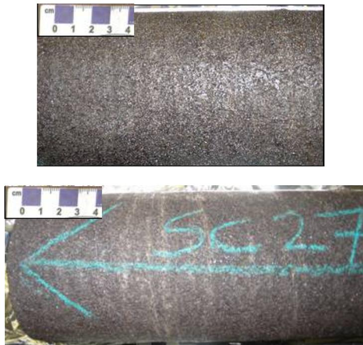
**Figure 3.2: Frozen oil sands core samples (SC # 21 and SC # 27) prior to core plug drilling for geomechanical testing. Paramount Leismer 09-28-78-10W4M.**
