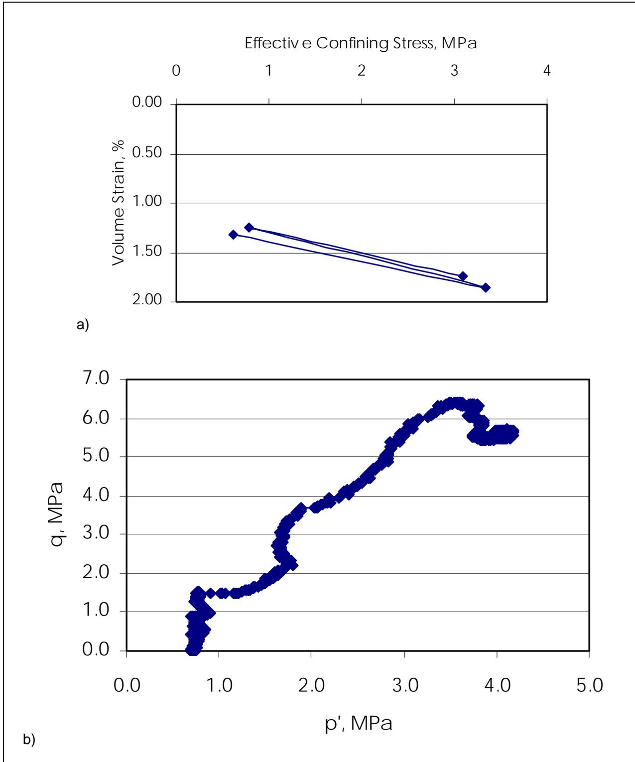
Figure 70. ST1 triaxial test results a) compressibility b) stress path
