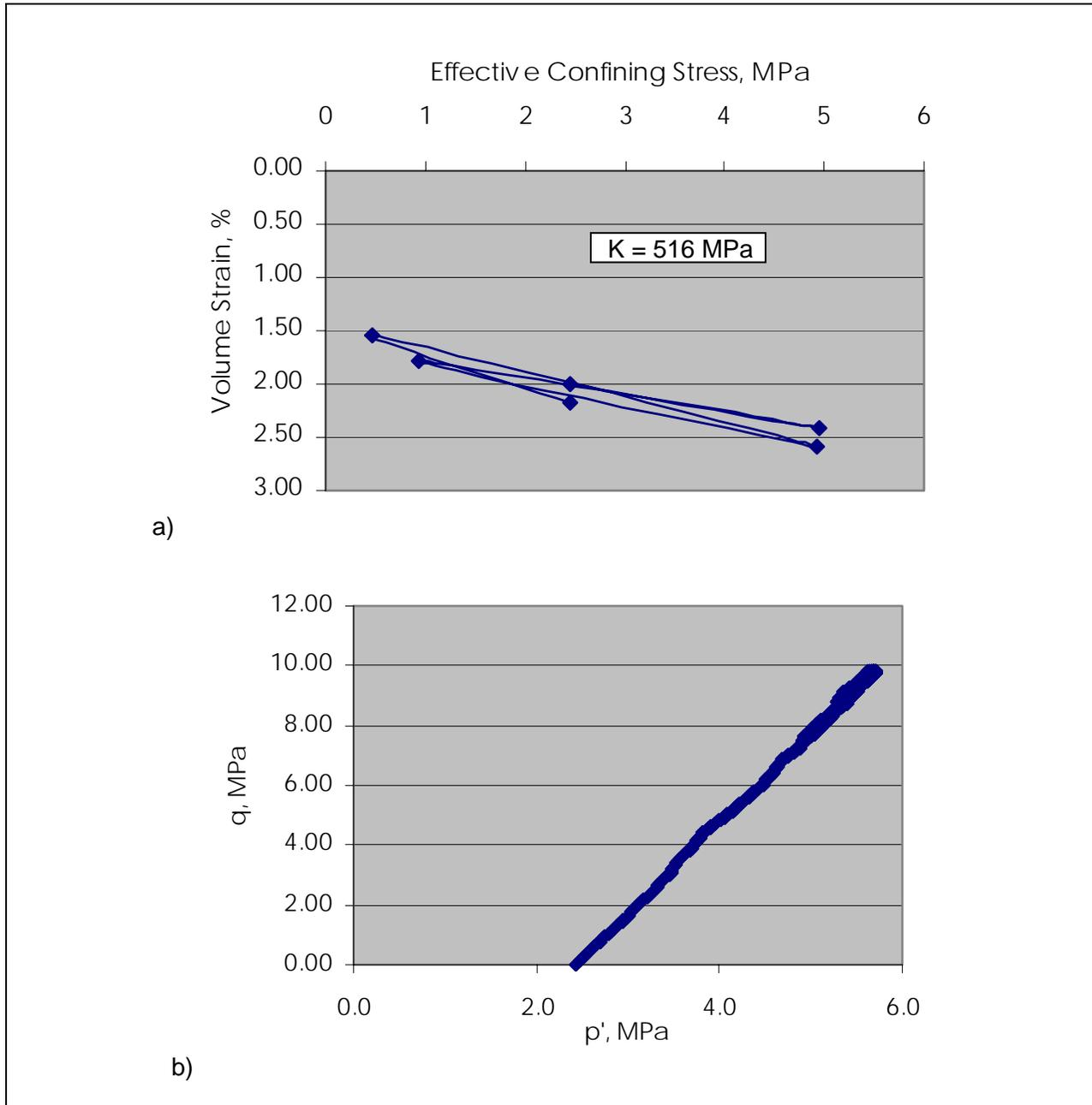
Figure 38. NTX1 triaxial test results a) compressibility b) stress path
