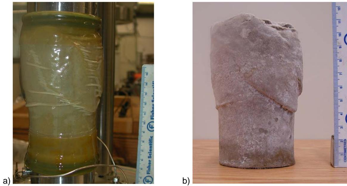
Figure 37. NTX1 test specimen a) post-test specimen still inside membrane b) frozen post-test specimen frozen and membrane removed showing highly deformed state of specimen
