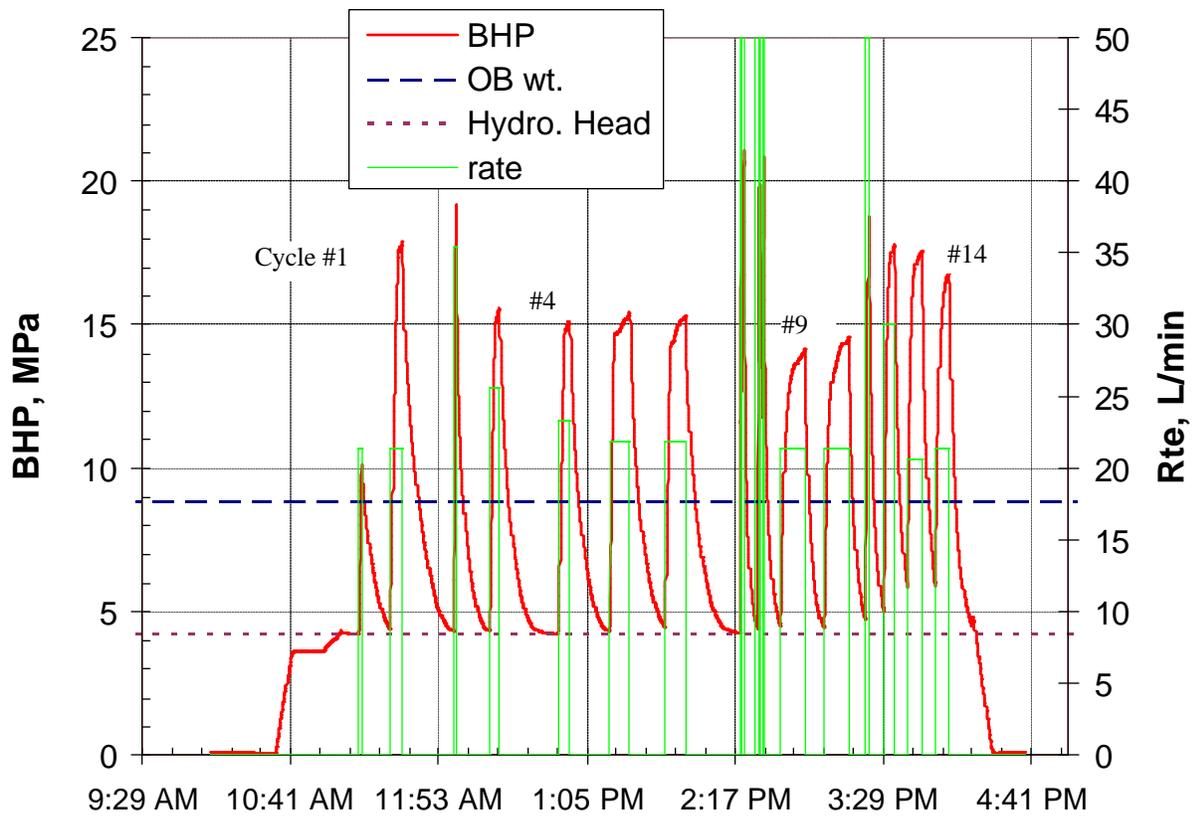
**Figure 2:** Recorded pressure history during the injection test in the oil sands facie at 420 mTVD at well 4-27. The bottomhole pressures (“BHP”) were recorded via two downhole pressure sensors. The hydraulic head (“Hydro. head”) was the water column weight. The overburden weight (“OB weight”) was calculated from the density log. Similar conventions are used below unless otherwise notified.
