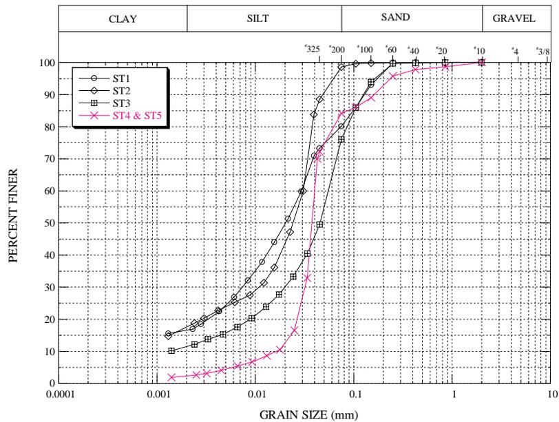
Figure 32. Particle size distributions for shale specimens
