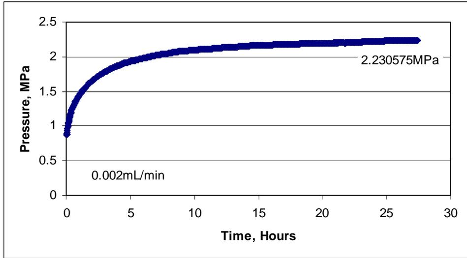
Figure 97. ST6 permeability test results
