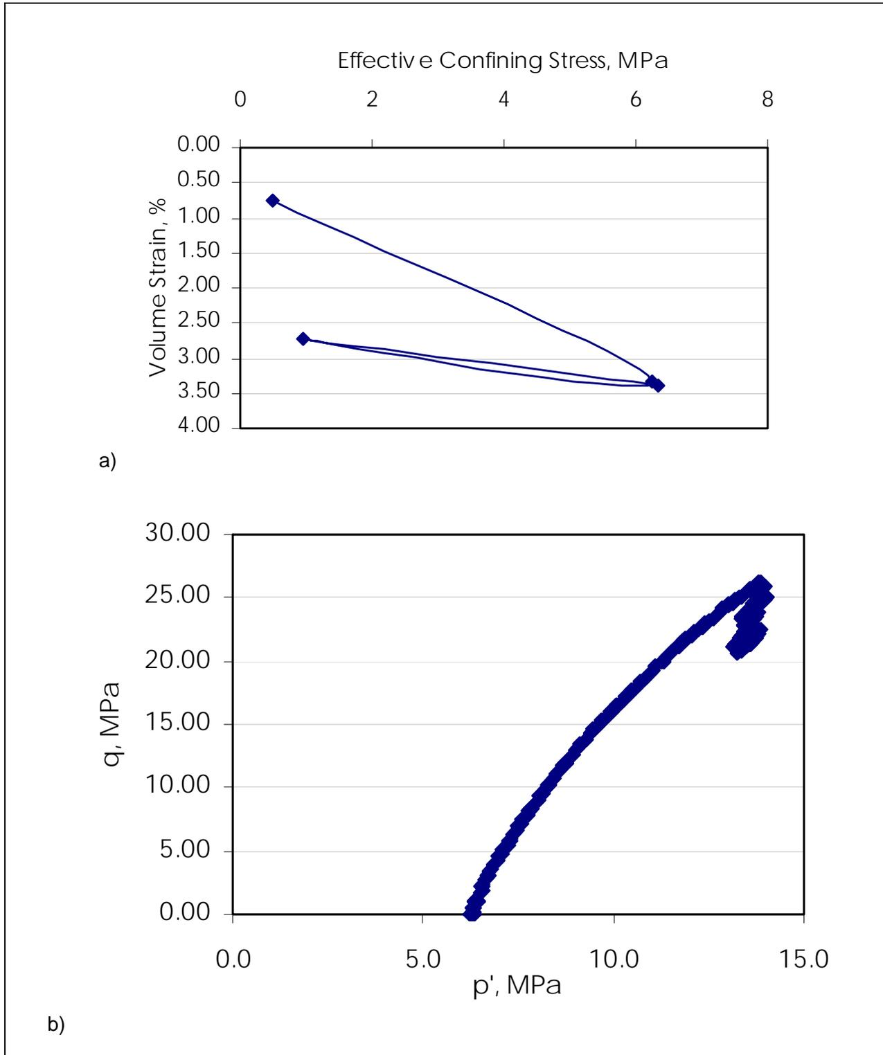
Figure 90. ST5 triaxial test results a) compressibility b) stress path
