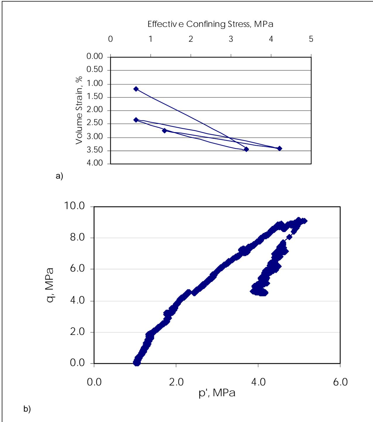
Figure 75. ST2 triaxial test results a) compressibility b) stress path
