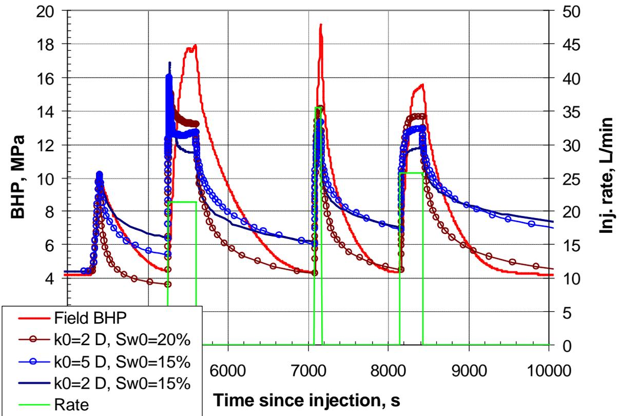
**Figure 13:** Effect of formation permeability ( $k_0$ ) and initial water saturation ( $Sw_0$ ) on the history-matching.
