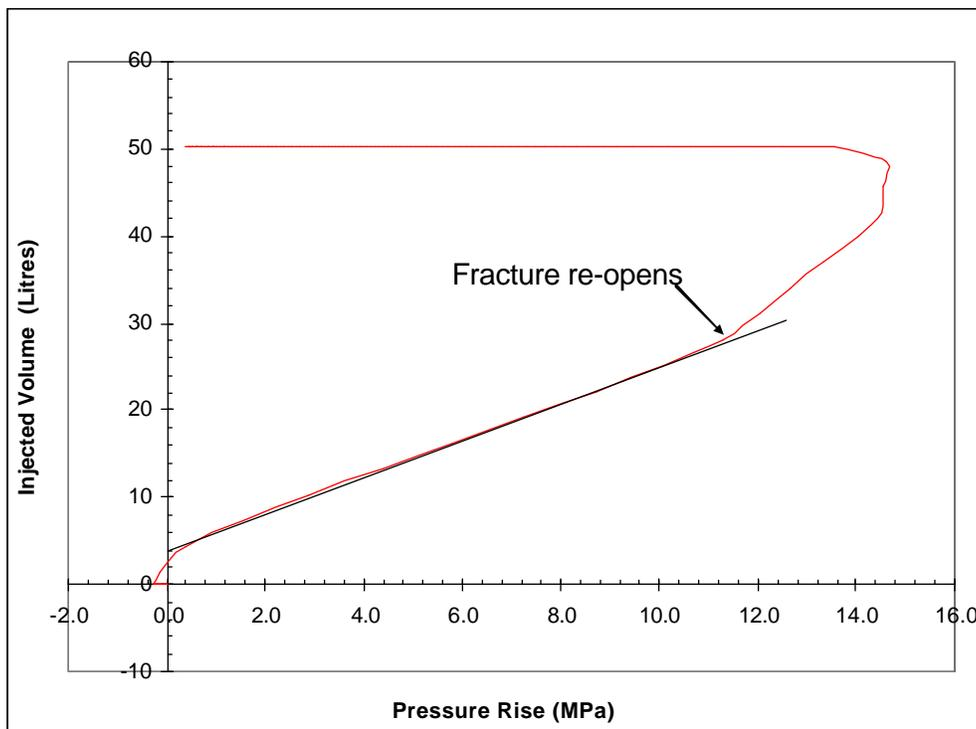
Figure A.7: An example Cartesian plot for pressure rise during the injection vs. cumulative injected volume to determine the fracture re-opening pressure.
