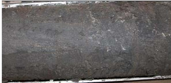
Figure 30. Interbedded mudstone/oil sands Sample SC18 (from Paramount Leismer 03-03-79-10W4M)
