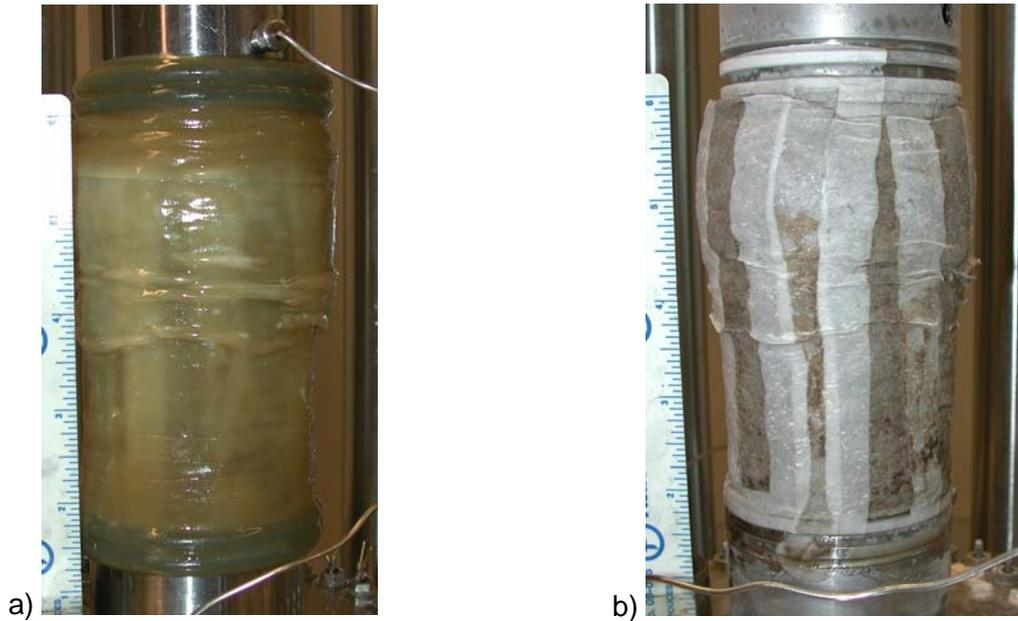
Figure 54. NTX4 test specimen a) post-test specimen still inside membrane b) frozen post-test specimen frozen and membrane removed showing highly deformed state of specimen
