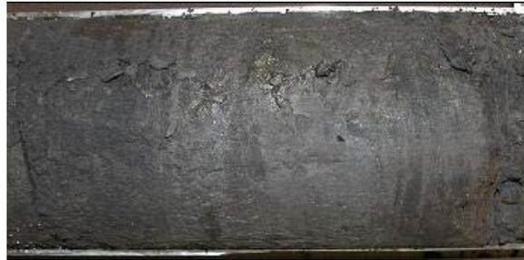
Figure 14. Interbedded mudstone/oil sands Sample SC2 (from Paramount Leismer 09-28-78-10W4M)
