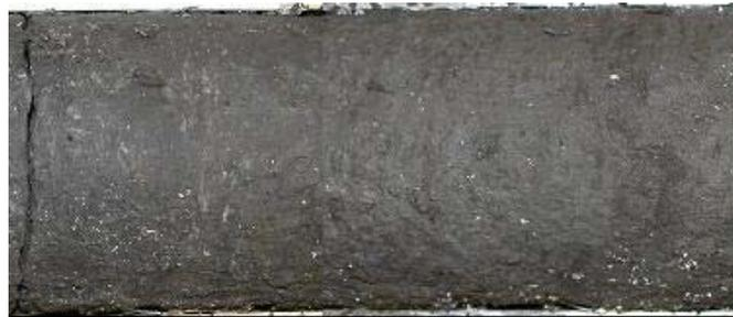
Figure 18. Interbedded mudstone/oil sands Sample SC6 (from Paramount Leismer 09-28-78-10W4M)
