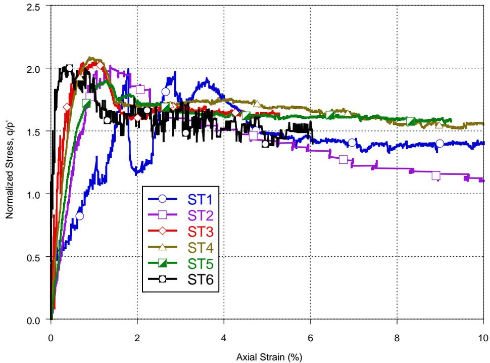
Figure 99. Normalized stress strain curves illustrating the variation in behavior between shale specimens.
