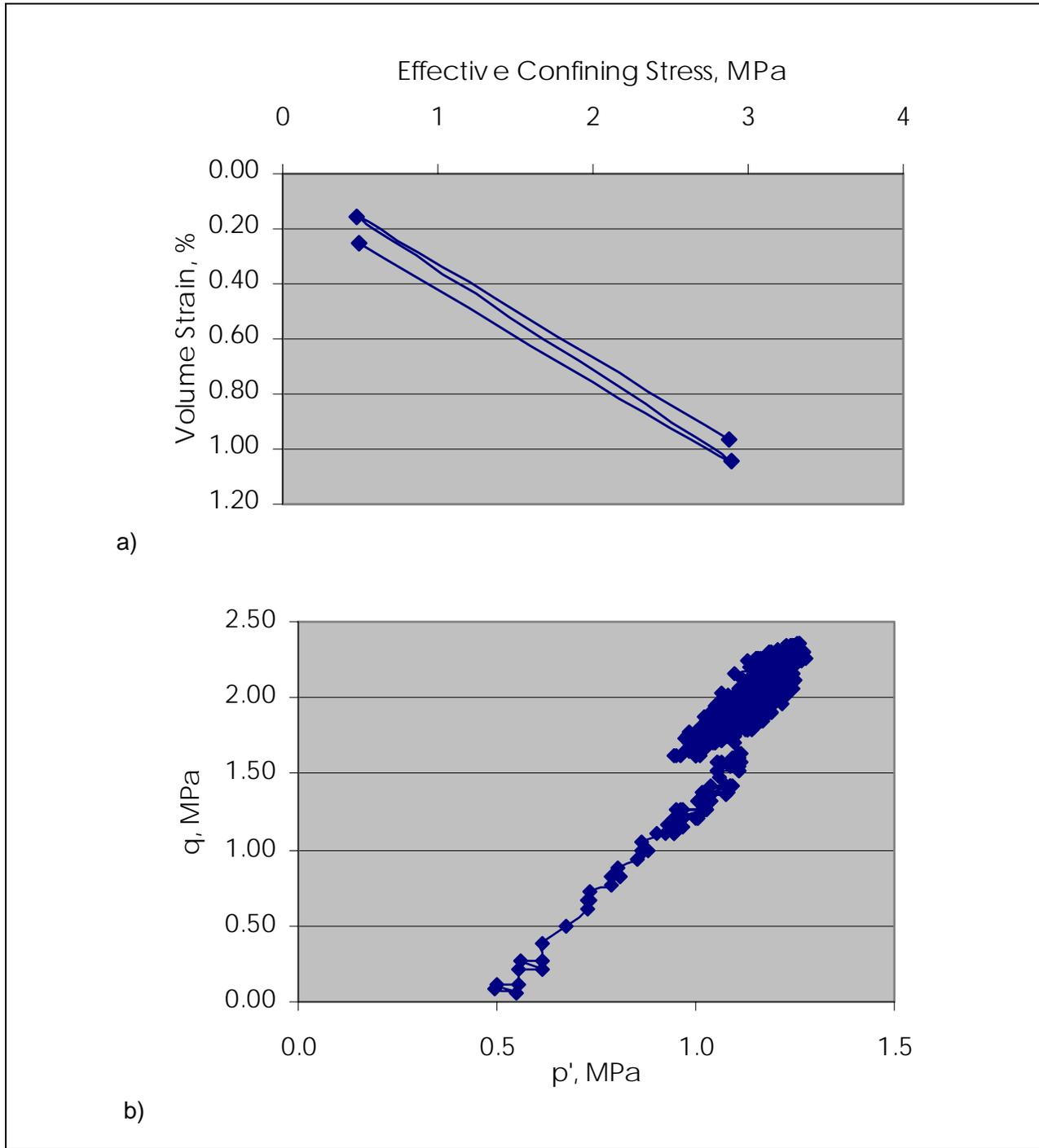
Figure 49. NTX3 triaxial test results a) compressibility b) stress path
