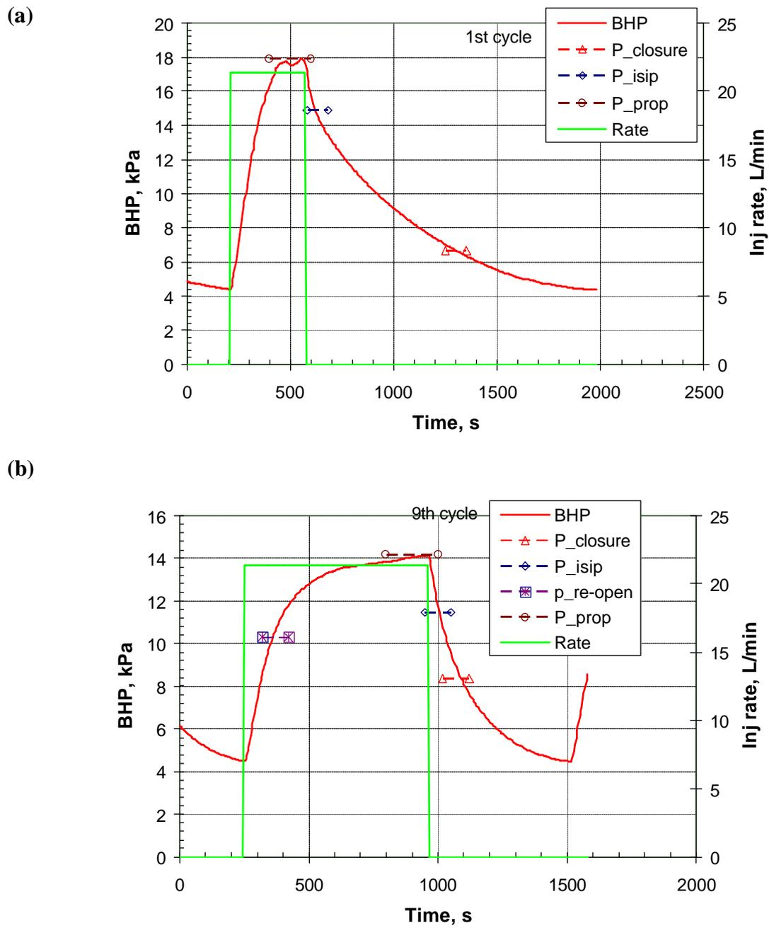
Figure 4: Comparison of pressure behaviour during injection for cycle #1 (a) and cycle #9 (b).
