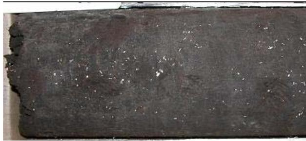
Figure 25. Interbedded mudstone/oil sands Sample SC13 (from Paramount Leismer 03-03-79-10W4M)
