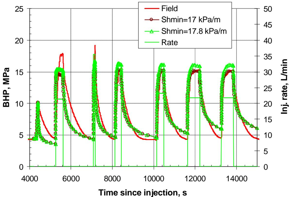
**Figure 10:** Effect of varying the SHmin in matching the field data.
