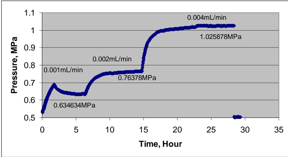
Figure 82. ST3 permeability test results
