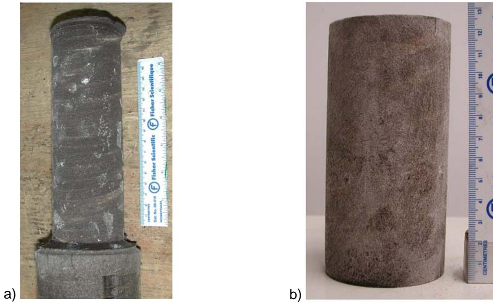
Figure 35. NTX1 test specimen a) frozen, lathed specimen b) final trimmed frozen bitumen saturated specimen
