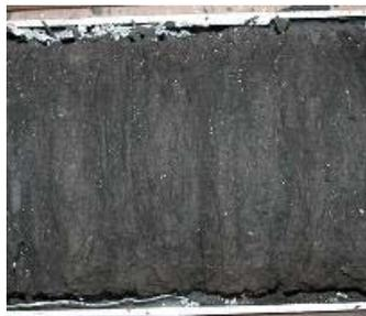
Figure 20. Interbedded mudstone/oil sands Sample SC8 (from Paramount Leismer 03-03-79-10W4M)
