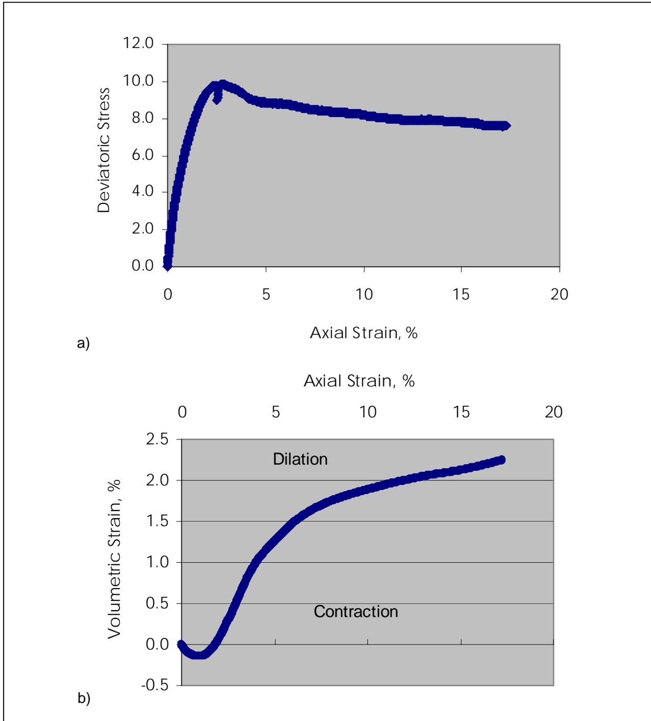
Figure 39. NTX1 triaxial test results a) stress-strain b) volume change
