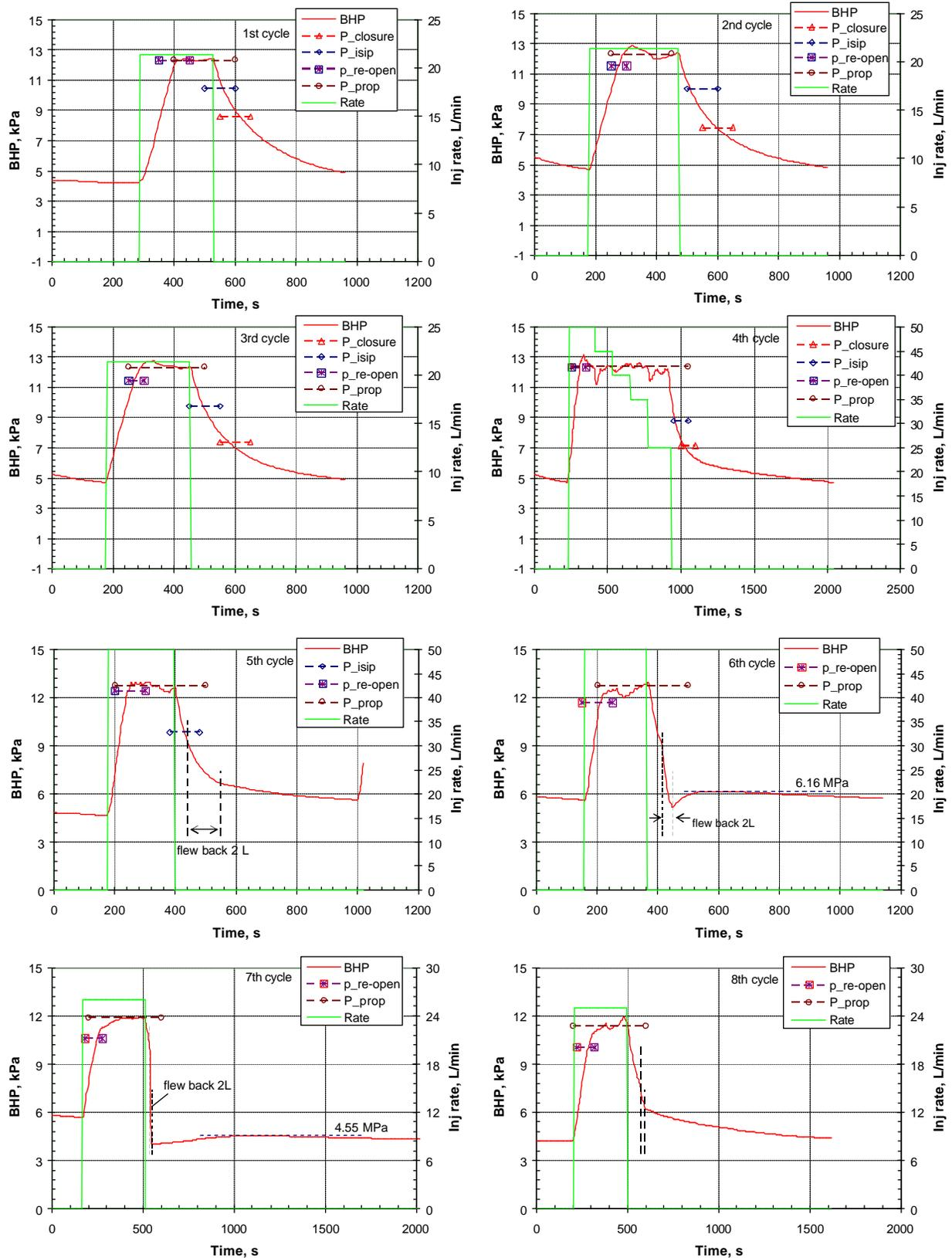
**Figure A.9:** Characteristic pressures determined from the various injection/shut-in cycles in testing the shaly facie (399 mTVD) at well 12-27.
