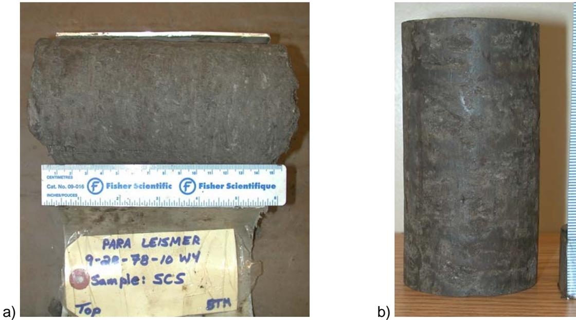
Figure 73. ST2 test specimen a) just after removal from liner b) after cutting specimen
