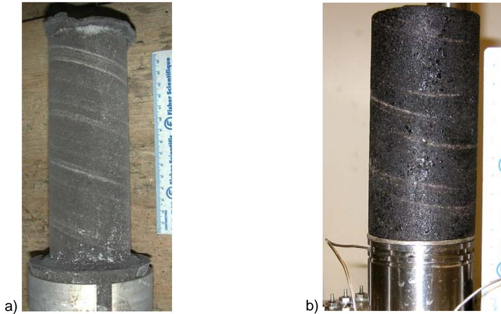
Figure 41. NTX2 test specimen a) frozen, lathed specimen b) final trimmed frozen bitumen saturated specimen
