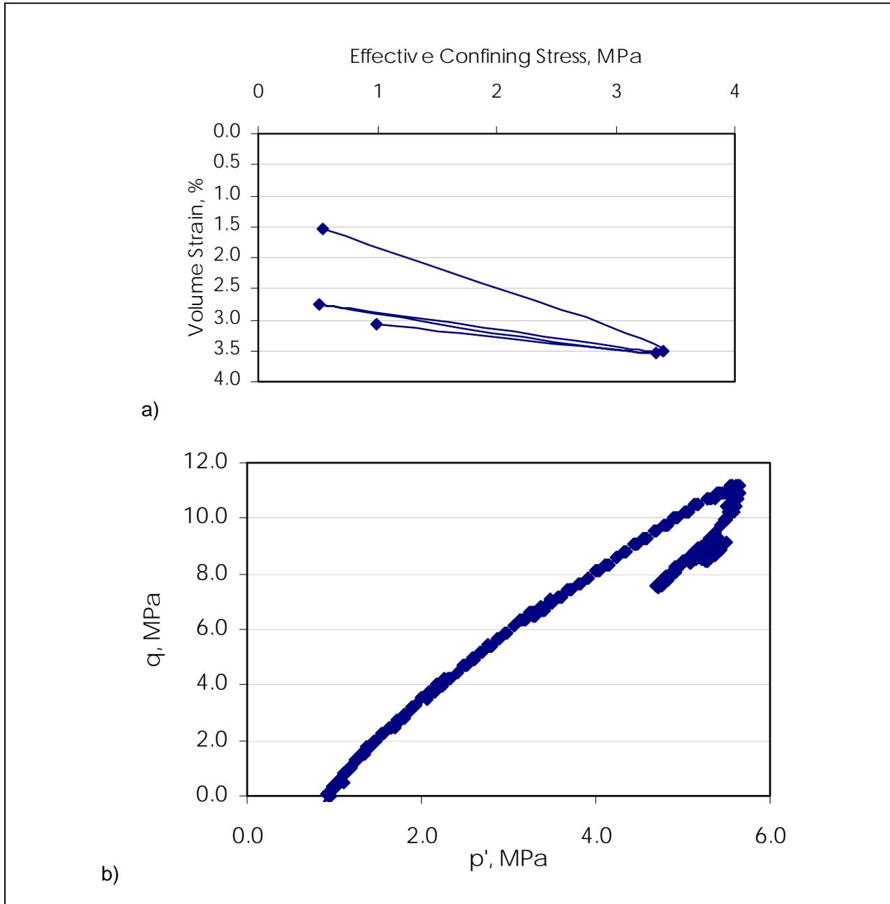
Figure 80. ST3 triaxial test results a) compressibility b) stress path
