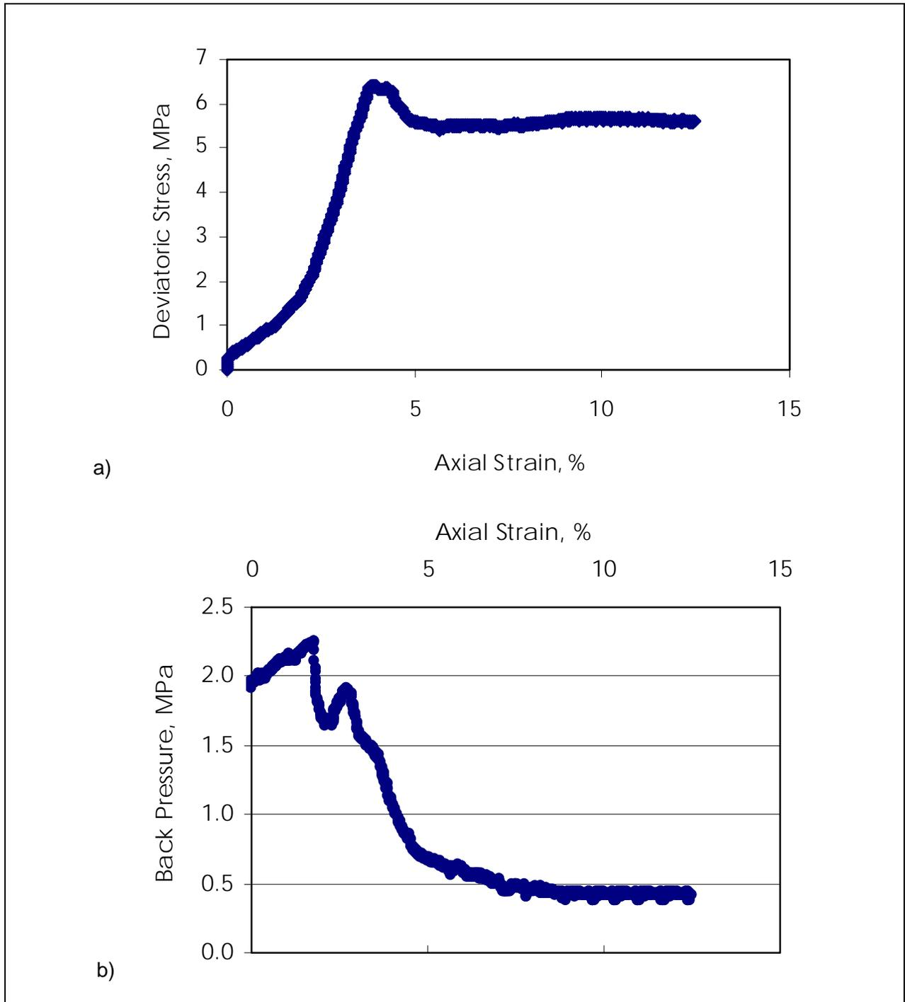
Figure 71. ST1 triaxial test results a) stress-strain b) volume change
