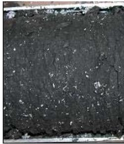
Figure 21. Interbedded mudstone/oil sands Sample SC9 (from Paramount Leismer 03-03-79-10W4M)
