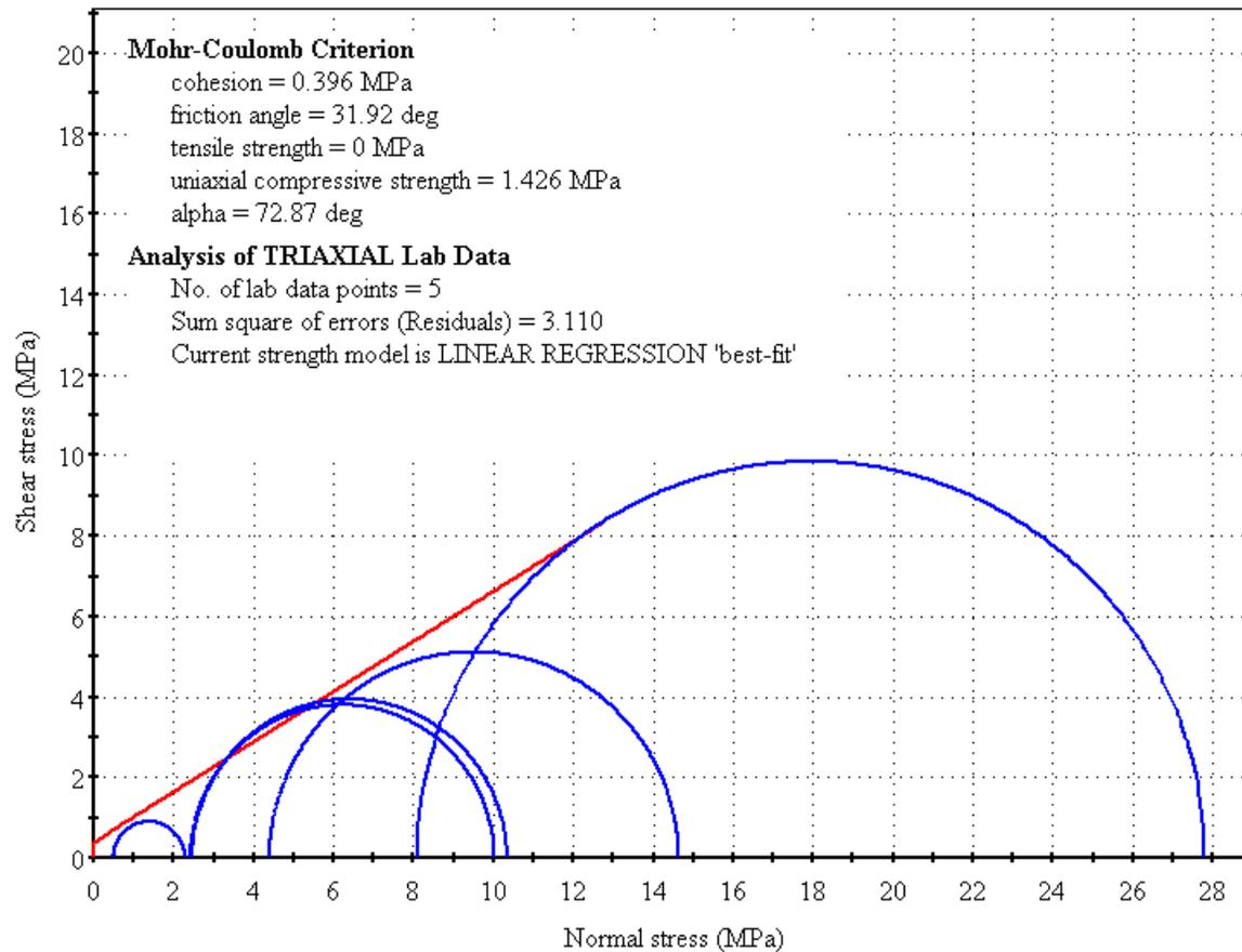
**Figure 4.6: Mohr-Coulomb failure envelope fit to residual triaxial test results on McMurray Formation oil sands samples from Paramount Leismer 09-28-78-10W4M (depth range: 420.9 mKB to 427.3 mKB). Data from U of A (2005)**
