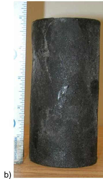
Figure 46. NTX3 test specimen a) frozen, lathed specimen b) final trimmed frozen bitumen saturated specimen
