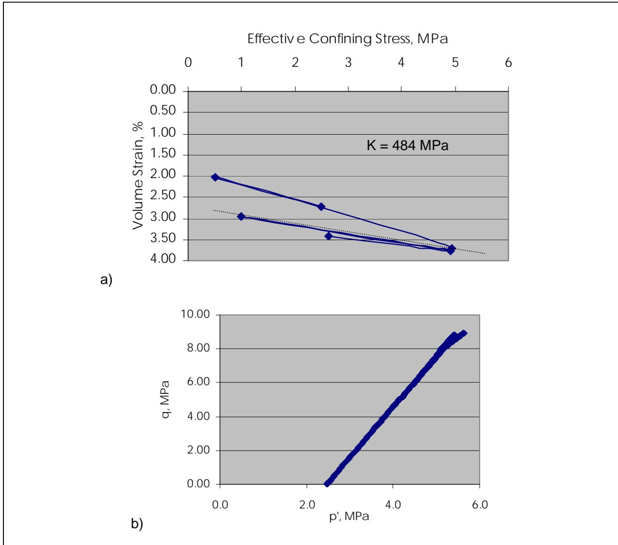
Figure 43. NTX2 triaxial test results a) compressibility b) stress path
