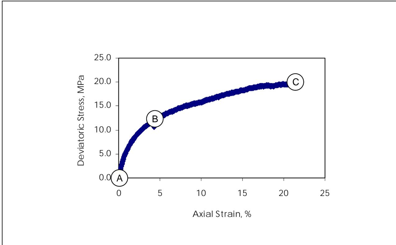
Figure 63. Locations in stress-strain curve where permeability measurements were taken on specimen NTX5
