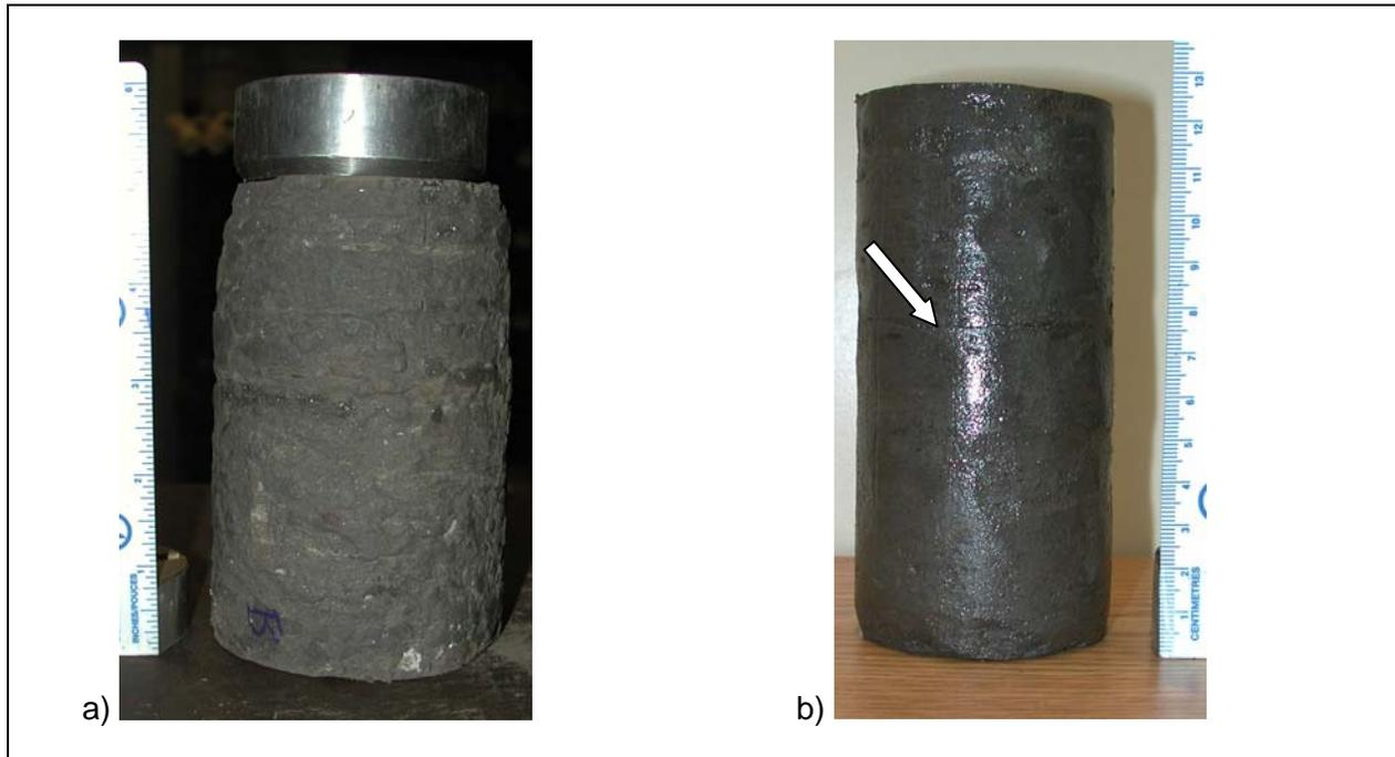
Figure 68. ST1 test specimen a) just after removal from liner b) after cutting (arrow denotes location of horizontal fracture in specimen)
