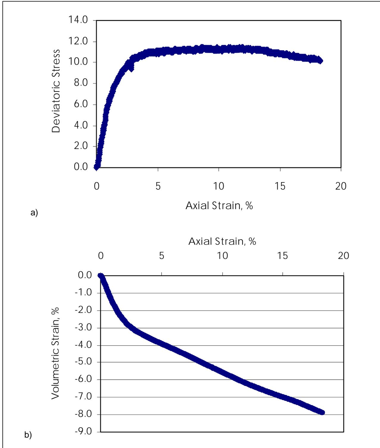
Figure 56. NTX4 triaxial test results a) stress-strain b) volume change
