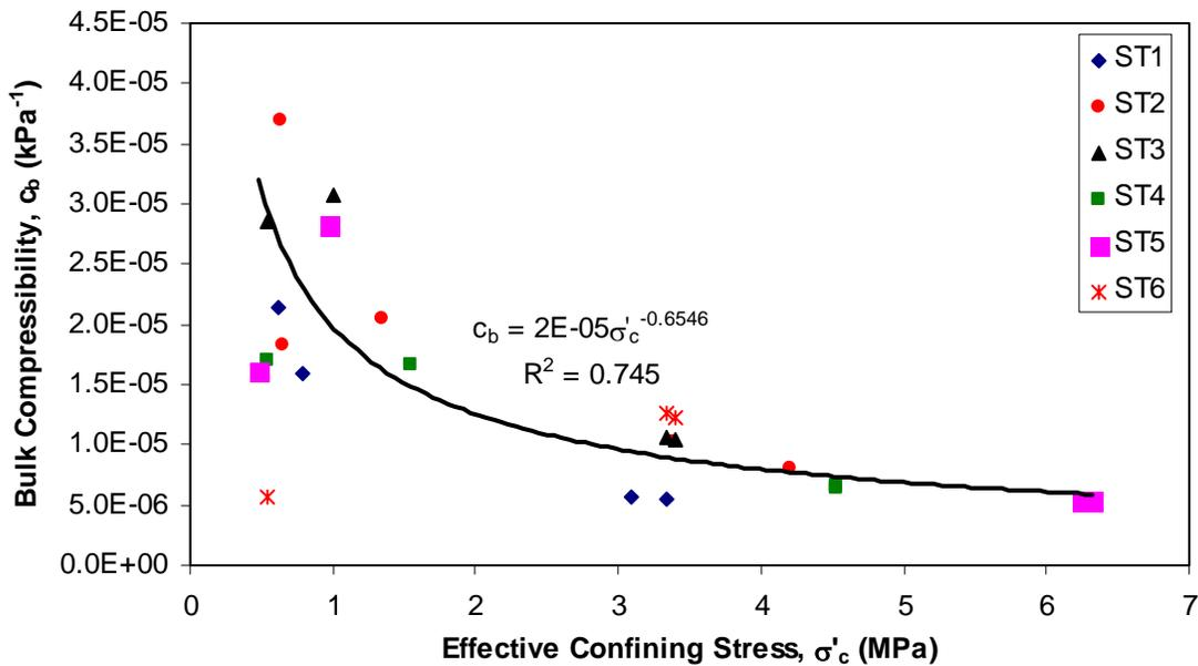
Figure 4.2: Bulk compressibility of mudstone samples as a function of effective confining stress during isotropic loading unloading tests.
