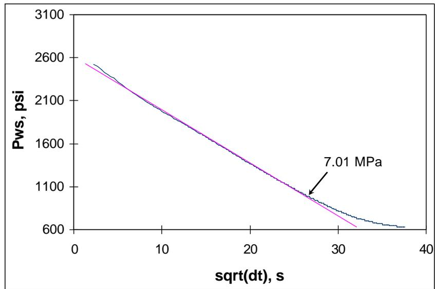
**Figure A.3:** An example pressure vs.  $\sqrt{dt}$  plot to select the fracture closure pressure.
