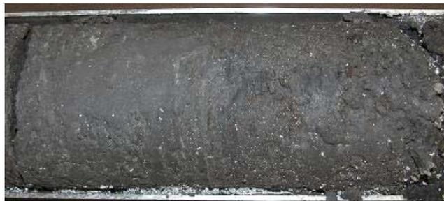
Figure 16. Interbedded mudstone/oil sands Sample SC4 (from Paramount Leismer 09-28-78-10W4M)
