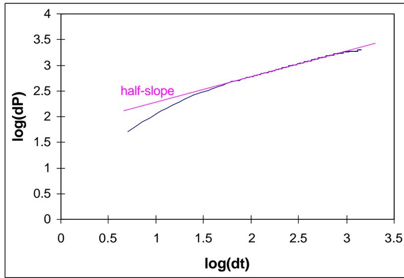
**Figure A.4:** When the data quality permits, a log-log plot on the pressure decline vs. time data can be used to aid selection of the linear flow regime and therefore, the fracture closure pressure.
