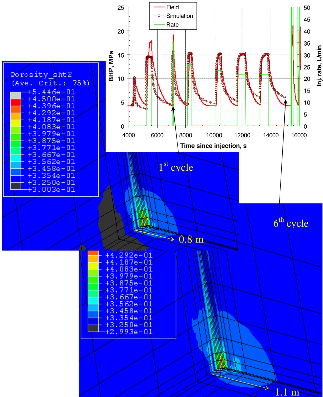
**Figure 15:** Extent of fracture propagation as marked by the high-porosity zone. The contour plots denote the porosity.
