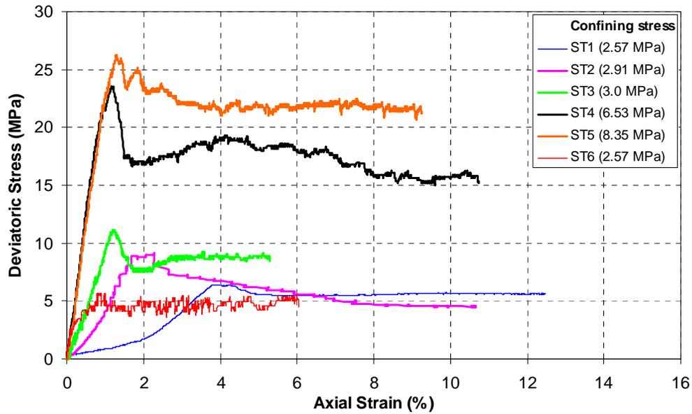
Figure 4.7: Stress-strain behaviour of McMurray Formation mudstone samples from Paramount Leismer 09-28-78-10W4M (depth range: 394.56 mKB to 397.75 mKB) during undrained triaxial tests. Data from U of A (2005).
