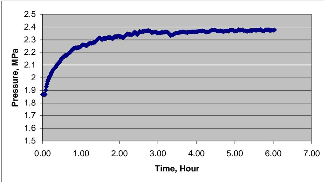
Figure 92. ST5 permeability test results
