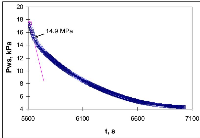
**Figure A.2:** An example pressure vs. time Cartesian plot aiding detection of the instantaneous shut-in pressure from the pressure decline data in a hydraulic fracturing stress test.
