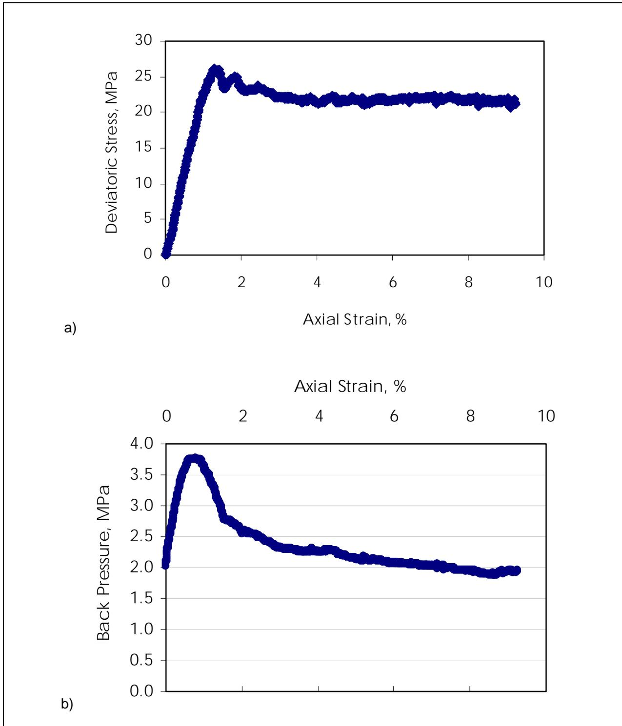
Figure 91. ST5 triaxial test results a) stress-strain b) volume change
