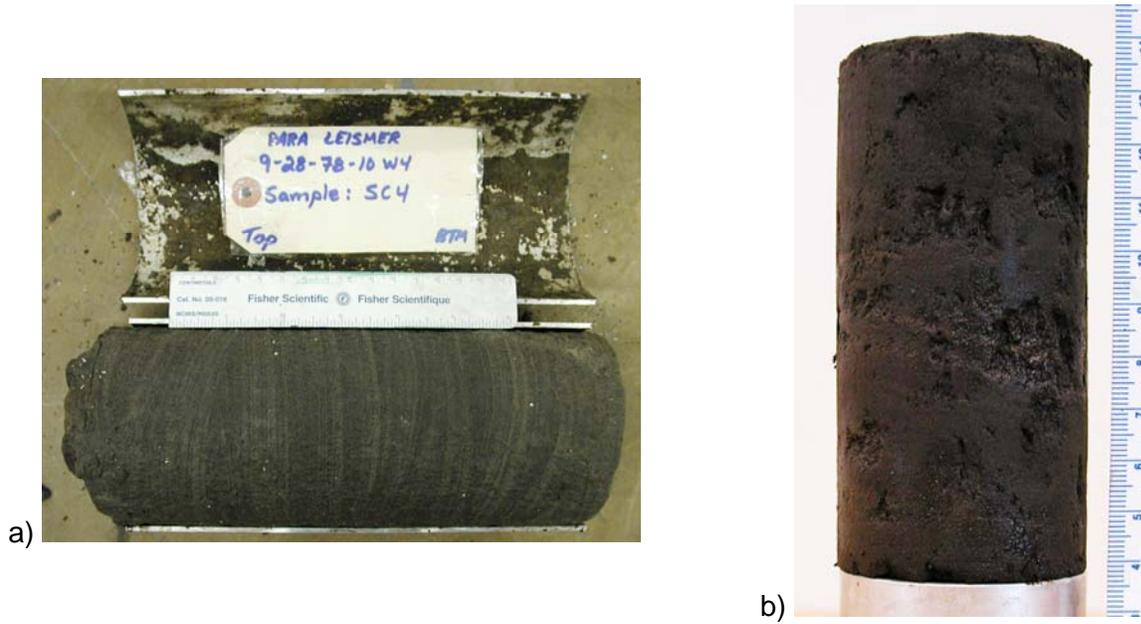
Figure 83. ST4 test specimen a) just after removal from liner b) after cutting (lithology of sample made cutting of specimen difficult, as evidenced by uneven exterior of specimen)
