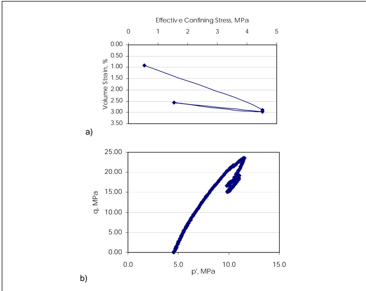
Figure 85. ST4 triaxial test results a) compressibility b) stress path
