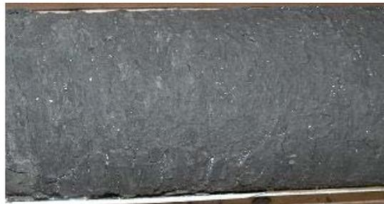
Figure 23. Interbedded mudstone/oil sands Sample SC11 (from Paramount Leismer 03-03-79-10W4M)
