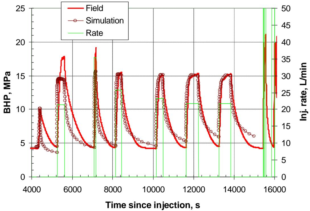
**Figure 7:** Comparison in the bottomhole pressure response between the simulated and field-recorded during the injection test in the oil sands facie at 420 mTVD at well 4-27.
