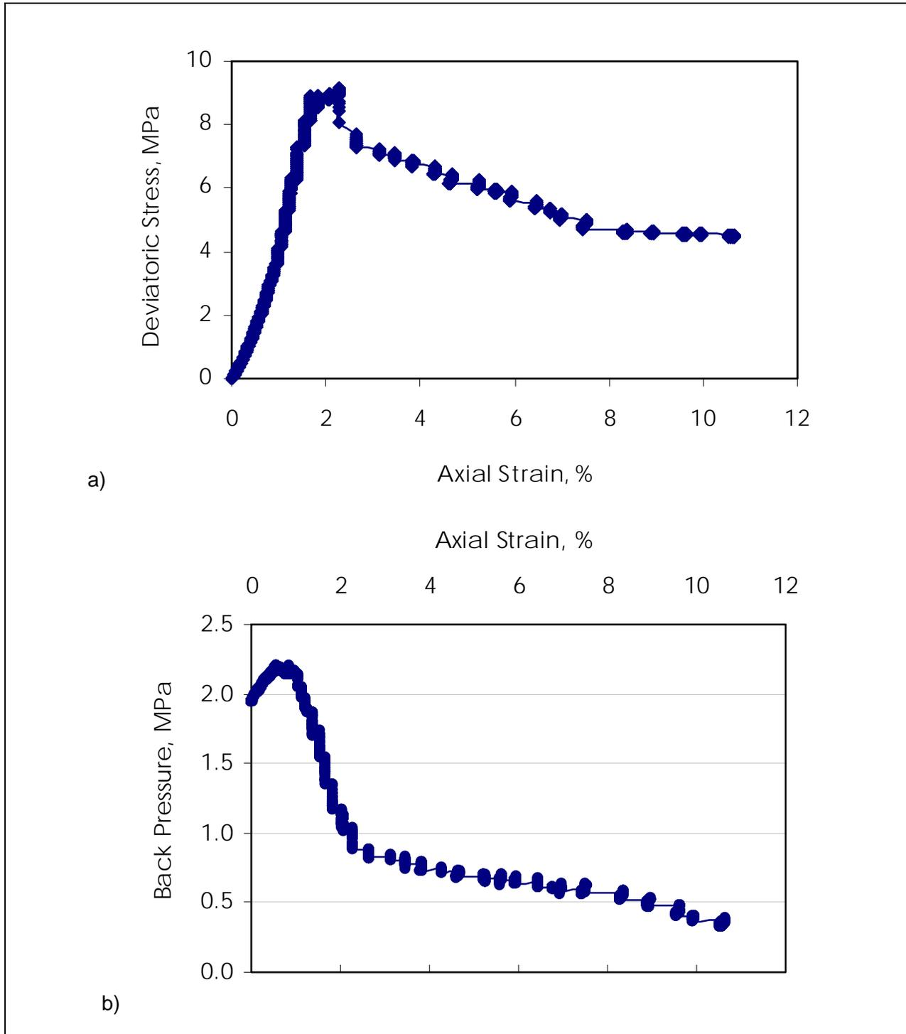
Figure 76. ST2 triaxial test results a) stress-strain b) volume change
