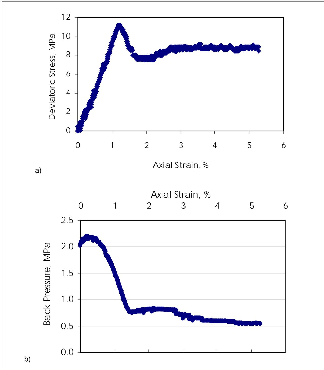
Figure 81. ST3 triaxial test results a) stress-strain b) volume change
