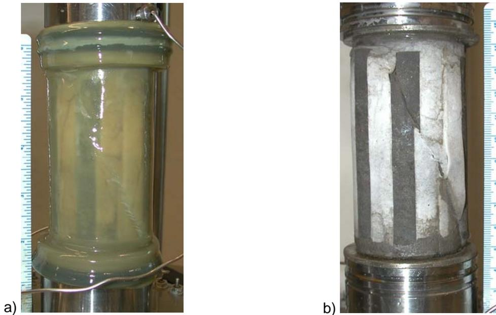
Figure 79. ST3 test specimen a) post-test specimen still inside membrane b) post-test specimen with membrane removed showing deformed state of specimen
