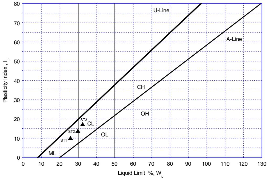
Figure 33. Plasticity chart used for soil classification of shale specimens
