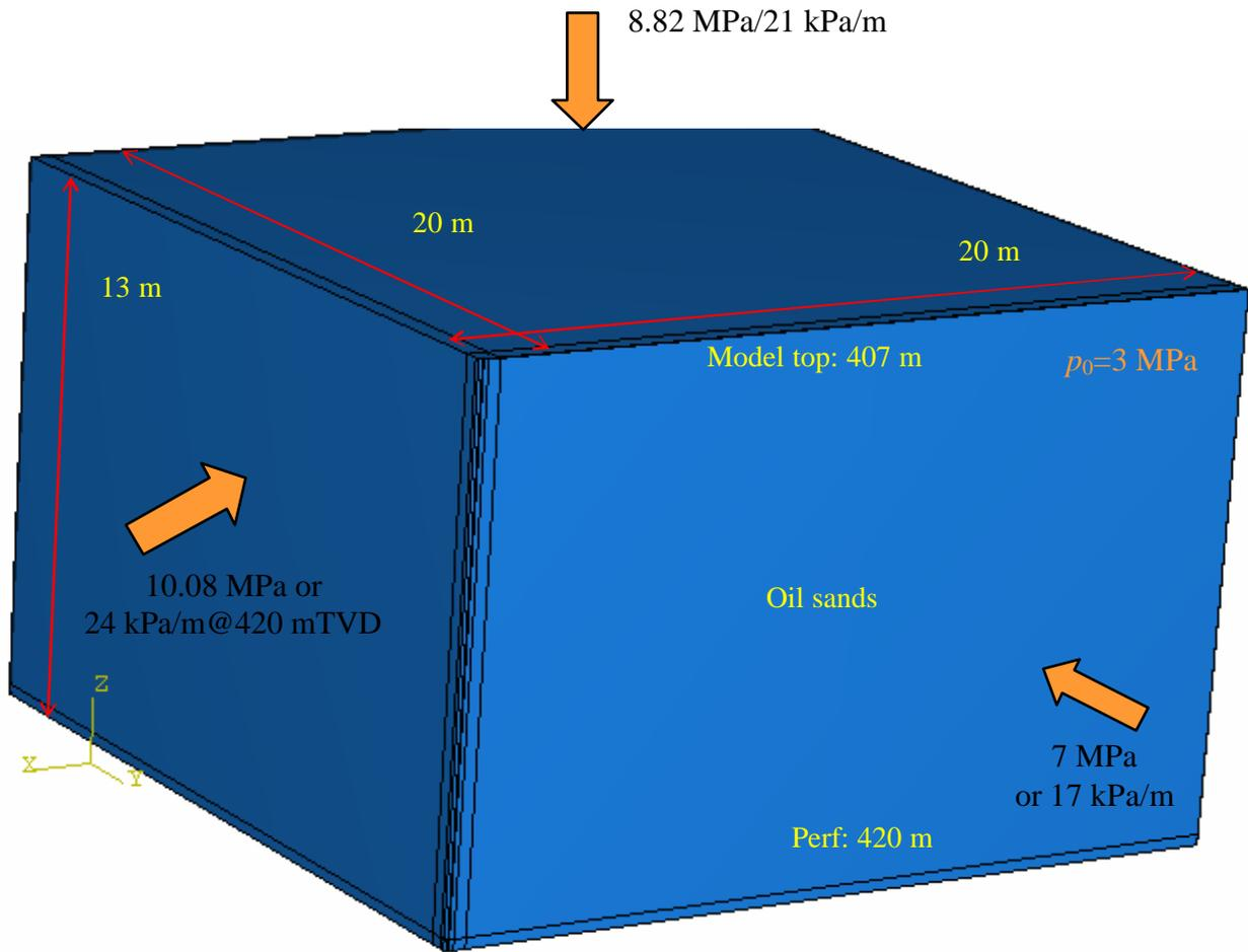
**Figure 8:** Geometry of the simulation model used in the history-matching shown in Figure 8. Please refer to Figure 1 for a log representation of the well. A quarter model is used because of the symmetry.
