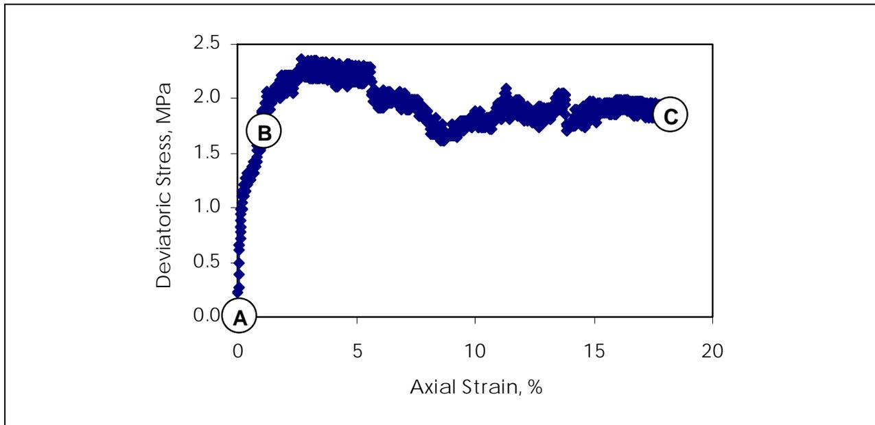
Figure 51. Locations in stress-strain curve where permeability measurements were taken on specimen NTX3
