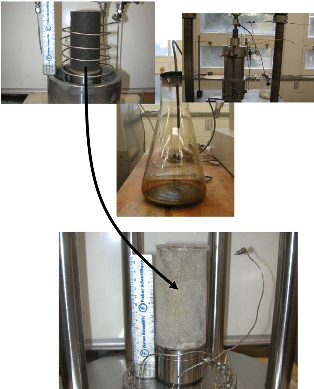
Figure 34. Demonstration of bitumen flushing efficiency for triaxial specimens
