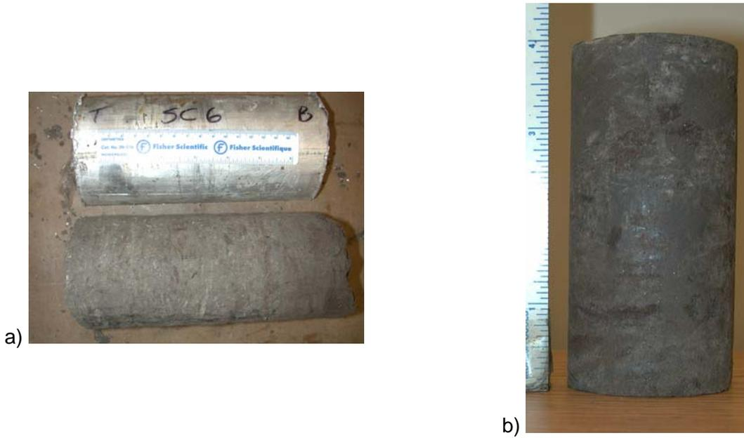
Figure 78. ST3 test specimen a) just after removal from liner b) after cutting specimen
