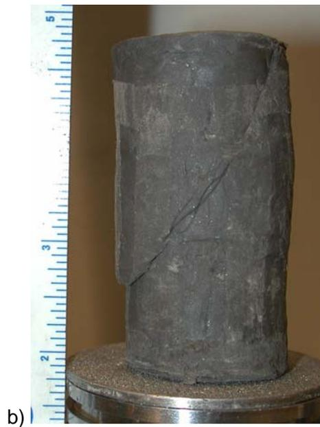
Figure 94. ST6 test specimen a) post-test specimen still inside membrane b) post-test specimen with membrane removed showing deformed state of specimen
