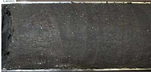
Figure 13. Interbedded mudstone/oil sands Sample SC1 (from Paramount Leismer 09-28-78-10W4M)
