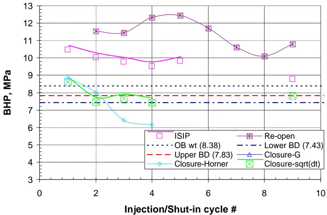
**Figure 6:** Various characteristic pressures interpreted from the hydraulic fracturing stress test in the shaly facie at 399 mTVD at well 12-27.
