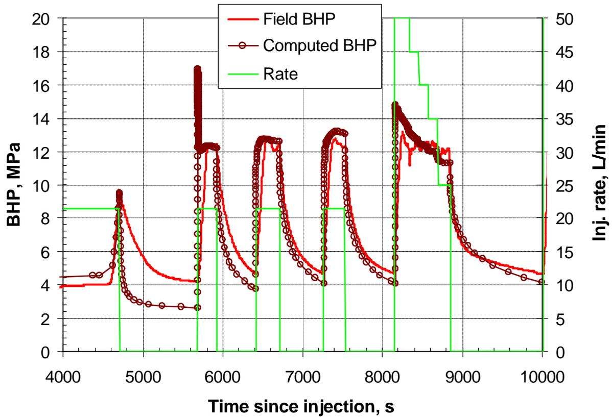
**Figure 16:** Comparison in the bottomhole pressure response between the simulated and field-recorded during the injection test in the shaly facie at 399 mTVD at well 12-27.
