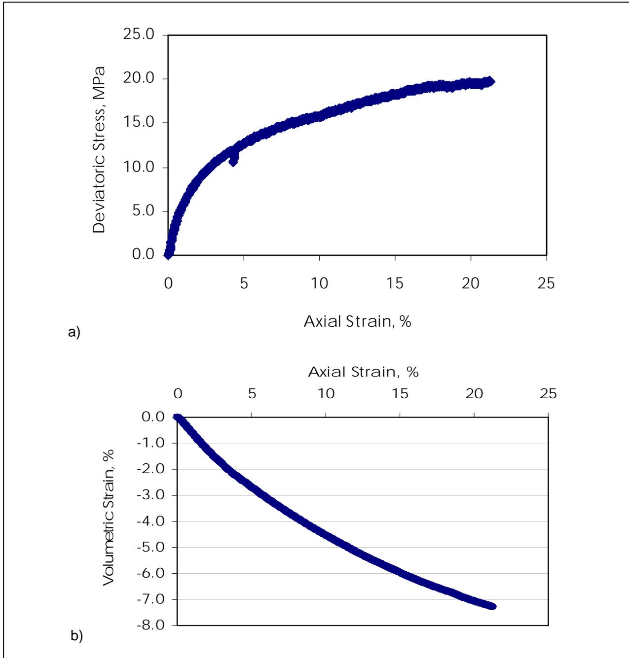
Figure 62. NTX5 triaxial test results a) stress-strain b) volume change
