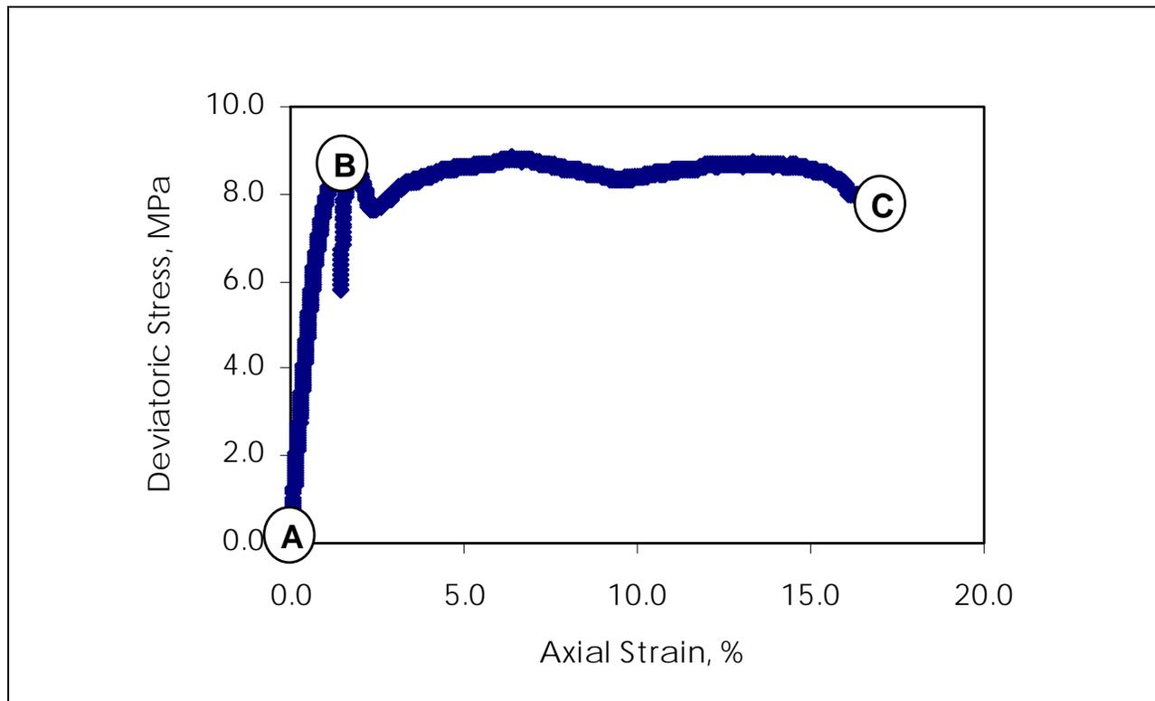
Figure 45. Locations in stress-strain curve where permeability measurements were taken on specimen NTX2
