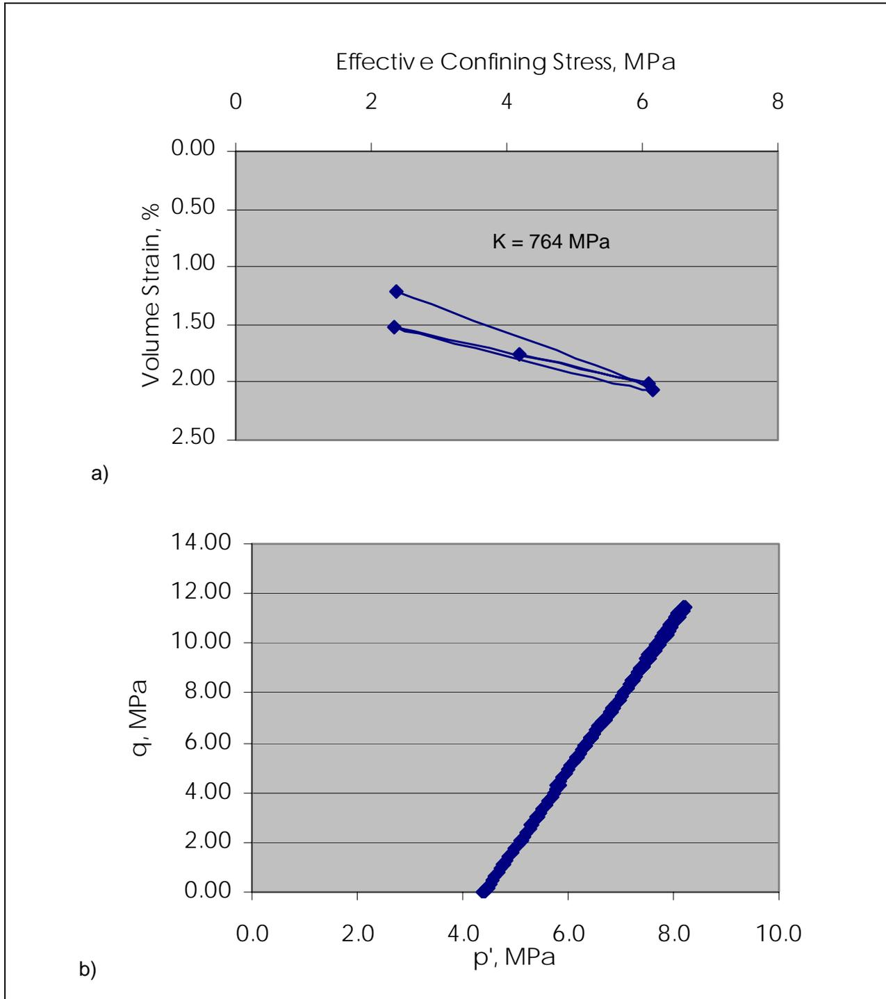
Figure 55. NTX4 triaxial test results a) compressibility b) stress path
