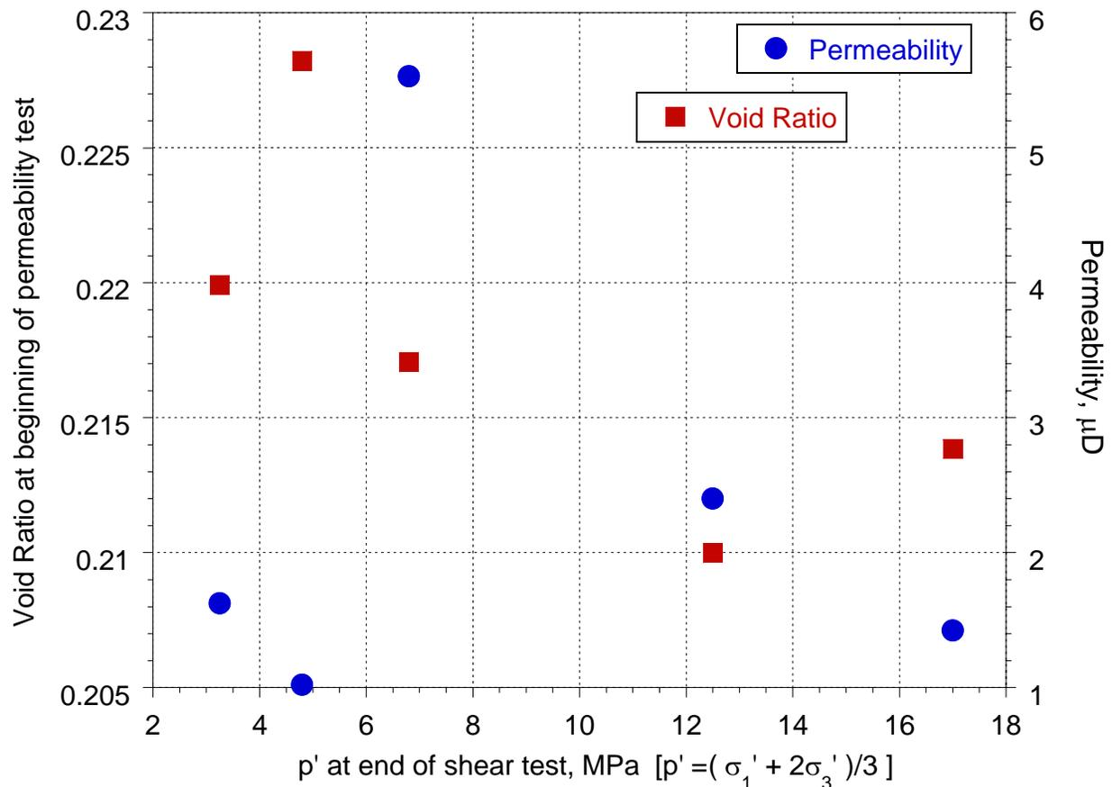
Figure 101. Variation of effective permeability to water with void ratio and mean effective confining stress at end of triaxial shear test.
