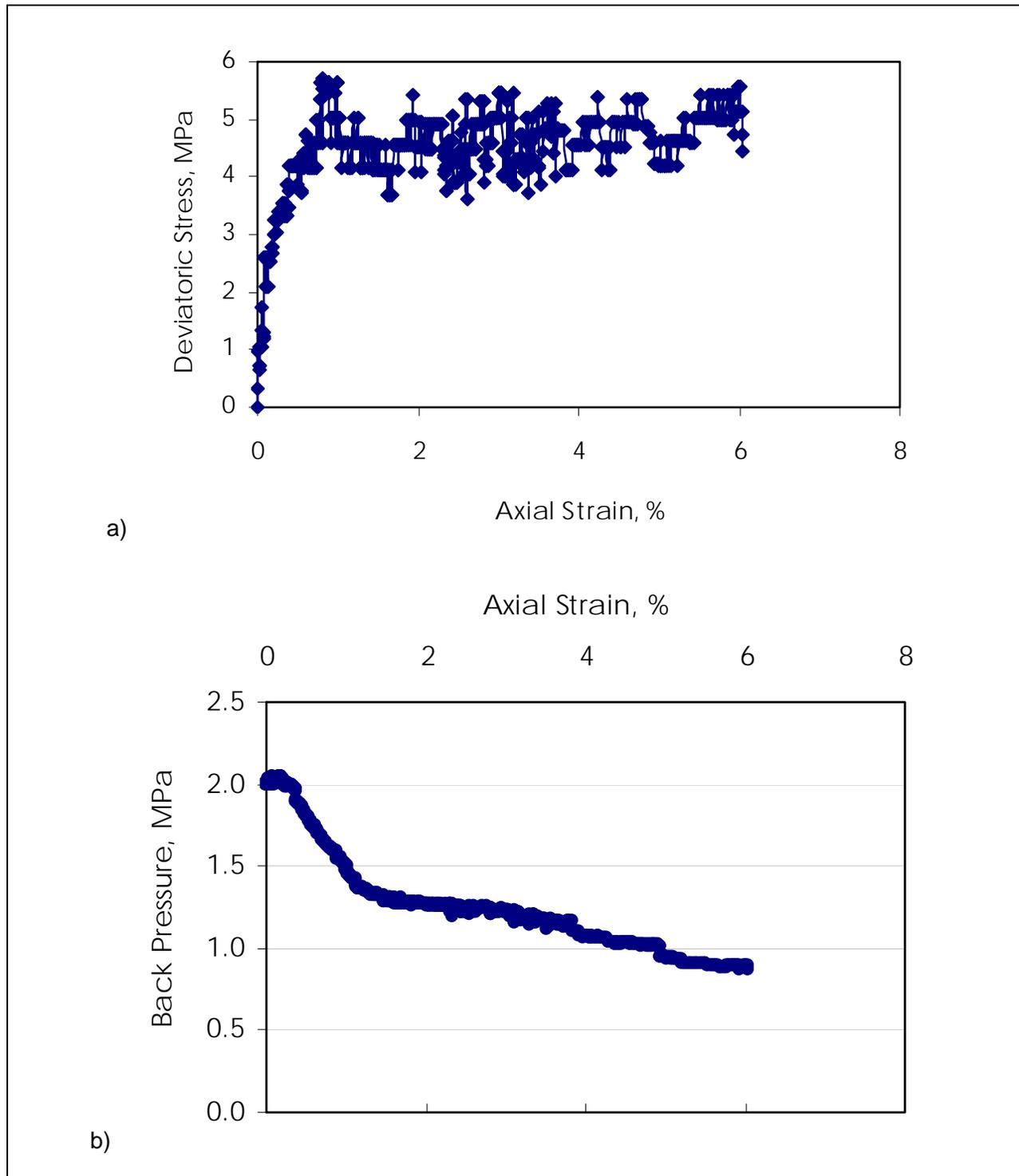
Figure 96. ST6 triaxial test results a) stress-strain b) volume change
