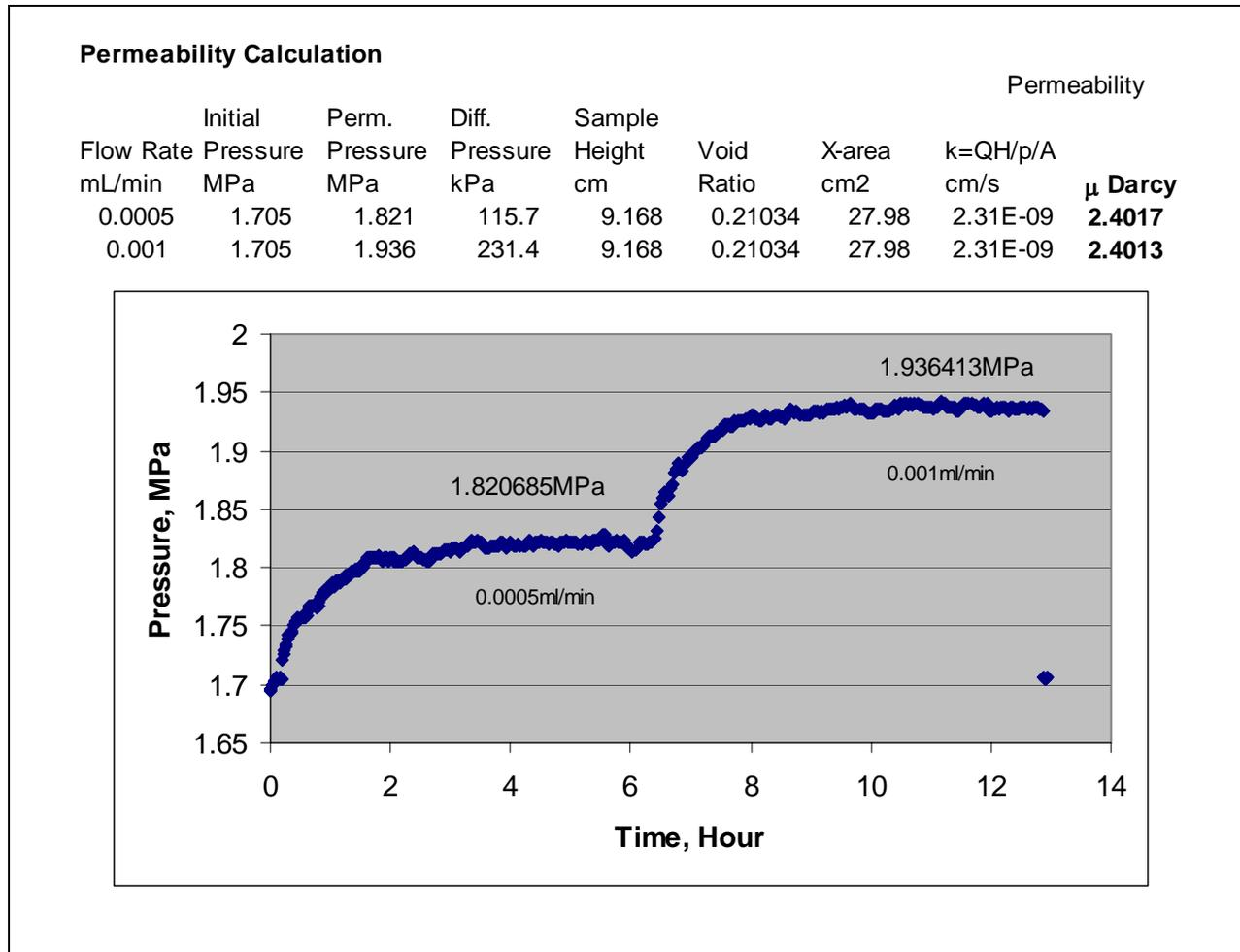
Figure 87. ST4 permeability test results
