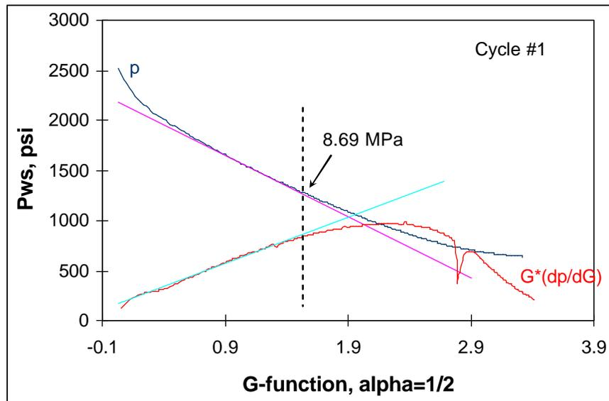
**Figure A.5:** An example G-plot used to determine the fracture closure pressure.
