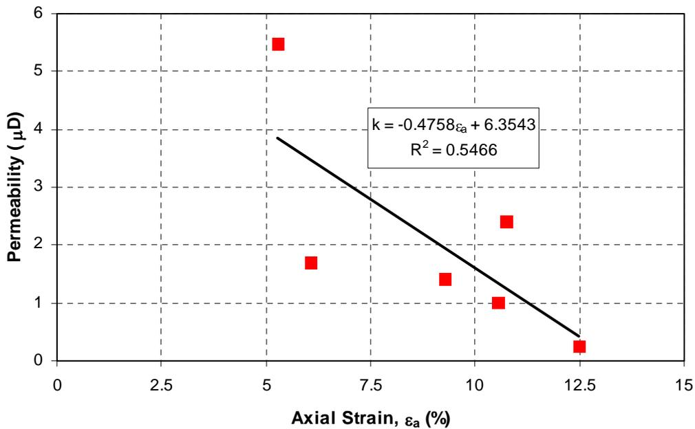
**Figure 4.12: Change of permeability ( $k$ ) as a function of axial strain ( $\epsilon_a$ ) in McMurray Formation mudstone samples measured at residual strength condition in undrained triaxial tests. Data from U of A (2005).**
