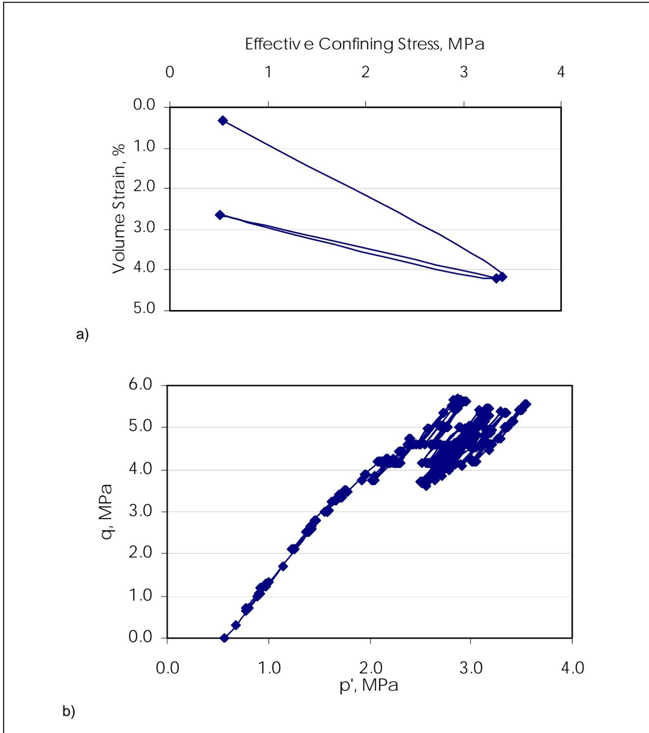
Figure 95. ST6 triaxial test results a) compressibility b) stress path
