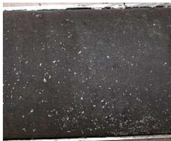
Figure 28. Interbedded mudstone/oil sands Sample SC16 (from Paramount Leismer 03-03-79-10W4M)
