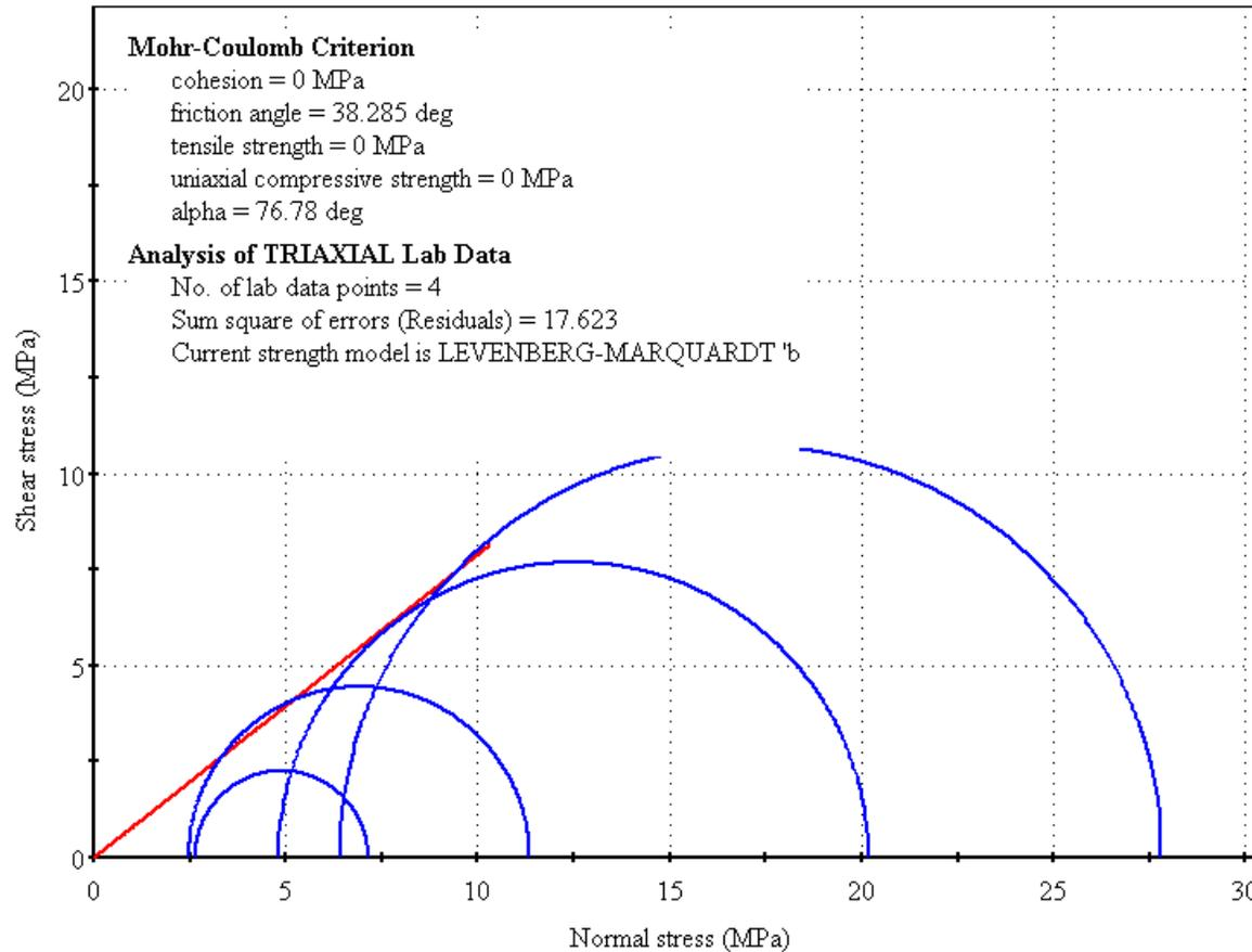
**Figure 4.4: Mohr-Coulomb failure envelope fit to residual triaxial test results on McMurray Formation mudstone samples from Paramount Leismer 09-28-78-10W4M (depth range: 394.56 mKB to 397.75 mKB). Data from U of A (2005)**
