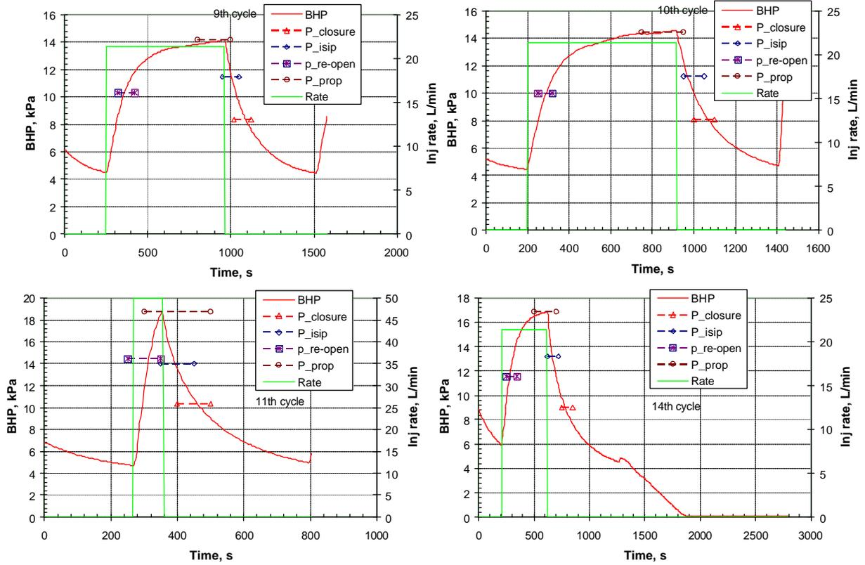
**Figure A.8 (cont'd):** Characteristic pressures determined from the various injection/shut-in cycles in testing the oil sands facie (420 mTVD) at well 4-27.
