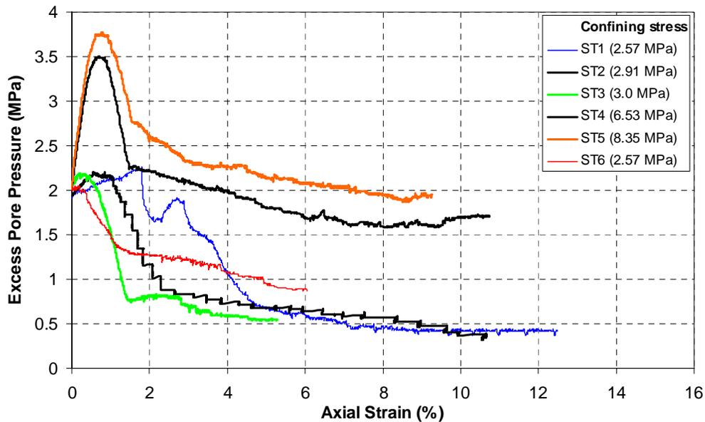
Figure 4.8: Excess pore pressure development as a function of axial strain in McMurray Formation mudstone samples from Paramount Leismer 09-28-78-10W4M (depth range: 394.56 mKB to 397.75 mKB) during undrained triaxial tests. Data from U of A (2005).
