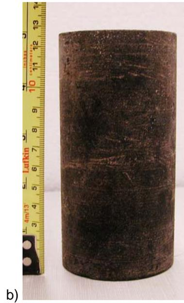
Figure 52. NTX4 test specimen a) frozen, lathed specimen b) final trimmed frozen bitumen saturated specimen
