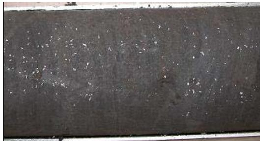
Figure 27. Interbedded mudstone/oil sands Sample SC15 (from Paramount Leismer 03-03-79-10W4M)
