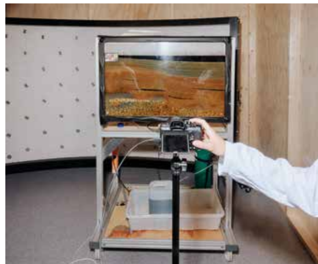
RESERVOIR MODEL: The model makes it possible to study floating patterns of CO 2 and water, which is used, together with mathematical models, to improve understanding and usage of simulation tools. Photo: Einar Aslaksen.
