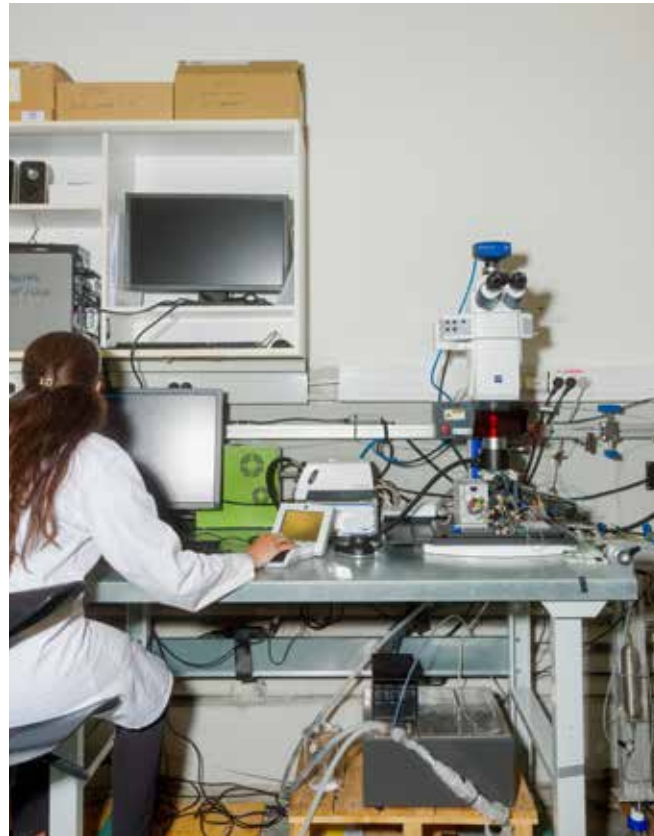
EXPERIMENT: Here, experiments with storing CO 2 in sandstone are conducted. The displacement of water by CO 2 is studied in a microscope, to better understand the mechanisms in small pores. Later, the process is physically scaled up and studied on a meter-sized scale. Photo: Einar Aslaksen.
