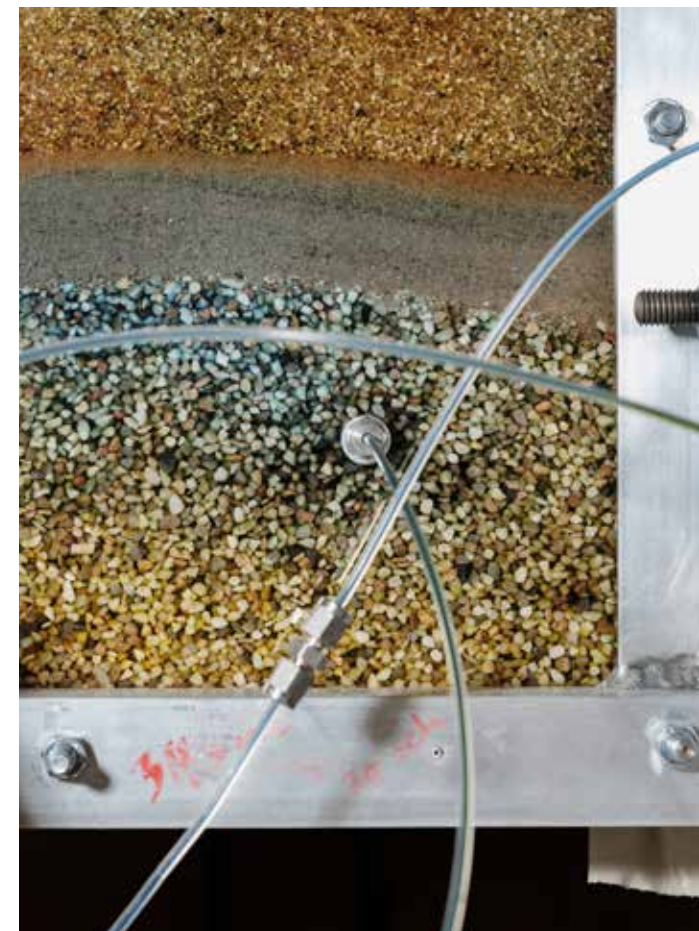
In the reservoir model studied by Martin Fernø and his colleagues, CO 2 is pumped into a reservoir filled with water, displacing the water as CO 2 is stored in the geological layers. Photo: Einar Aslaksen.
