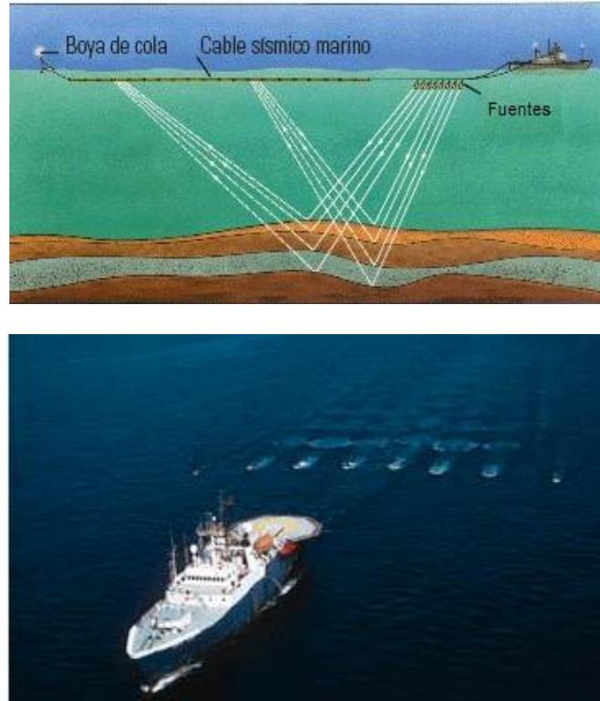
**Figure 5. Scheme and photograph of a seismic vessel, the emission sources, the seismic cable (streamers) and the tail buoy.**
