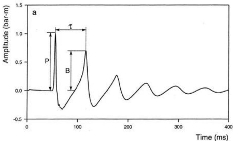
**Figure 19. Pressure signature of a compressed air power source in the near field.**
