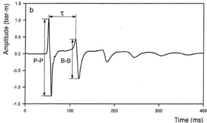
Figure 20. Pressures signature of a compressed air power source in the far field.
