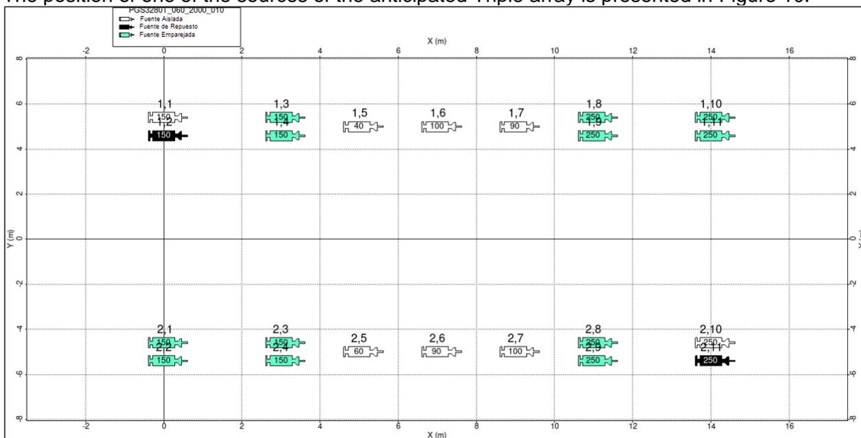
**Figure 10. Emitting sub-array of the Triple array of compressed air power sources. 3,280 cu.in Volume.**
