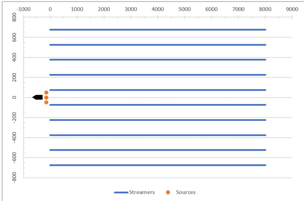
Figure 9. Layout diagram of compressed air energy sources (sources) and streamers.
