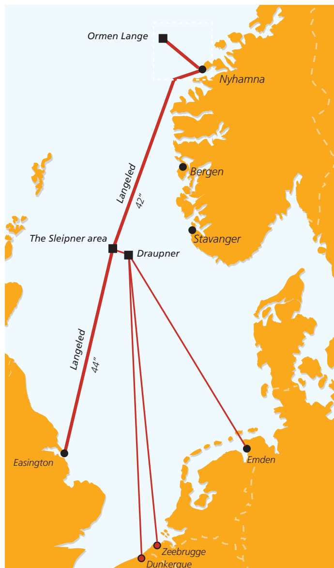
The gas trunkline from Ormen Lange will be laid via Sleipner to the UK. This decision strengthens Sleipner's position as a gas hub in the North Sea. Gas from other fields can be mixed with the gas from Ormen Lange, and gas from this field can be delivered to other markets.
