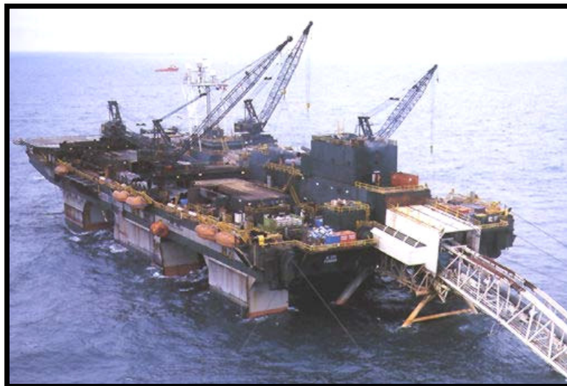
Figure 3.4 Stolt Offshore LB200 Lay Barge
