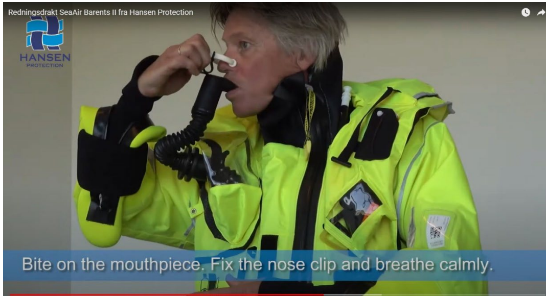
Figure 3-21 Integrated emergency breathing system in SeaAir Barents II survival suit (source: YouTube video from Hansen Protection, Ref /75/)
