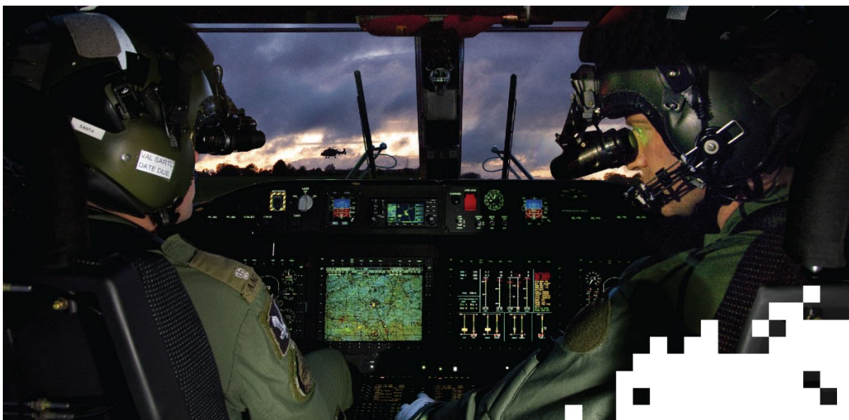
Figure 3-15 Night vision goggles (NVG) for helicopter pilots (source: Leonardo helicopters website, Ref /81/)
