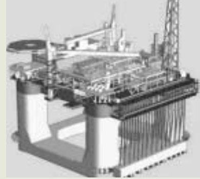
The Kristin gas and condensate field on the Halten Bank will be developed with 12 subsea wells tied back to a floating production platform. Due to come on stream in 2005, the Statoil-operated project will cost NOK 17 billion.
