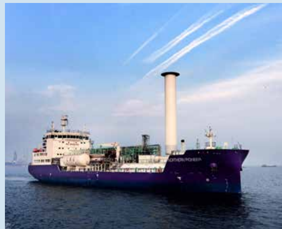
Northern Pioneer is the world's first dedicated CO 2 transport vessel for commercial storage.
