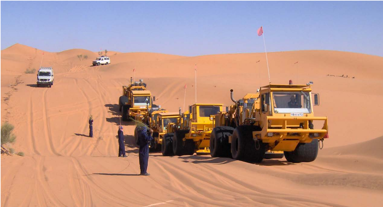
Figure 3.17 A fleet of vibrator trucks
