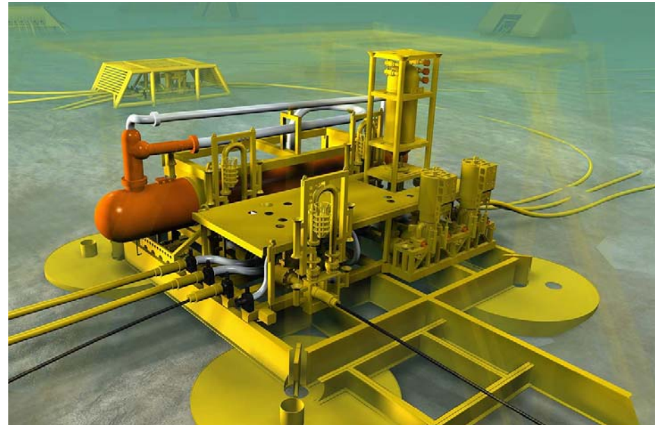
Tordis sub sea separation facility
