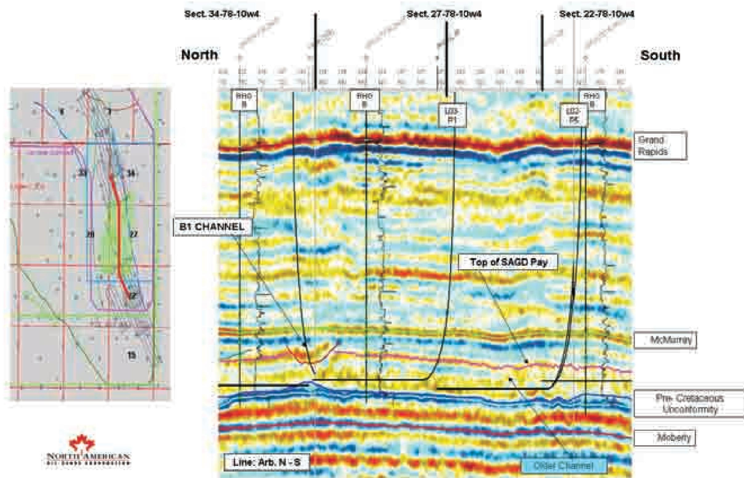
Figure B4.1 - 13 NS Seismic Profile
