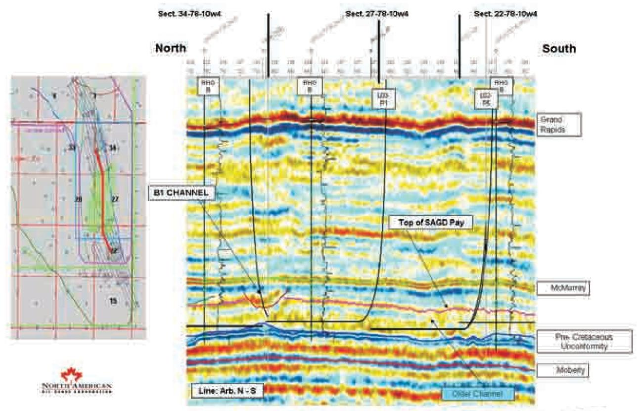
Figure B4.1 - 13 NS Seismic Profile
