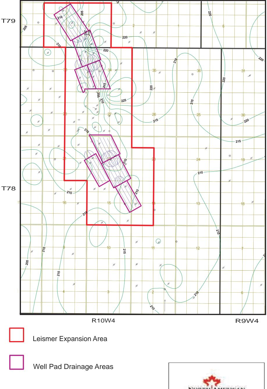
Figure B4.1-23 Drainage Pads and Horizontal Well Pairs with Base SAGD Structure
