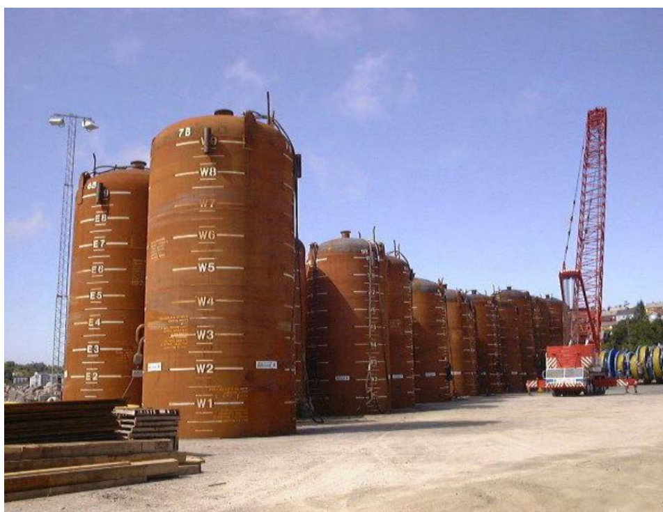
Figure 4-3 Illustration of suction anchor
