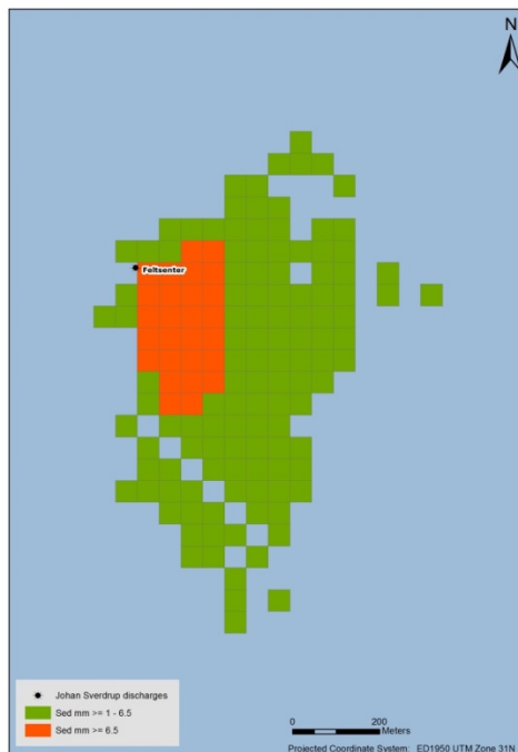
Figure 5-55 Areas where modelled sedimentation rates is 1-6.5 mm and >6.5 mm, simulation 1 discharge from 6 wells at Field-center.
