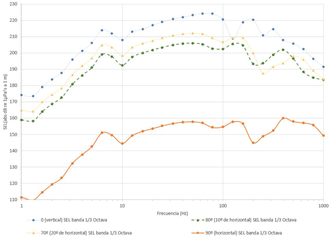
**Figure 12. Energy per octave for different angles in 0° Azimuth (forward direction).**
