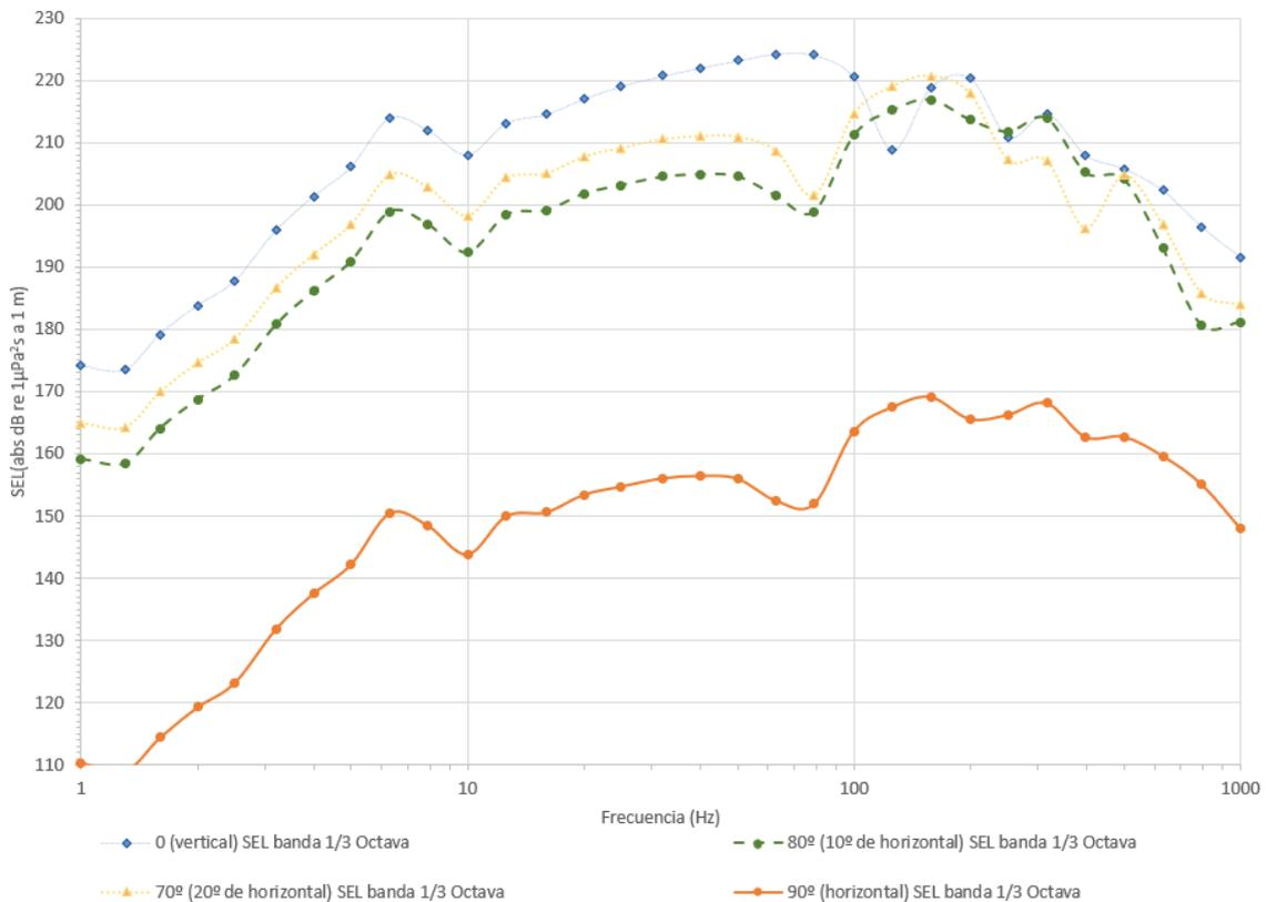
**Figure 13. Energy per octave for different angles in 90° Azimuth (perpendicular to the advance).**
