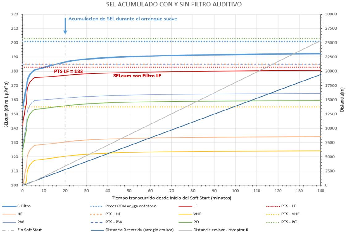
**Figure 38. CAN\_114. Accumulated SEL. 20-minute Soft Start. Initial position of the receiver 400 m away from the emitter, perpendicular to the advance line at the Soft Start starting point. 90° at 2 m / s Azimuth movement of the receiver.**
