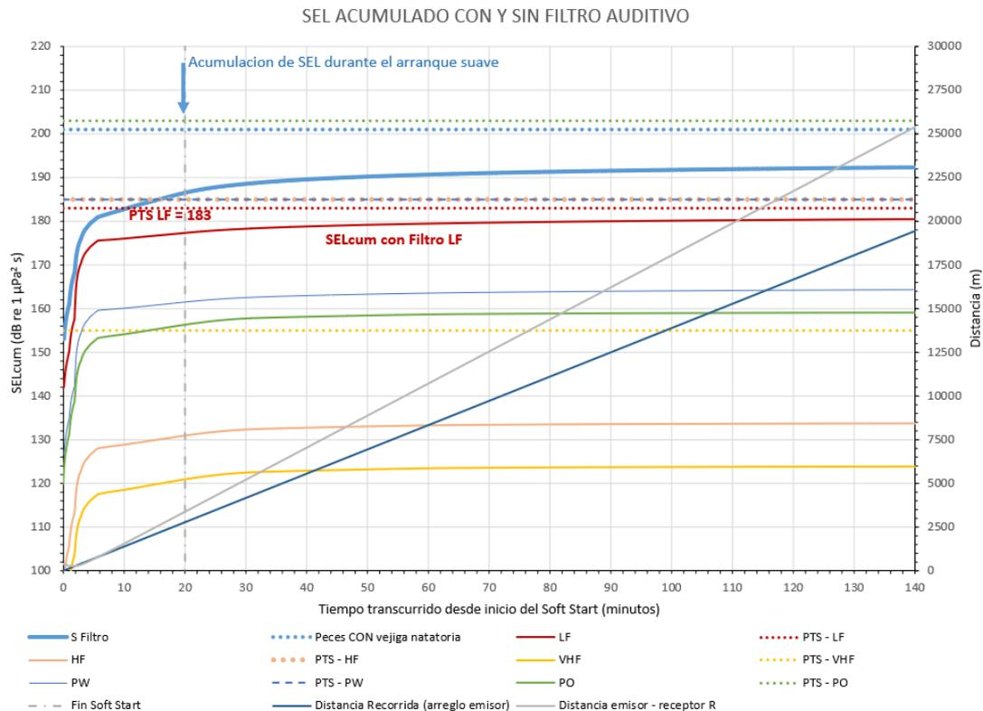
**Figure 32. CAN\_100-108. Accumulated SEL. 20-minute Soft Start. Initial position of the receiver 400 m from the transmitter on the line of advance. 90° at 2 m / s Azimuth movement of the receiver.**
