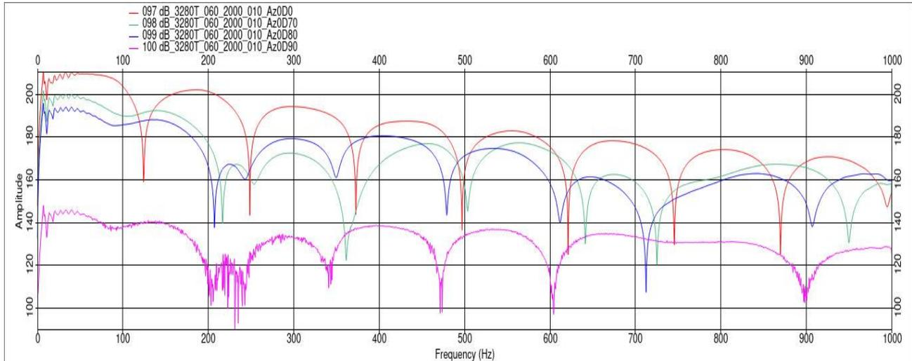
**Figure 10. Energy spectrum for different angles with the vertical and with 90° Azimuth regarding the advance direction for the 3,280 cu.in array.**
