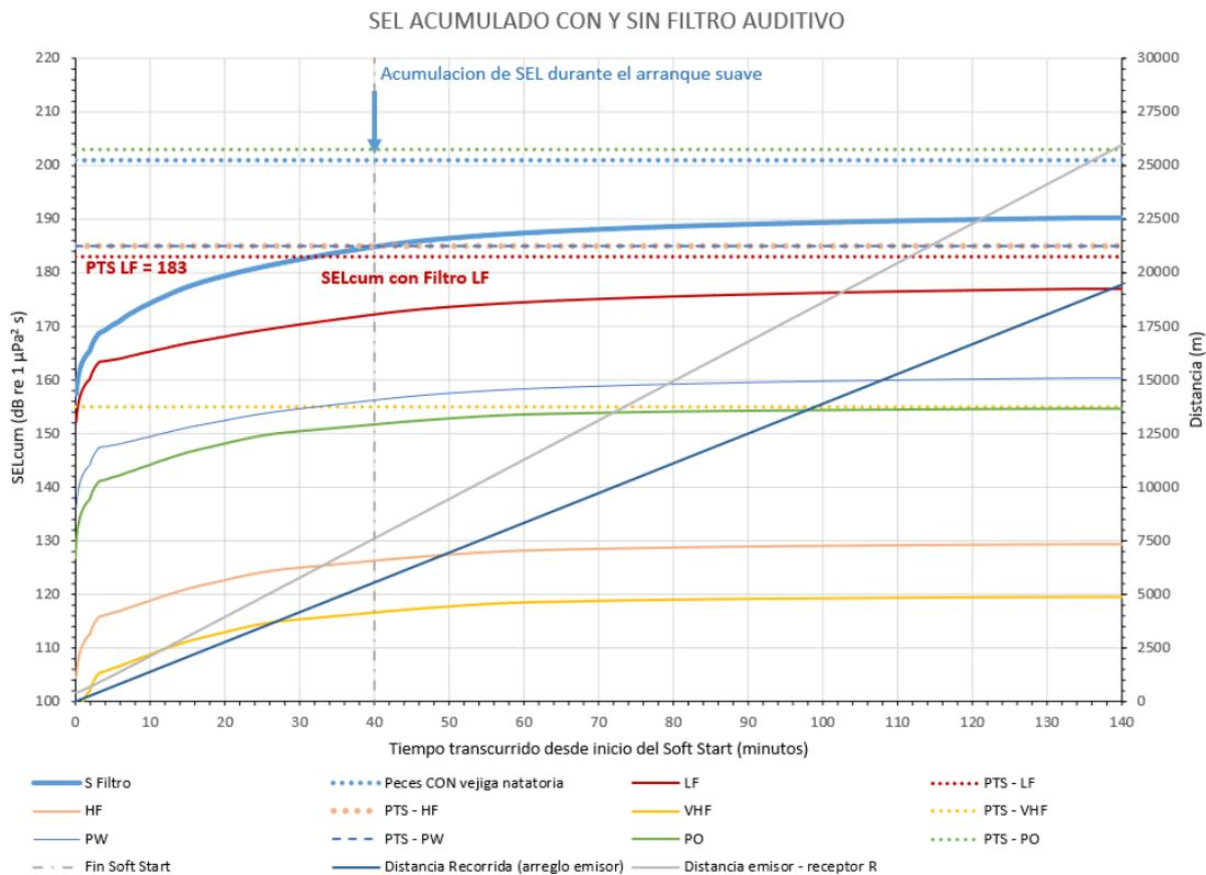
**Figure 36. CAN\_100-108. Accumulated SEL. 40-minute Soft Start 40. Initial position of the receiver 400 m away from the transmitter, perpendicular to the advance line at the Soft Start starting point. 90° at 2 m / s Azimuth movement of the receiver.**
