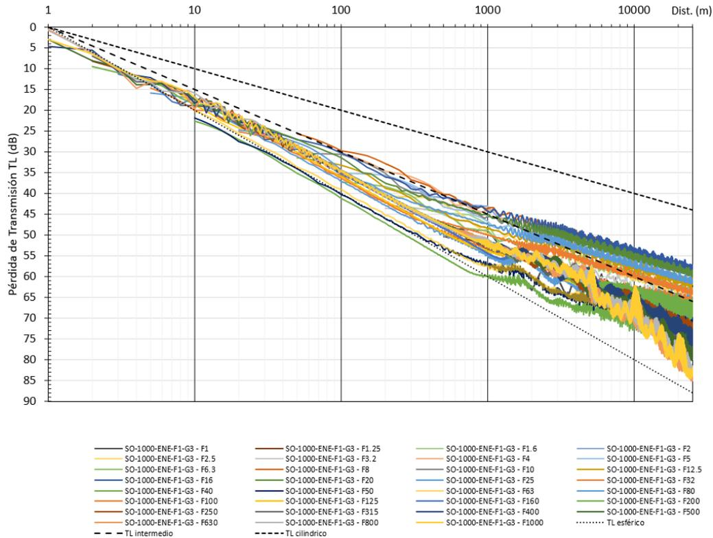
**Figure 18. Minimum Transmission Loss in the vertical and in TLV, H distance for the CAN\_100-108 area, with the most conservative condition of the sensitivity analysis (Sludge F1 and underlying Gravel G3).**
