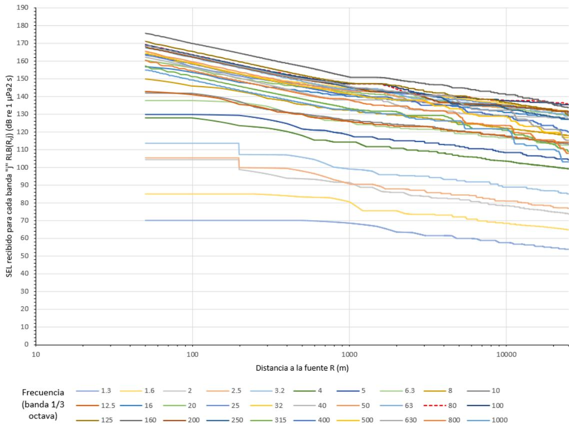
**Figure 23. Received SEL (RL) for each band. CAN\_100-108. 0° Azimuth 70° Dip. LF Filter.**
