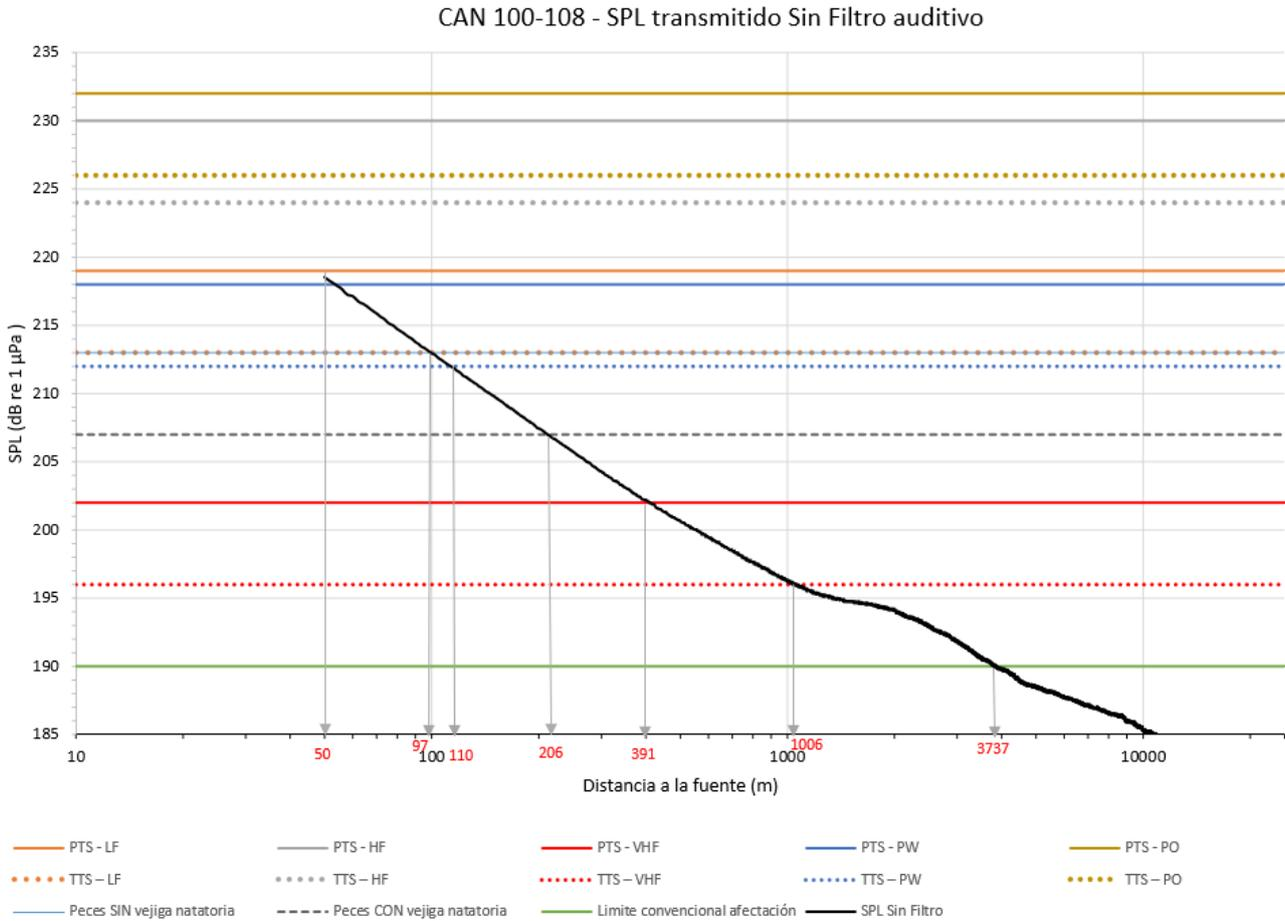
**Figure 30. Example of comparison between the SPLTOTAL values and the different thresholds to determine the corresponding distances (CAN\_100-108. 90° Azimuth - 70° Dip, AB-GB Soils).**
