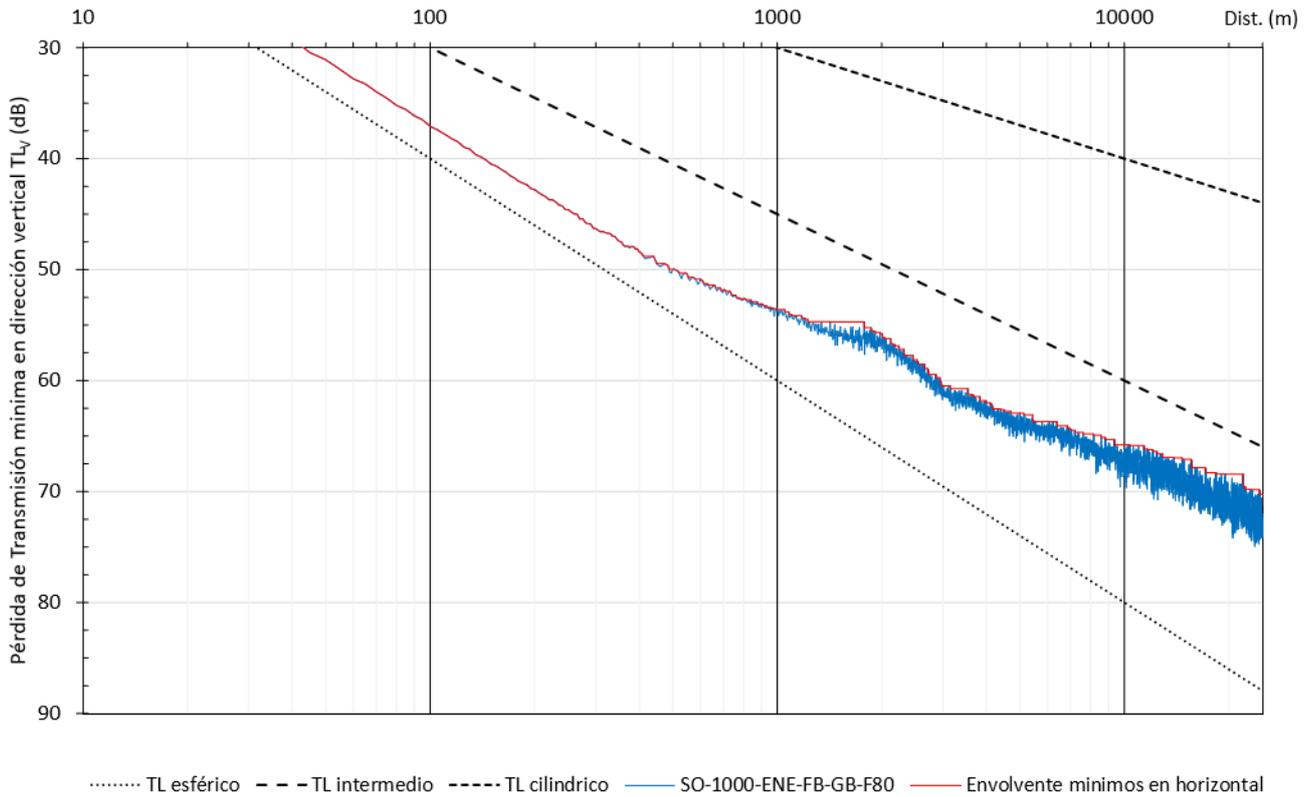
**Figure 16. Example of processing of the two-dimensional TL matrix calculated by the RAM model to obtain the minimum Transmission Loss vertically (oscillating blue line) and the minimum envelope horizontally (red line).**
