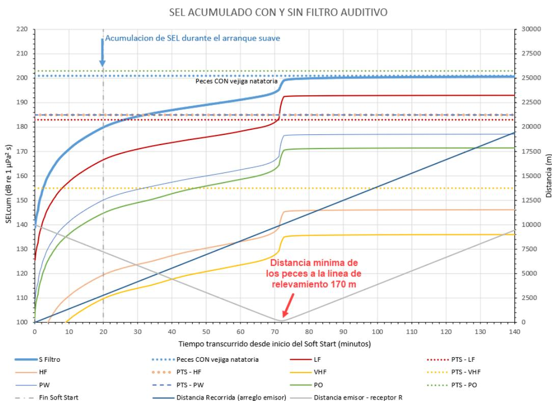
**Figure 37. CAN\_100-108. Cumulative SEL equal to the potential mortality threshold for fish with swim bladder, considering that they are located 170 m from the survey line.**
