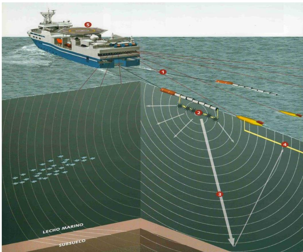
**Figure 2. Display of a 3D seismic survey.**
