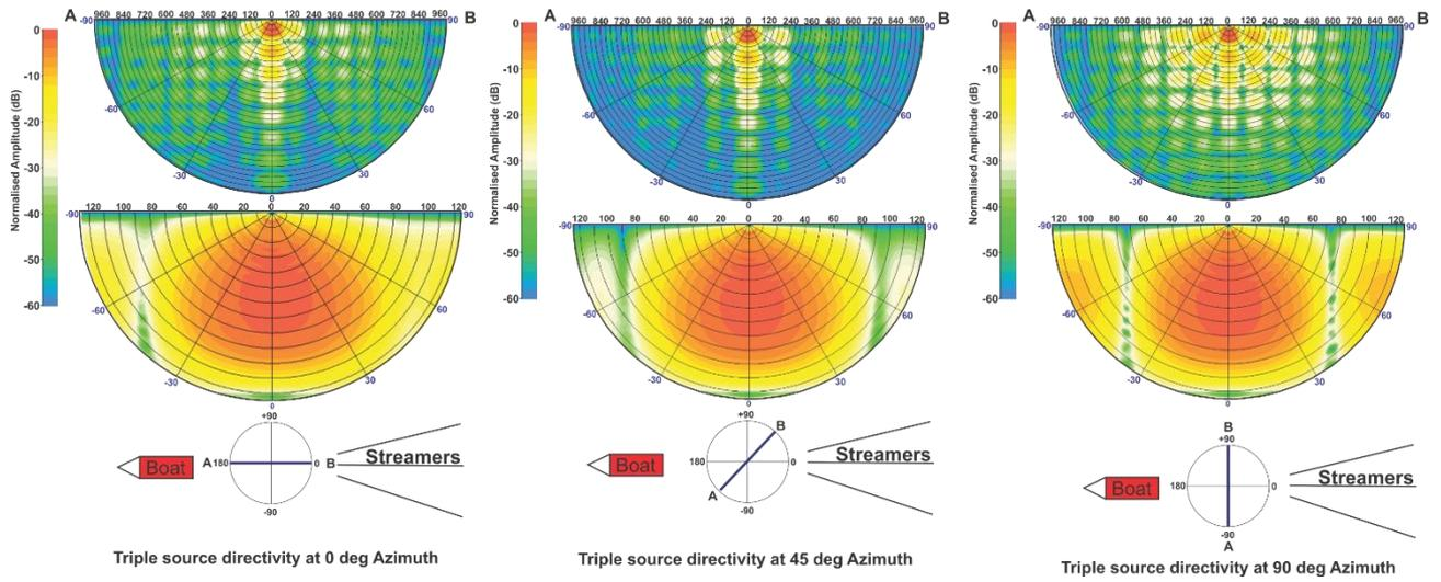
**Figure 8. 2D spectra for different Azimuths as regards the direction of advance of the survey for the Triple array of 3,280 cu.in.**
