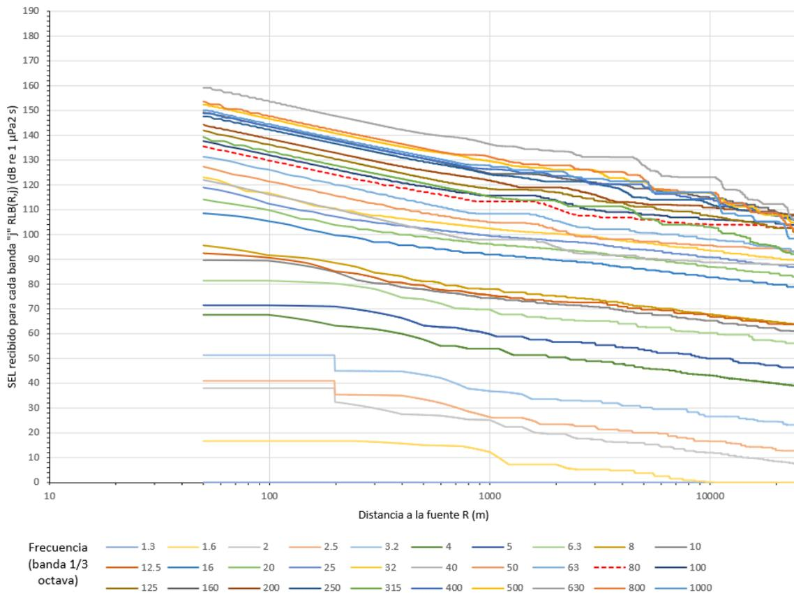
Figure 27. Received SEL (RL) for each band. CAN\_100-108. 0° Azimuth 70° Dip. PO Filter.
