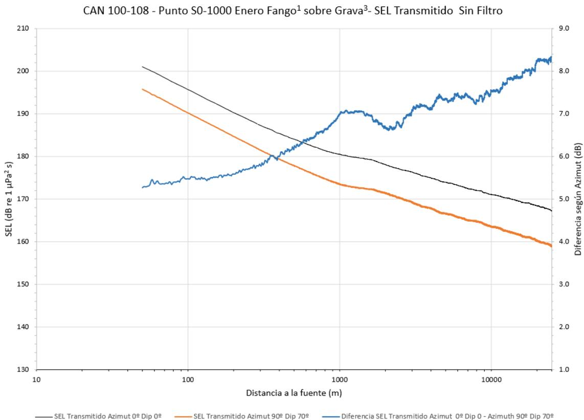
**Figure 28. Received SEL (RL). CAN\_100-108. 0° Azimuth vs 90° no filter.**
