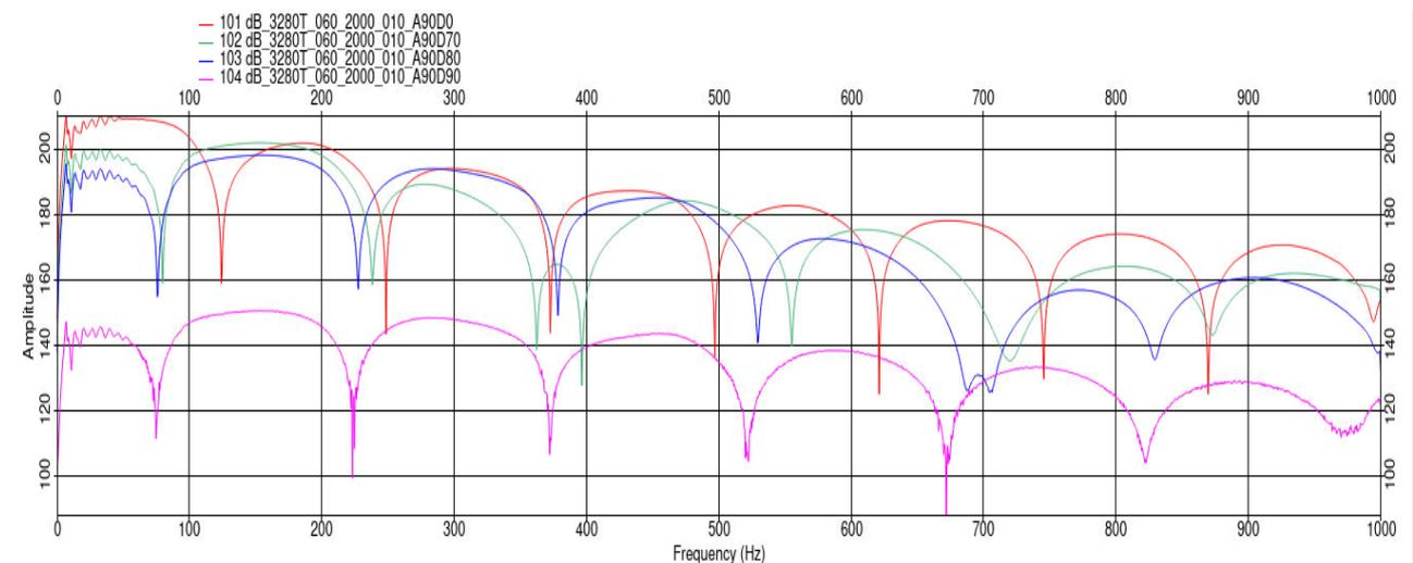
**Figure 11. Energy spectrum for different angles with the vertical and with 90° Azimuth regarding the advance direction for the 3,280 cu.in array.**
