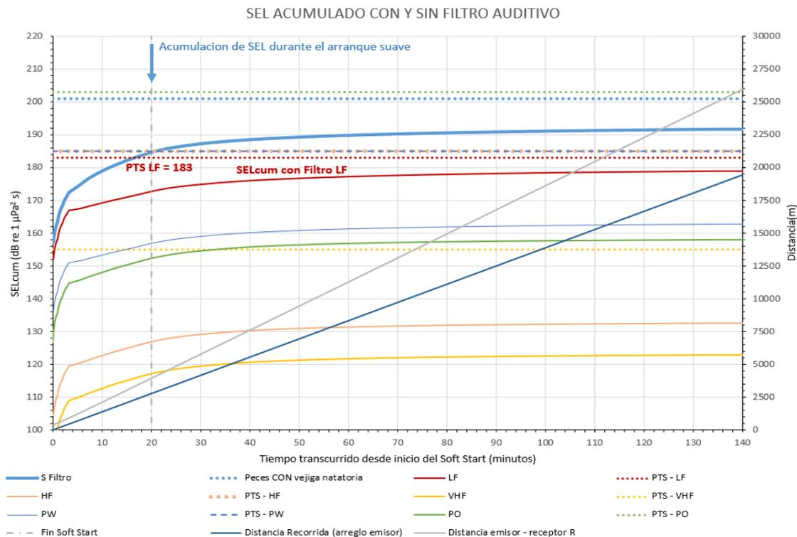
**Figure 39. CAN\_114. Accumulated SEL. 20-minute Soft Start. Initial position of the receiver 400 m away from the emitter, perpendicular to the advance line at the Soft Start starting point. 90° at 2 m / s Azimuth movement of the receiver.**
