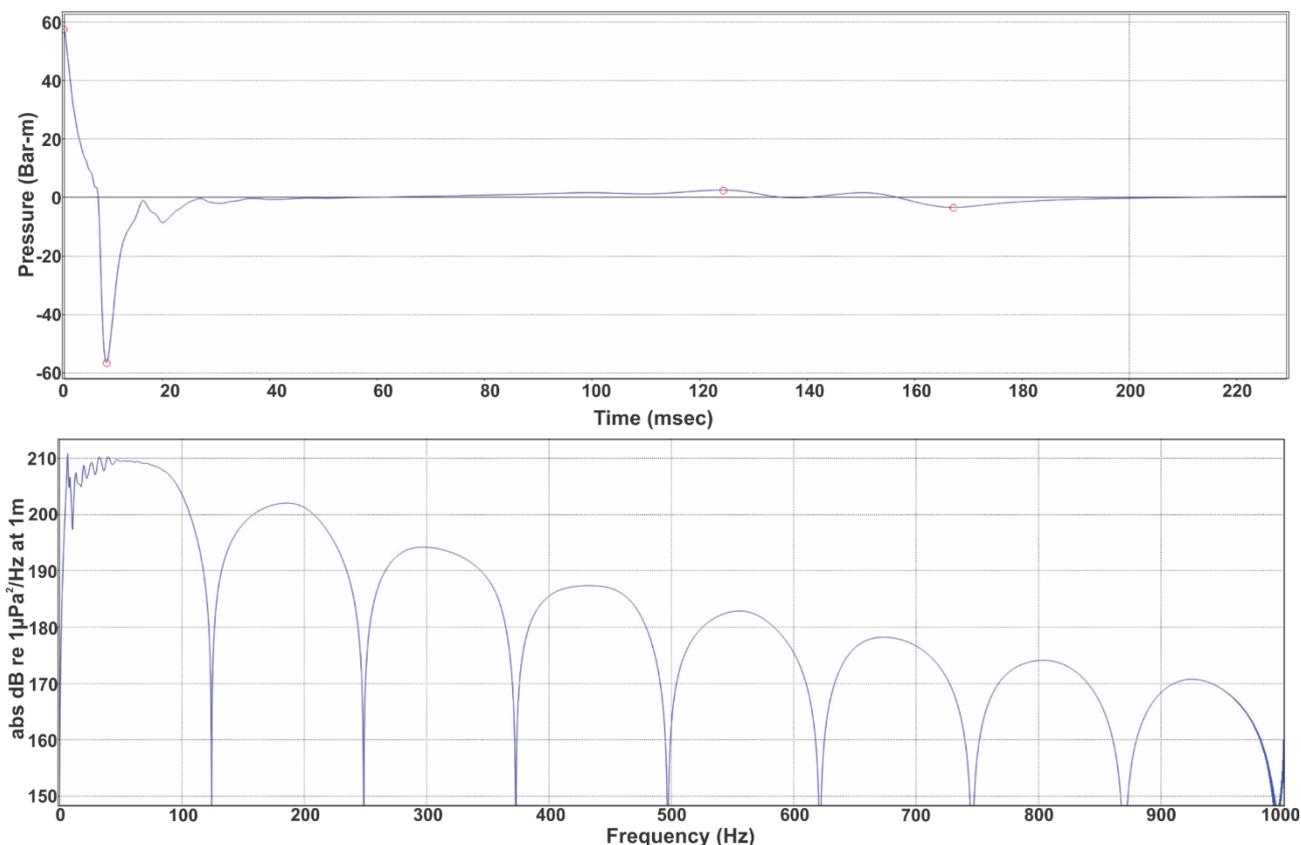
Far Field Signature Time and Amplitude spectra for the Triple Source. Far Field is computed at a distance of 9000m in the inline direction (Azimuth = 0) and directly below the source array (Dip = 0).
