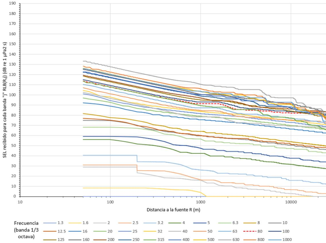
Figure 24. Received SEL (RL) for each band. CAN\_100-108. 0° Azimuth 70° Dip. HF Filter.
