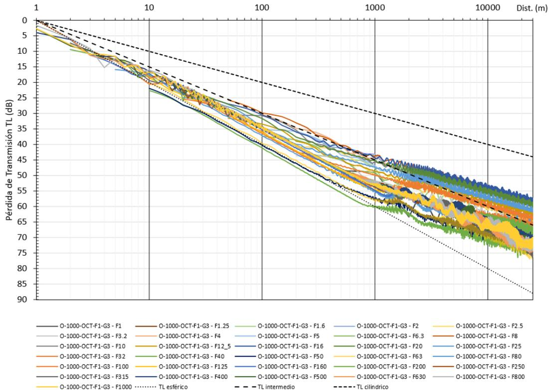
**Figure 20. Minimum Transmission Loss in the vertical and in TLV, H distance for the CAN\_114 Area, with the most conservative condition of the sensitivity analysis (Sludge F1 and underlying Gravel G3).**
