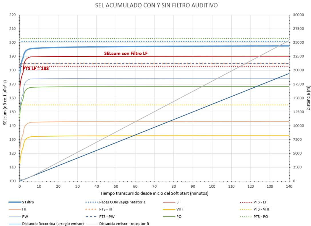
**Figure 34. CAN\_100-108. Accumulated SEL. No Soft Start Hypothesis. Initial position of the receiver 400 m from the transmitter on the line of advance. 90° at 2 m / s Azimuth movement of the receiver.**
