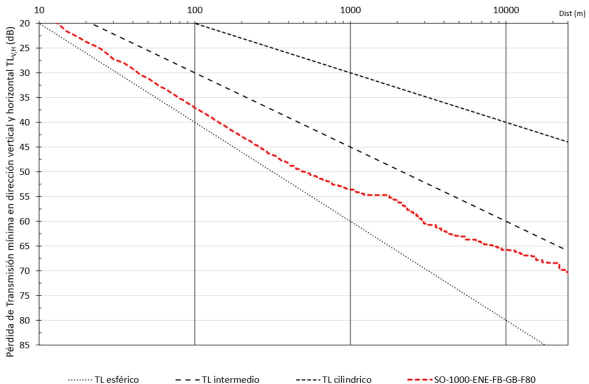
**Figure 17. Example of the final result of the processing of the two-dimensional TL matrix calculated by the RAM model to obtain the minimum Transmission Loss vertically and horizontally.**
