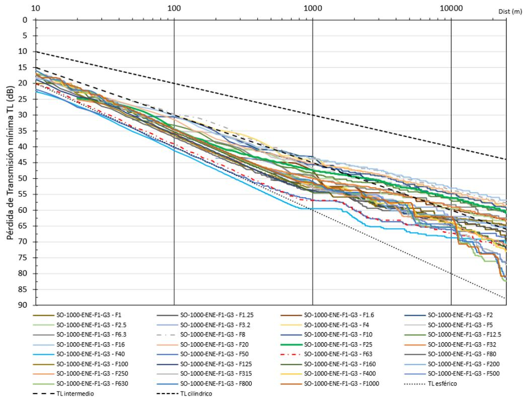
**Figure 19. Minimum Transmission Loss in the TLV vertical for the CAN\_114 Area, with the most conservative condition of the sensitivity analysis (Sludge F1 and underlying Gravel G3).**
