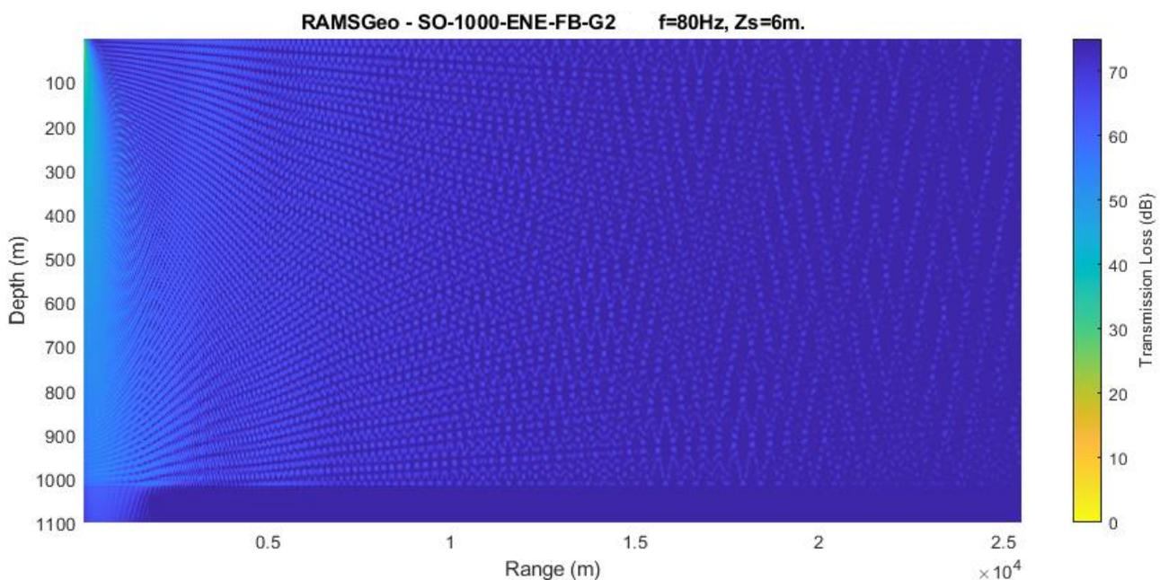
Figure 15. Example of a two-dimensional TL matrix calculated by the RAM model
