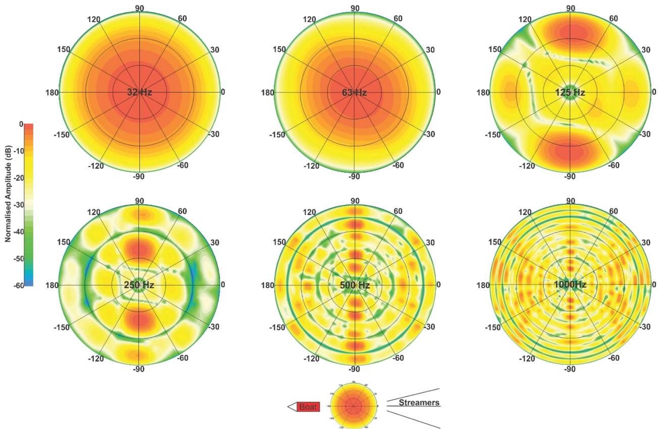
**Figure 9. Polar graphics of angular distribution of sound energy for frequencies in octaves.**
