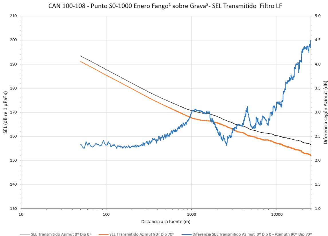
**Figure 29. Received SEL (RL). CAN\_100-108. 0° Azimuth vs 90° LF Filter (low frequency).**
