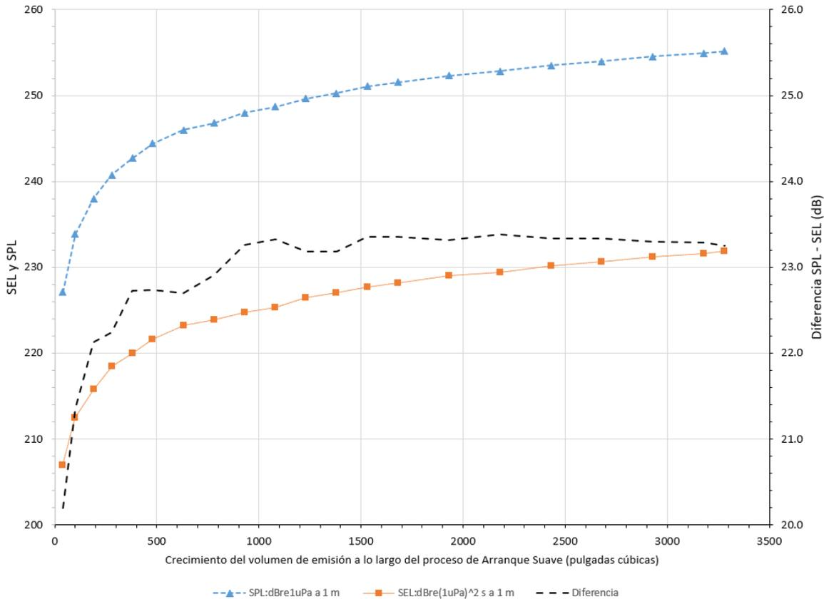
**Figure 14. Evolution of the SPL and SEL<sub>peak</sub> resulting from the increase in the emission volume during the soft start procedure. Note that the units of each variable are different.**
