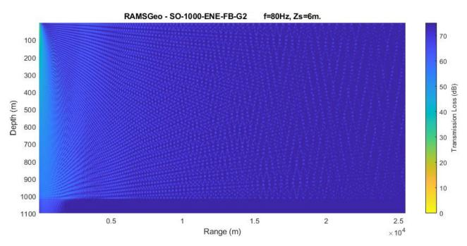
Figure 15. Example of a two-dimensional TL matrix calculated by the RAM model
