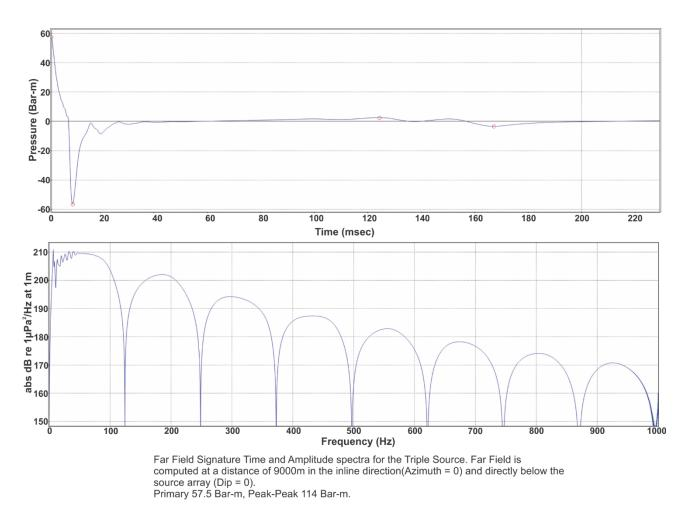
Figure 7. Vertical acoustic signature of the 3,280 cu.in. Triple array spectrum.
