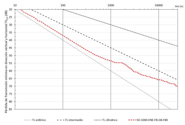
Figure 17. Example of the final result of the processing of the two-dimensional TL matrix calculated by the RAM model to obtain the minimum Transmission Loss vertically and horizontally.
