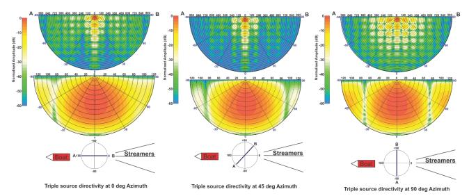
Figure 8. 2D spectra for different Azimuths as regards the direction of advance of the survey for the Triple array of 3,280 cu.in.
