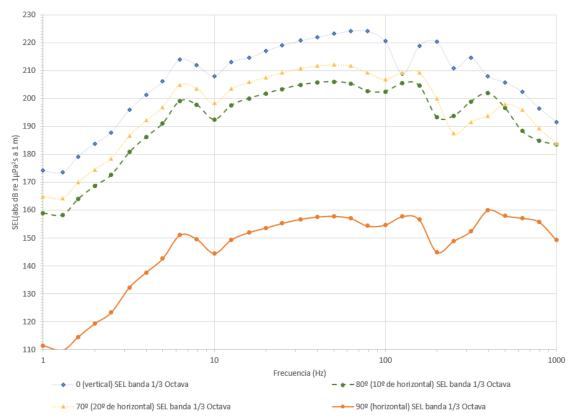
Figure 12. Energy per octave for different angles in 0° Azimuth (forward direction).
