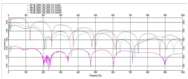
Figure 10. Energy spectrum for different angles with the vertical and with 90° Azimuth regarding the advance direction for the 3,280 cu.in array.
