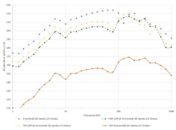
Figure 13. Energy per octave for different angles in 90° Azimuth (perpendicular to the advance).
