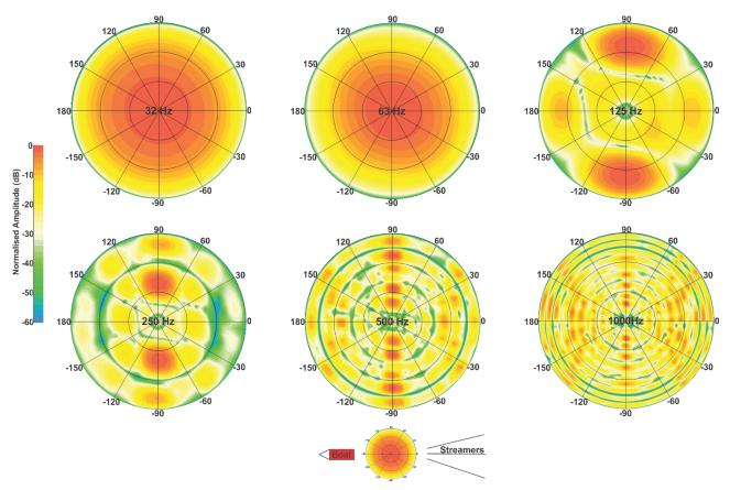
Figure 9. Polar graphics of angular distribution of sound energy for frequencies in octaves.
