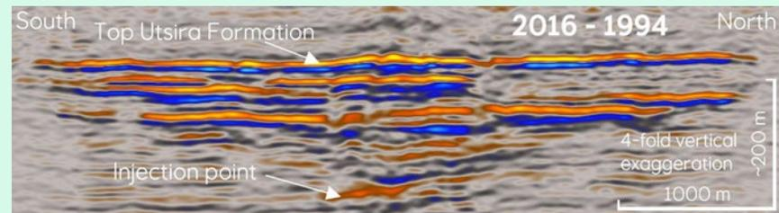
Seismic section through the Sleipner CO<sub>2</sub> reservoir: seismic time-lapse data (amplitude difference) of the 2016 and 1994 campaigns. The intense colours (especially yellow, blue) show the presence of CO<sub>2</sub> accumulating beneath thin clay layers and under the tight caprock seal.
