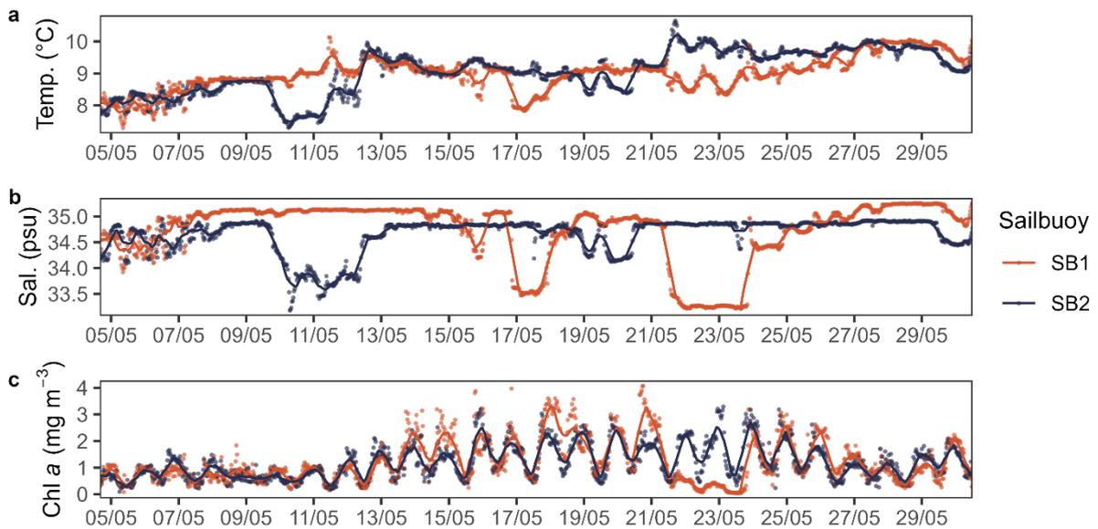
Figure 7 Surface (a) temperature, (b) salinity, and (c) chlorophyll *a* from SB Echo 1 (red line) and Echo 2 (blue line) during the Hywind Tampen survey. The dots show the raw data, and the lines represent the rolling mean (rolling window of 20 samples).
