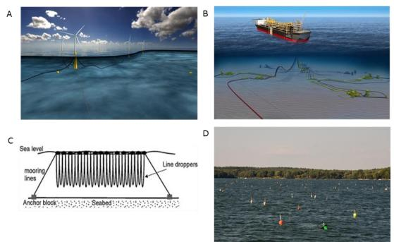
**Figure 4:** Structures with comparative layouts to floating wind turbines. a) typical floating turbine layout. *Source*: Equinor (2015); b) FPSO facility. *Source*: MODEC; c) longline mussel farms. *Source*: Stevens *et al.* (2008); and d) high density of lobster pots. *Source*: <u>SeaGoingGreen</u>, photographer: Andrew Malone.
