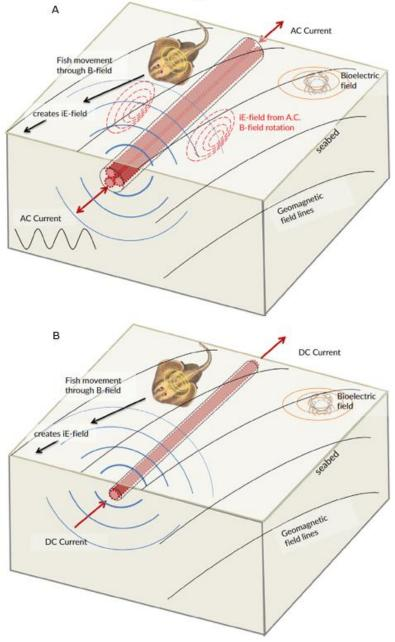
**Figure 5:** EMF s associated with a) AC and b) DC power cables .GMF in black, bioelectric fields in orange, B-fields in blue, iE-fields induced in fish yellow, and iE-field in surrounding conductive seawater in red. *Source*: Newton *et al.* (2019).
