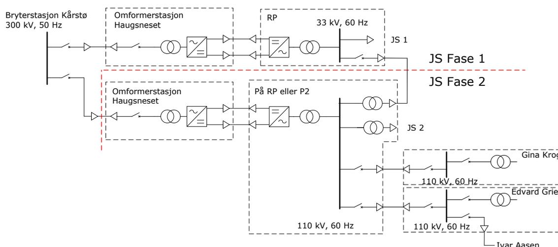
**Figure 4-1 Phased Expansion of Johan Sverdrup Power Solution to Cover Utsira High Area**
