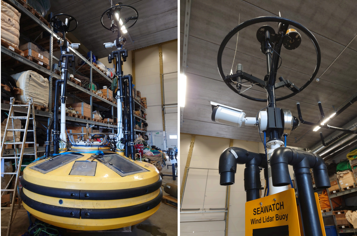
Figure 6: The Fugro SEAWATCH buoy in the workshop prior to deployment. The bird monitoring cameras are installed at the two poles. Pictures taken March 2023 by Felix Kelberlau, Fugro.
