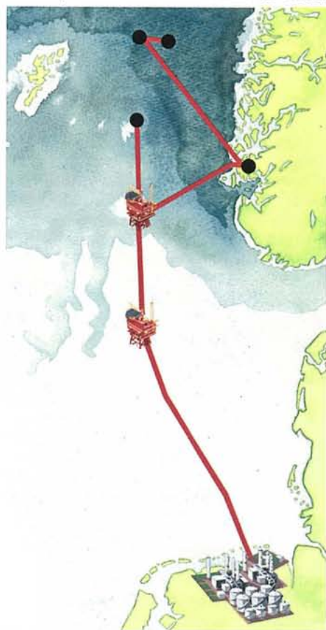
The Statpipe gas gathering system will tie Statfjord and Gullfaks directly to the Continental buyers via the Norpipe system from Ekofisk to Emden.
