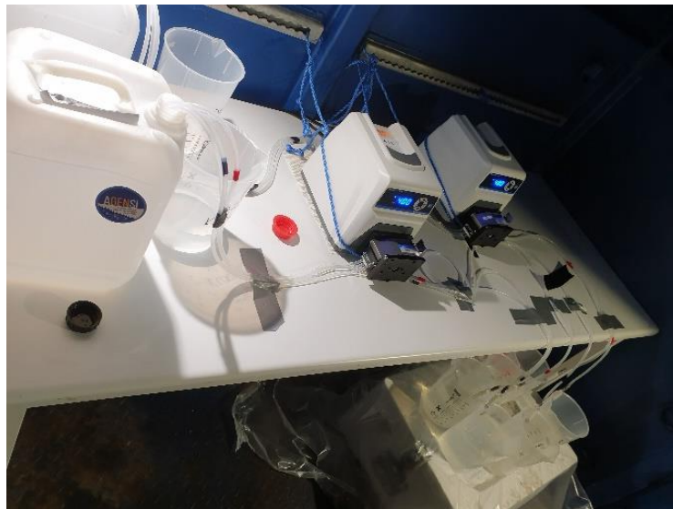
Figure 3. Simultaneous filtration of collected water samples inside the on-deck container using peristaltic pumps powered from electricity to the container. Triplicate 2L-water samples (brown bottles) from each sampling depth were filtered through 0.45 µm Sterivex filters using four-channel pump heads and subsequently frozen. Filter outflow was collected in 2L-beakers, and outflow volume was measured and recorded.
