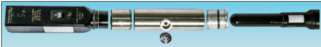
Figure 7. GRAS 42 AC Pistonphone, sleeve coupler and hydrophone
