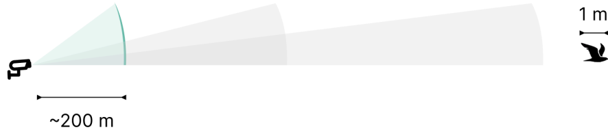
Figure 49: The estimated detection range for a bird with wingspan of 1 m is ~200 m for viewpoint C. The flight height distribution in Figure 48 covers this range.
