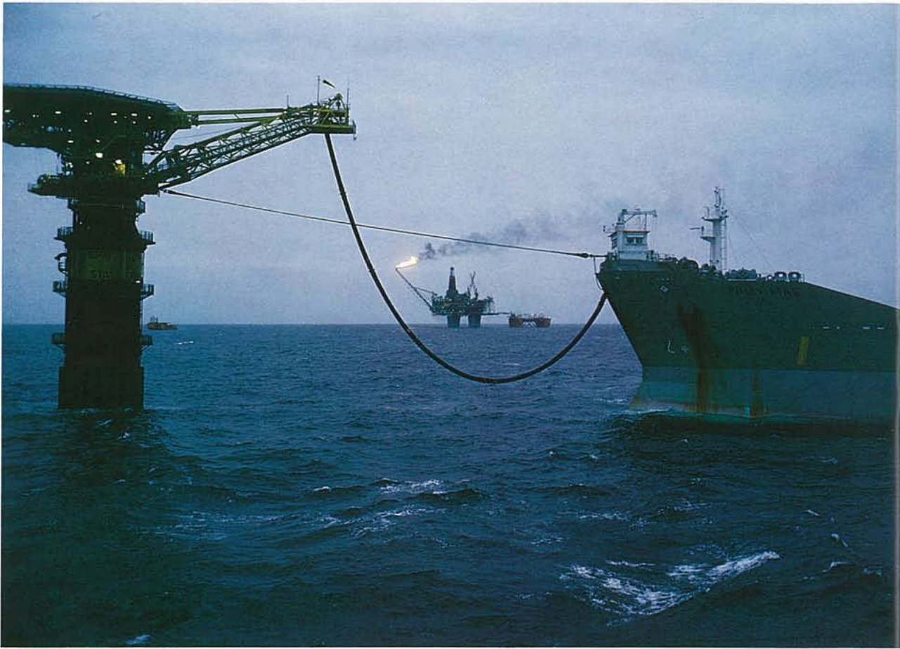
Top: Buoy loading at the Statfjord field. M/T Polyviking receives crude oil from the Statfjord B-buoy. Bottom: Polyviking has arrived at Rotterdam and has started unloading. In the harbour we see the crane barges Balder and Hermod , both of which made many heavy lifts when Statfjord was developed.
