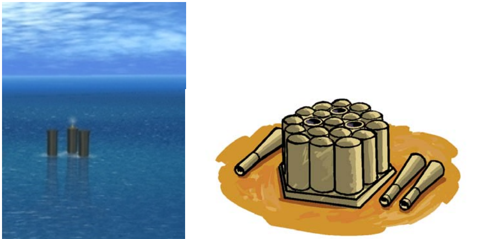
Figure 5. Illustrations of options for leaving the concrete substructure in situ, entirely with navigation lights (left) and cut down to the storage cells. Examples from Frigg cessation plan where the illustration to the left represents the approved solution for Frigg. Source: Total E&P Norge AS.
