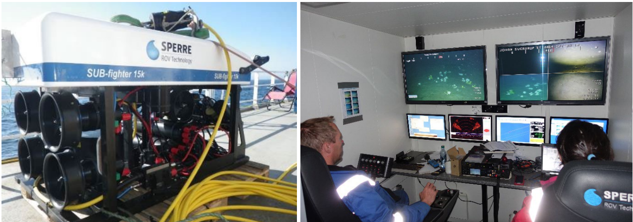
Figure 3-4 ROV type and ROV container (control room) utilized during Hywind Scotland visual mapping survey. Note that the pictures are not from the Hywind Scotland survey but shown for illustration purposes.
