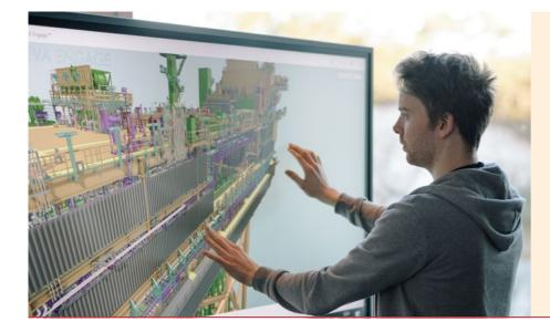
An Equinor operator uses a computer generated 3D model (a digital twin) of the Equinoroperated Valemon platform in Norway to plan offshore work. This technology will allow Rosebank operations teams to pre-plan work onshore, reducing the amounts of physical trips to the platform; reducing safety exposure and lowering emissions.
