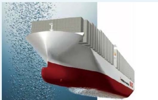
Unorthodox ways of reducing fuel consumption of ships: supplying air to the ship's underside to create a layer of tiny bubbles to reduce friction
